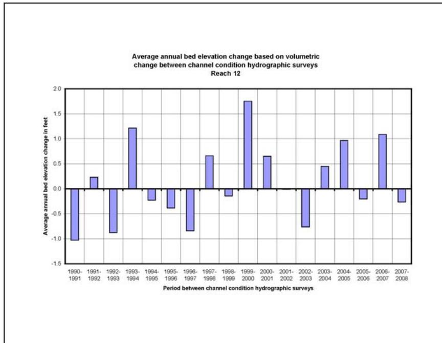
Figure 3.50. Annual average channel bed displacement between channel condition survey periods for Reach 12
