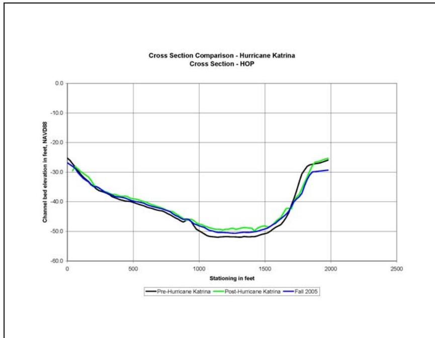
Figure 3.32. Cross section comparison for Hurricane Katrina for cross section located at Head of Passes.
