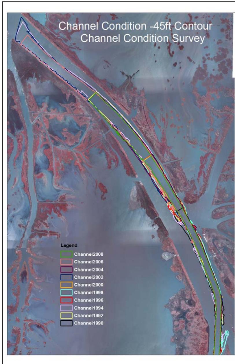
Figure 3.60. Channel location tracings of the -45 foot contour based on the channel condition surveys from Venice to Head of Passes.
