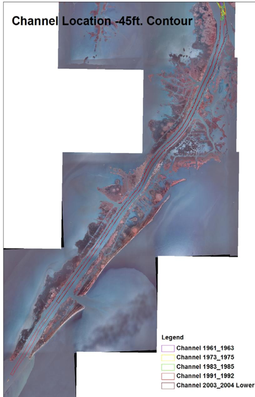
Figure 3.59. Channel location tracings of the -45 ft contour based on the comprehensive surveys from Head of Passes to East Jetty.
