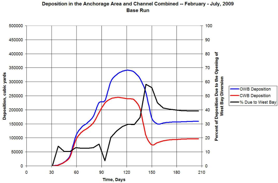
Figure 5.34. Deposition quantities for the combined anchorage area and adjacent channel, base run.
