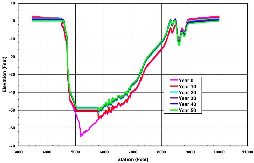
Figure 4.17. Channel Cross Section At River Mile 3.83 In 10 Year Intervals. West Bay Diversion Open, No Dredging Allowed in PAA
