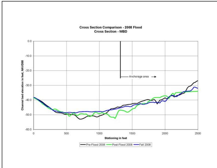
Figure 3.27. Cross section comparison for 2008 flood for cross section located at West Bay diversion.
