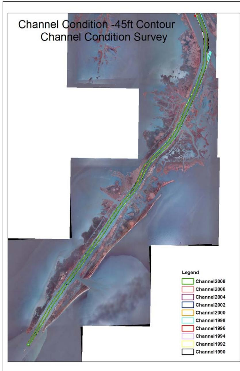
Figure 3.61 Channel location tracings of the -45 foot contour based on the channel condition surveys from Head of Passes to East Jetty
