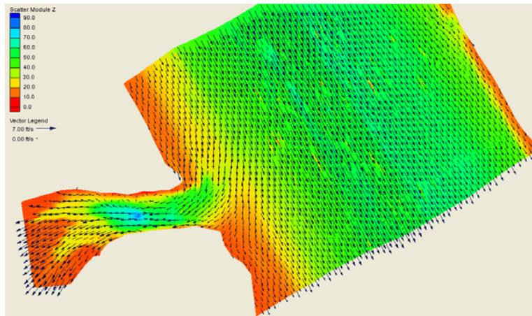
Figure 5.10. Observed bottom velocities at West Bay Diversion on April 22-23.
