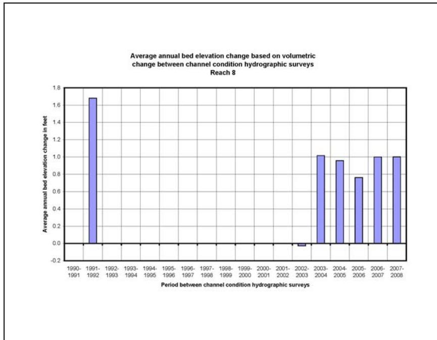
Figure 3.48. Annual average channel bed displacement between channel condition survey periods for Reach 8
