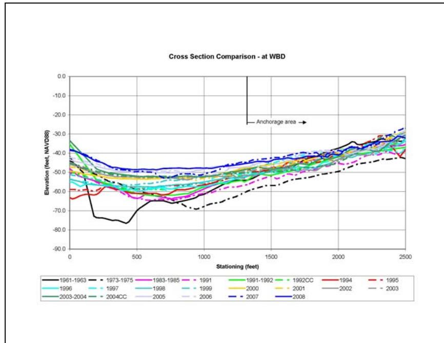
Figure 3.11. Cross section comparison for section located at West Bay Diversion.
