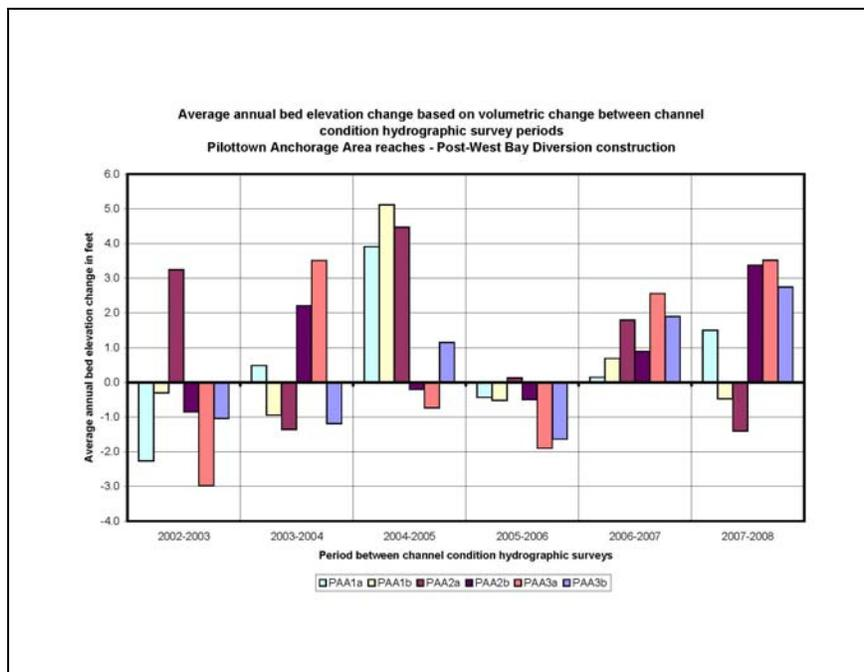
Figure 3.54. Average channel bed displacement based on post-construction channel condition surveys for Pilottown anchorage area reaches.
