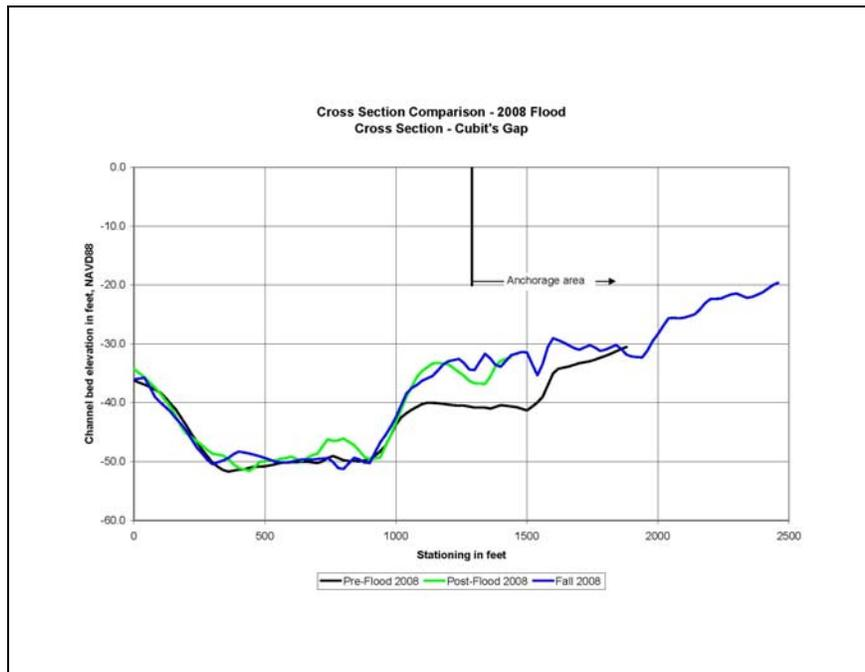
Figure 3.28. Cross section comparison for 2008 flood for cross section located at Cubits Gap.
