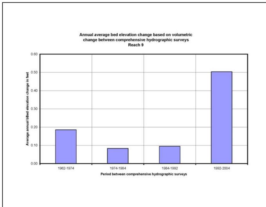
Figure 3.47. Annual average channel bed displacement between comprehensive survey periods for Reach 9.
