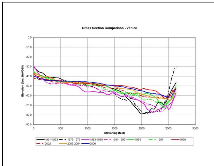
Figure 3.9. Cross section comparison at Venice, just downstream of Grand Pass.
