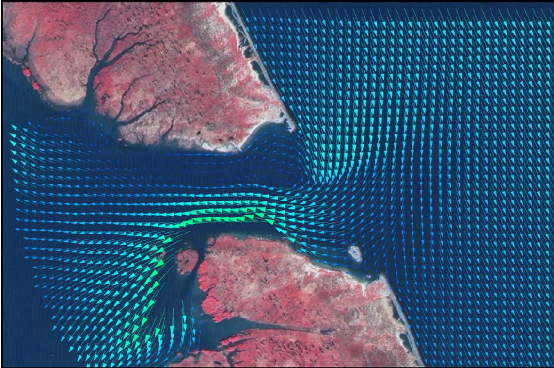
Figure 5.38. Bottom Velocity Vectors.
