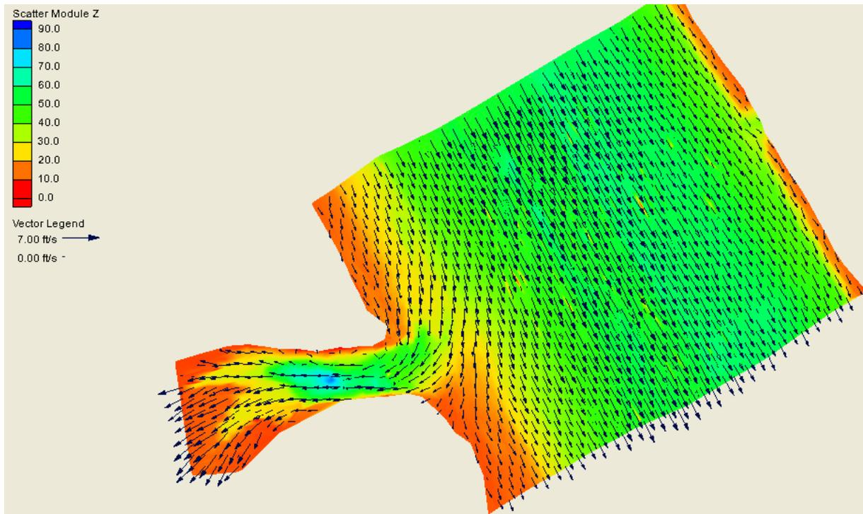
Figure 2.34. Bottom Velocities of the 3D flow measurements during April 23, 2009 trip.
