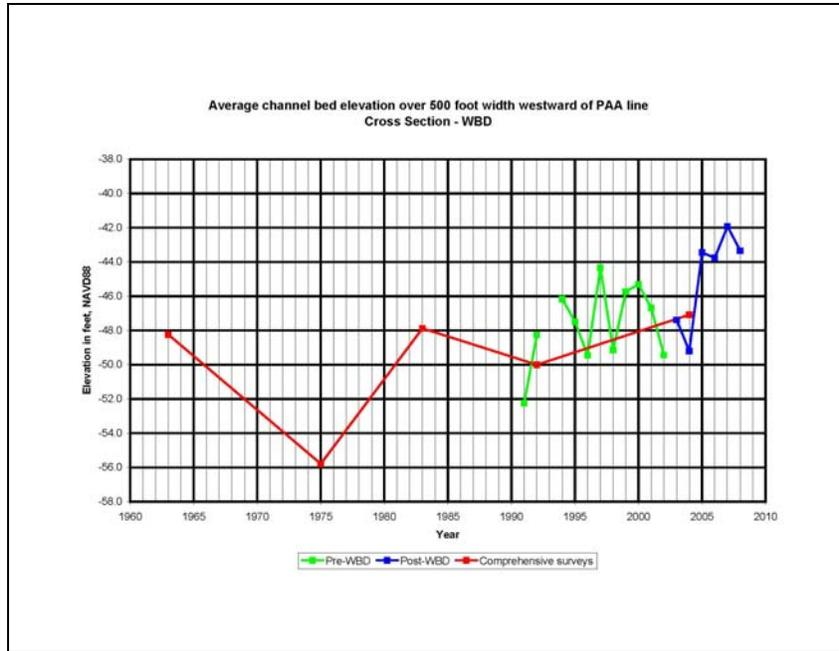
Figure 3.19. Comparison of average channel bed elevation for cross section located at West Bay diversion.
