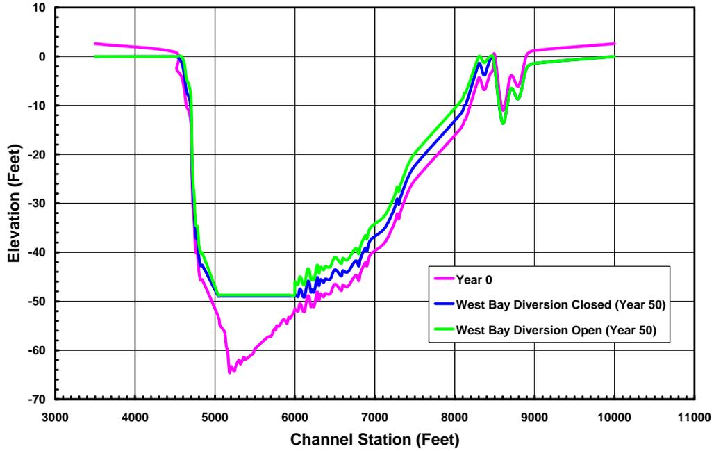
Figure 4.13. Channel Cross Section At River Mile 3.83 At Beginning and End of 50 Year Simulation. Dredging In Pilottown Anchorage Area
