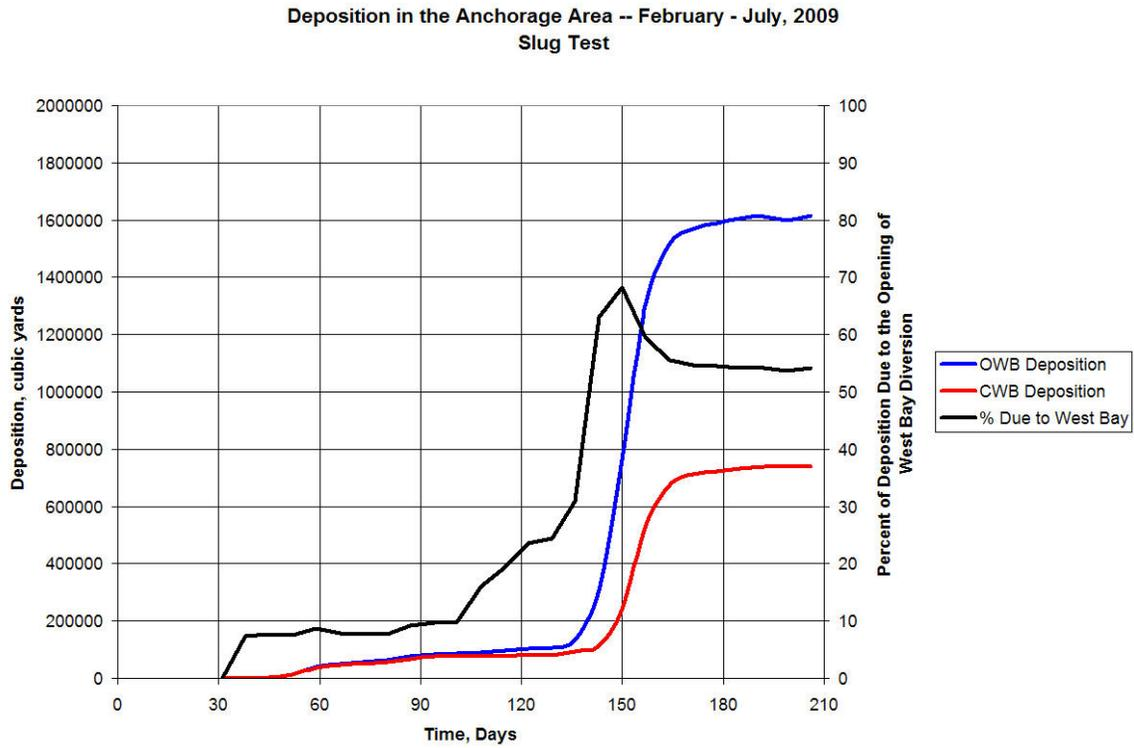
Figure 5.32. Deposition quantities for the anchorage area, slug test.
