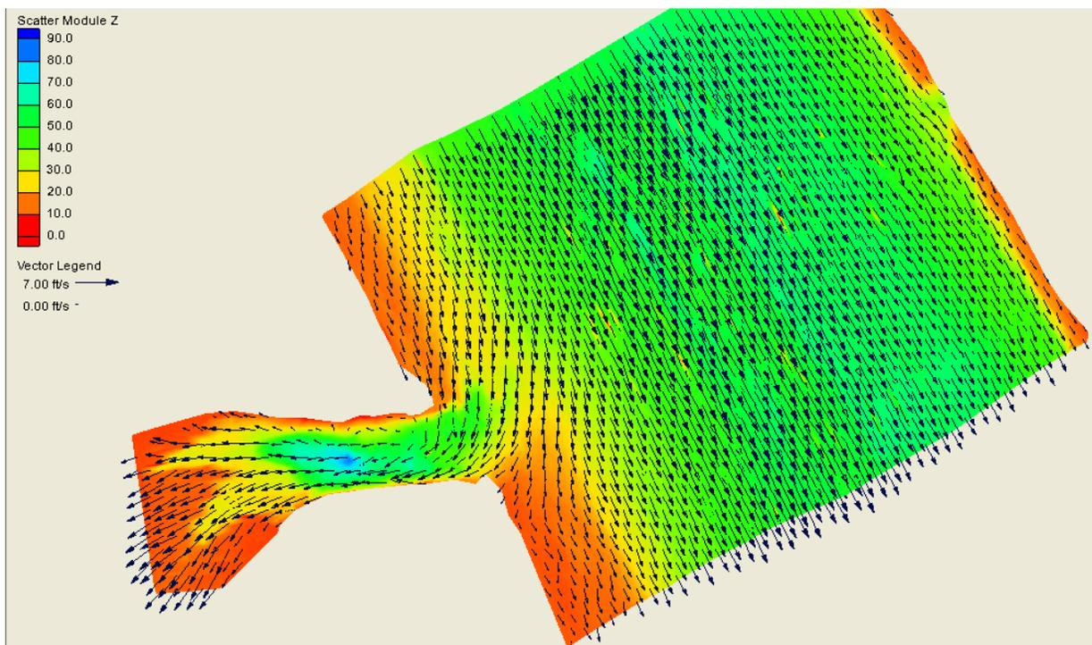
Figure 2.33. Surface Velocities of the 3D flow measurements during April 23, 2009 trip.
