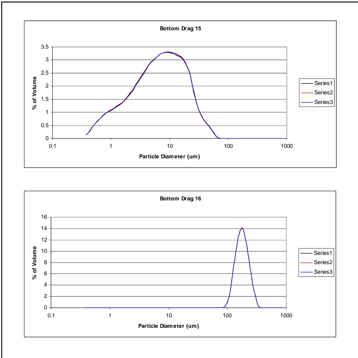
Figure 2.29. Grain size distributions for bottom drag samples 15 and 16.
