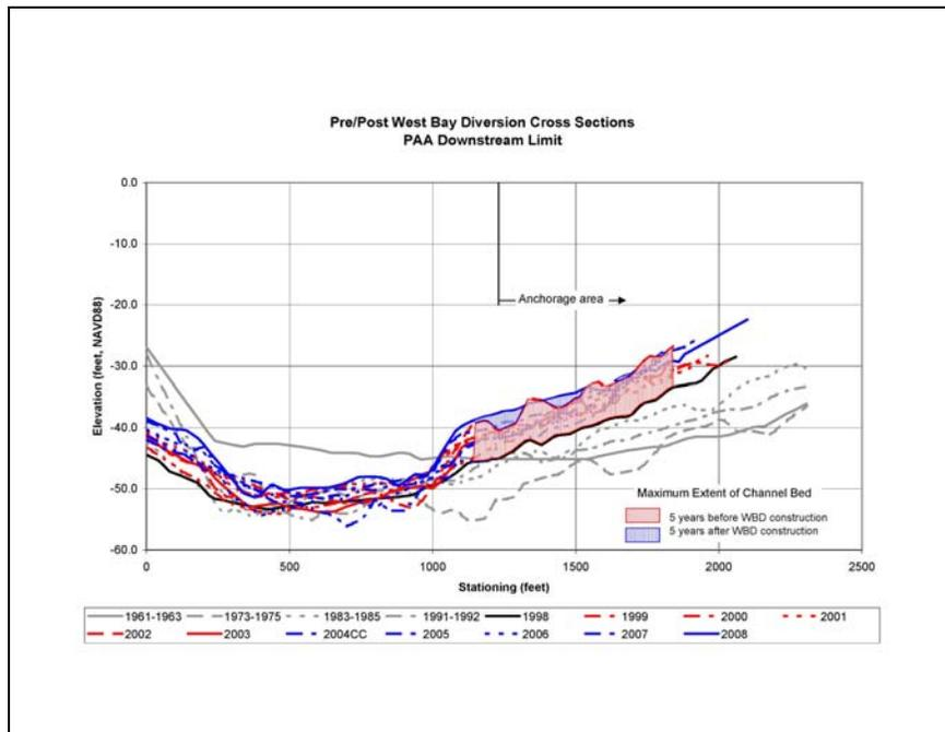
Figure 3.40. Maximum extent of channel bed elevation before and after West Bay diversion construction at downstream limit of anchorage area.
