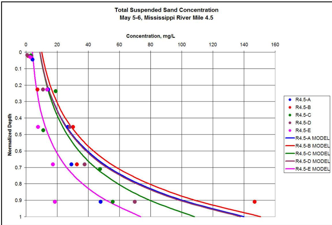
Figure 5.15. Suspended sediment verification for May 5-6.
