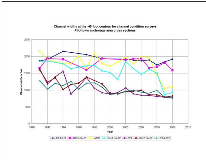
Figure 3.63. Channel widths at the -45 foot contour based on channel condition surveys for cross sections located in the Pilottown anchorage area.
