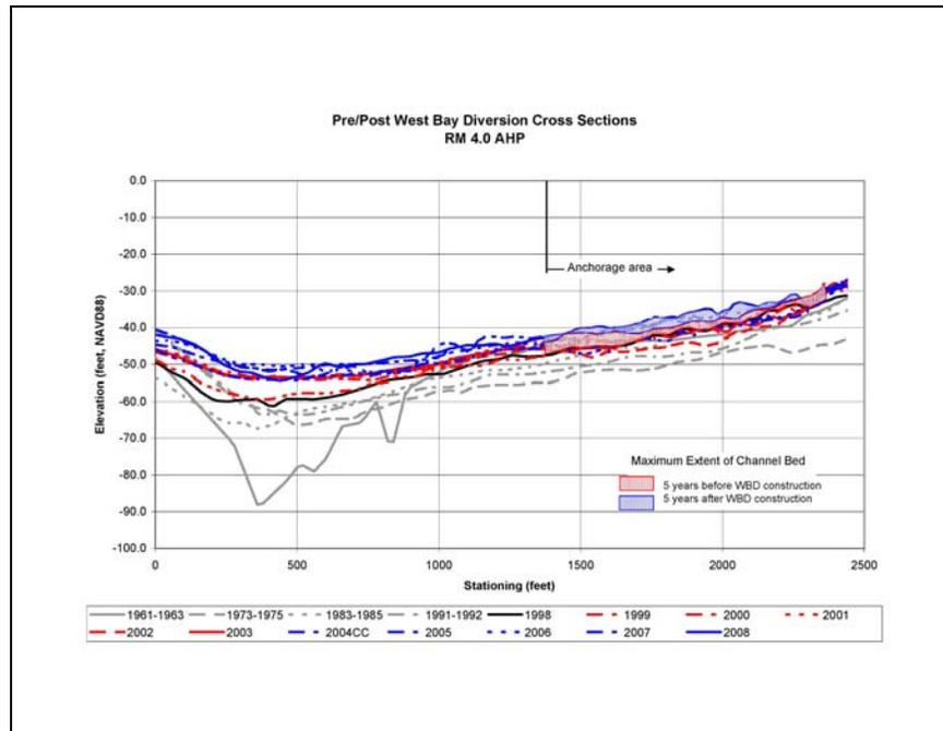
Figure 3.37. Maximum extent of channel bed elevation before and after West Bay diversion construction at RM 4.0 AHP.
