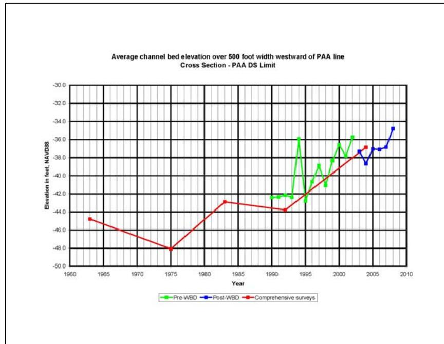
Figure 3.23 .Comparison of average channel bed elevation for cross section located at the downstream limit of the Pilottown anchorage area.
