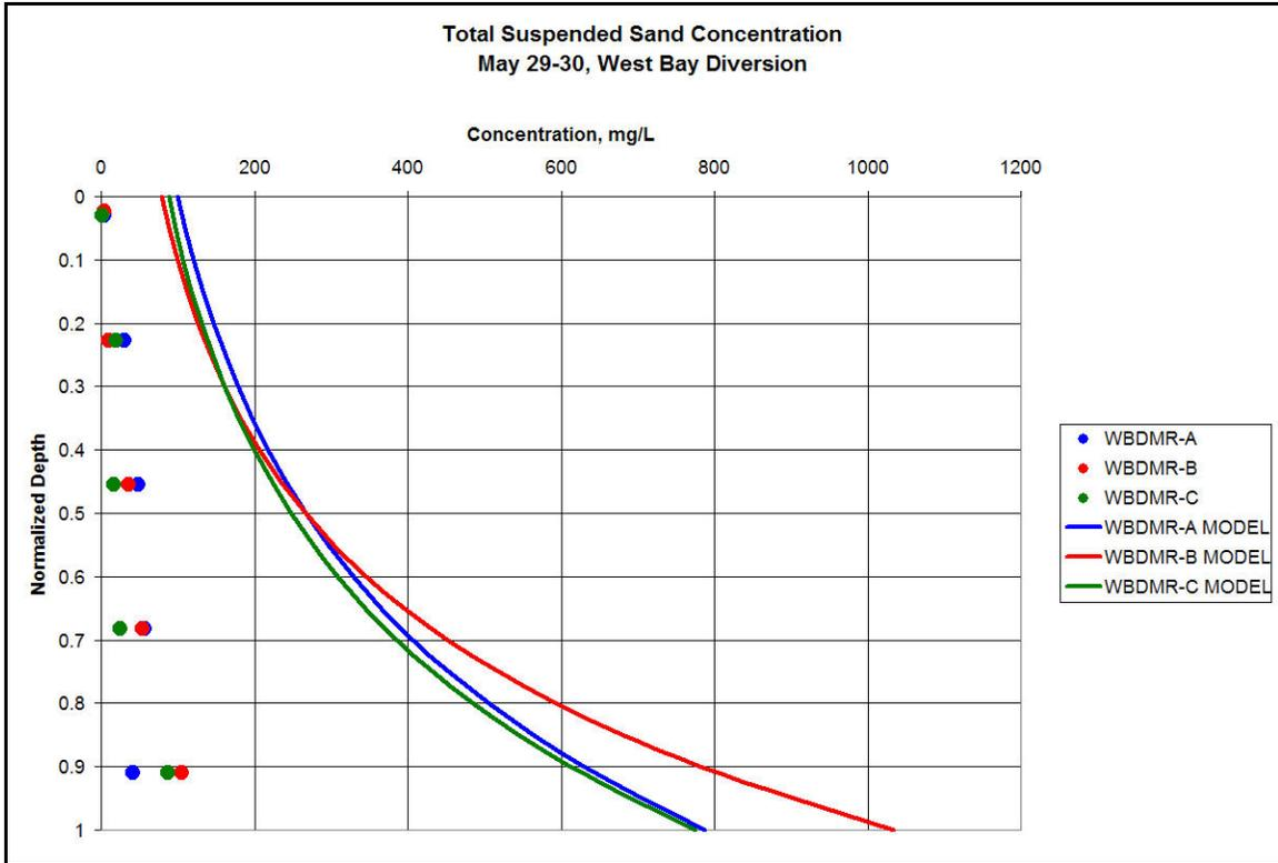
Figure 5.17. Suspended sediment verification at WBD for May 29-30.
