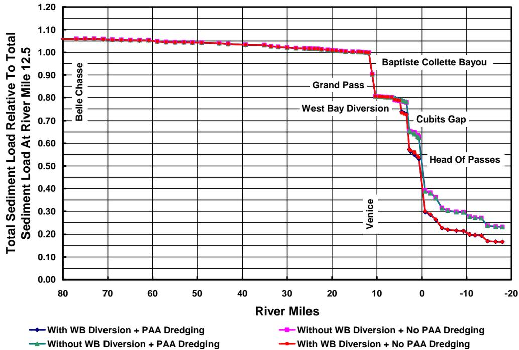
Figure 4.12. Total Sediment Load For The Mississippi River Between RM 80 and RM -20 Relative to Total Sediment Load at River Mile 12.5
