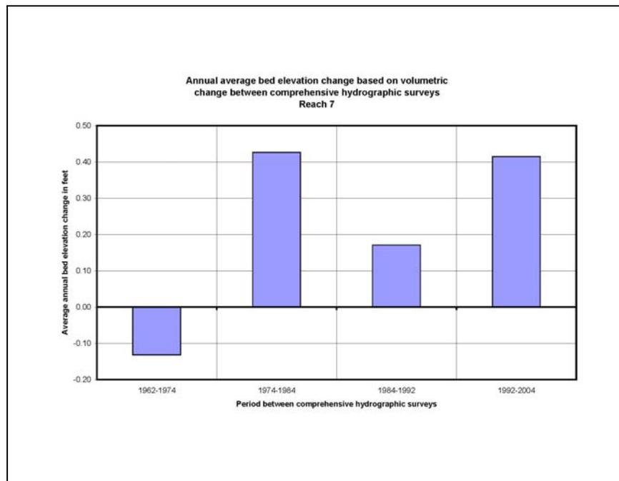
Figure 3.45. Annual average channel bed displacement between comprehensive survey periods for Reach 7.
