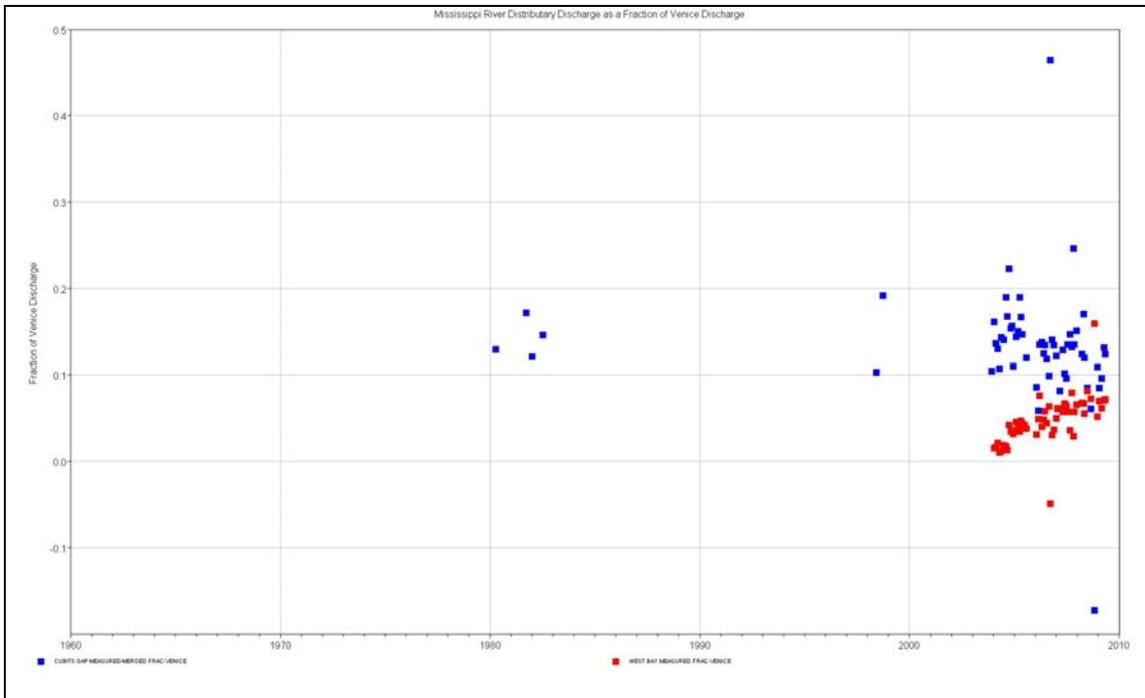
Figure 3.66. Discharge at Cubits Gap and West Bay diversion as a fraction of Venice discharge.
