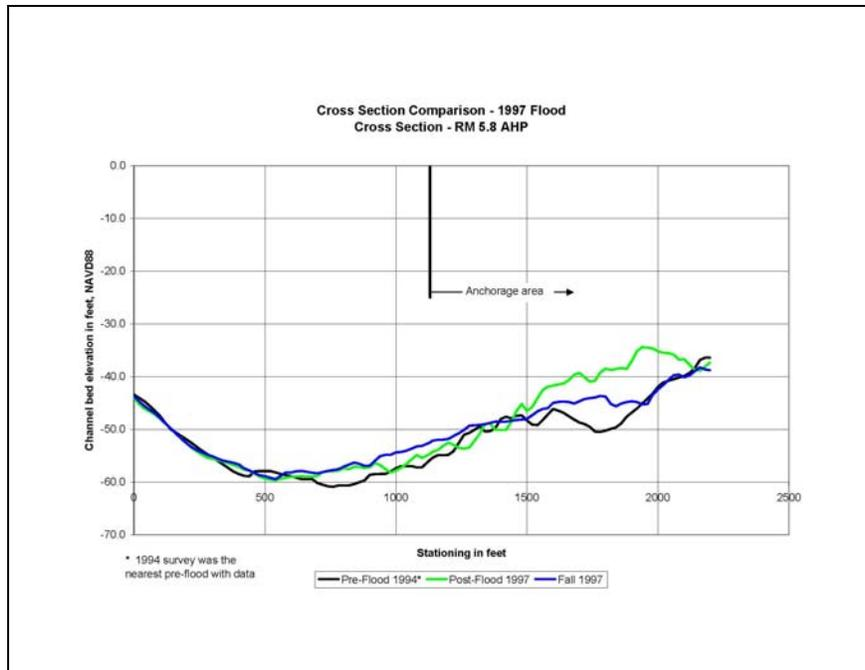
Figure 3.24. Cross section comparisons for 1997 flood for cross section located at RM 5.8 AHP.
