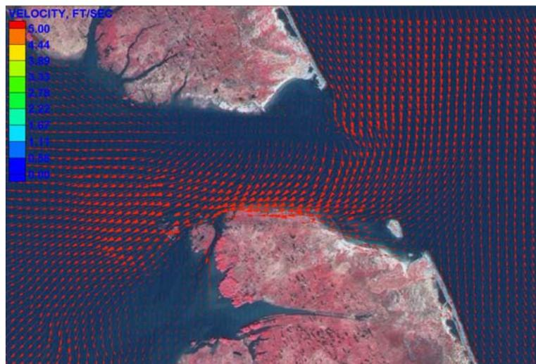
Figure 5.9. Computed surface velocities at West Bay Diversion on April 22-23.
