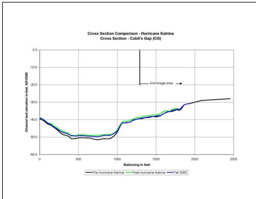
Figure 3.31. Cross section comparison for Hurricane Katrina for cross section located at Cubits Gap.
