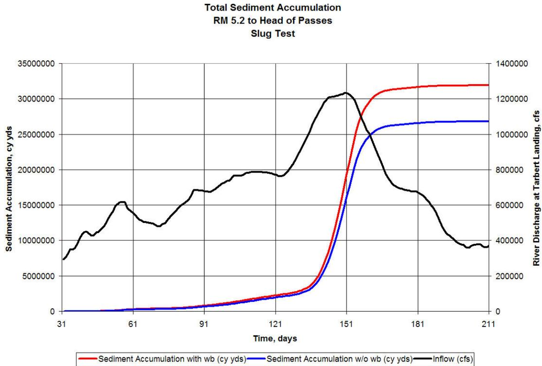
Figure 5.39. Net deposition within between RM 5.2 and Head of Passes, slug test.
