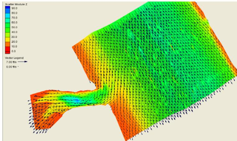
Figure 5.8. Observed surface velocities at West Bay Diversion on April 22-23.
