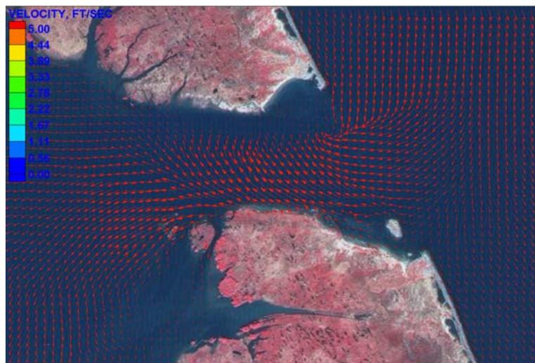
Figure 5.11. Computed bottom velocities at West Bay Diversion on April 22-23.
