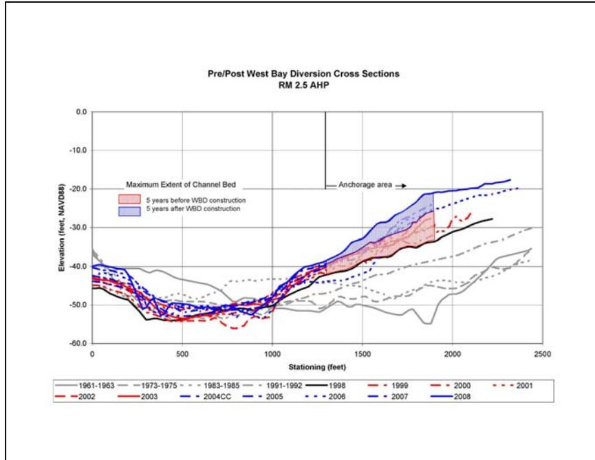
Figure 3.39. Maximum extent of channel bed elevation before and after West Bay diversion construction at RM 2.5 AHP.
