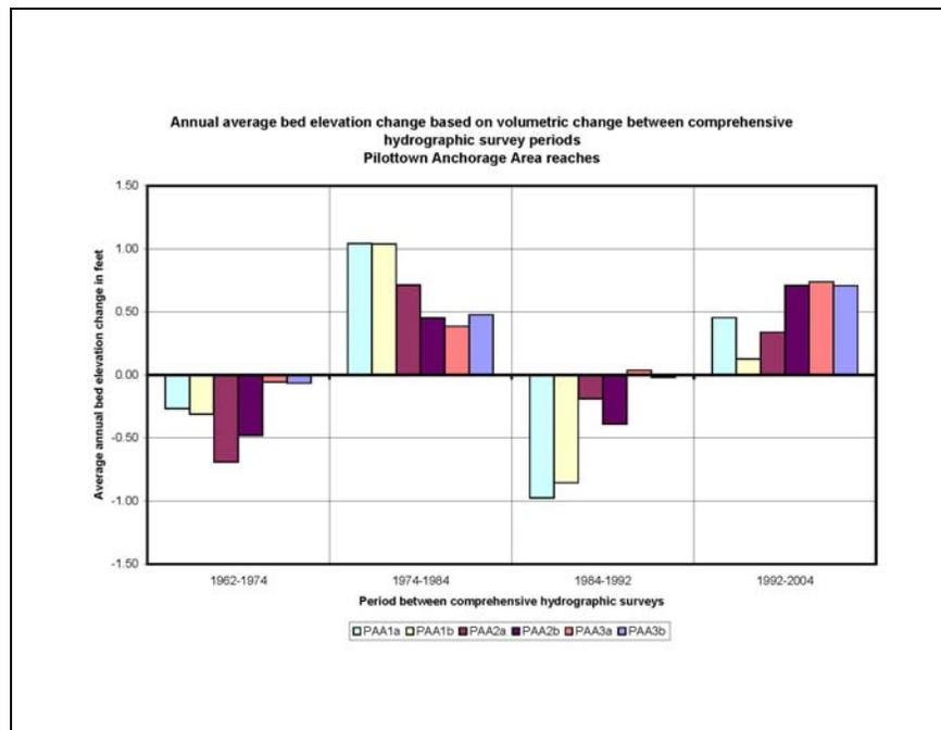
Figure 3.52. Annual average channel bed displacement based on comprehensive hydrographic surveys for the Pilottown anchorage area reaches.
