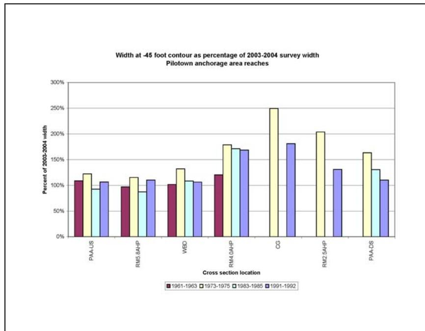
Figure 3.62. Channel widths at the -45 foot contour as a percentage of 2003-2004 width for cross sections located within the Pilotown anchorage area.
