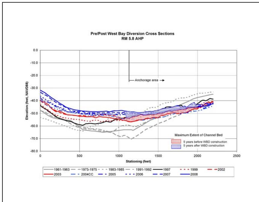
Figure 3.35. Maximum extent of channel bed elevation before and after West Bay diversion construction at RM 5.8 AHP.
