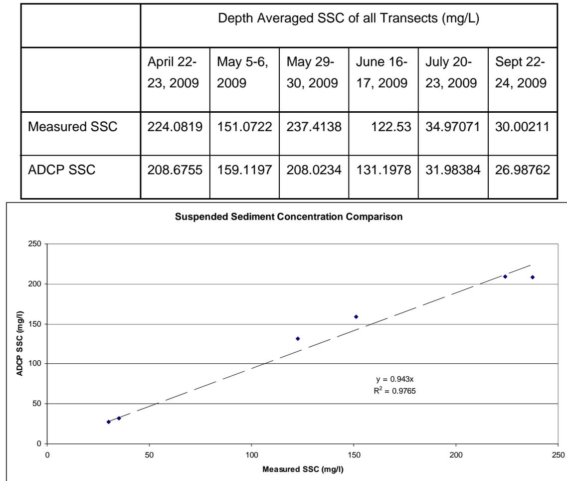
Figure 2.36. Average TSM values compared to Average TSM from Back Scatter Data
