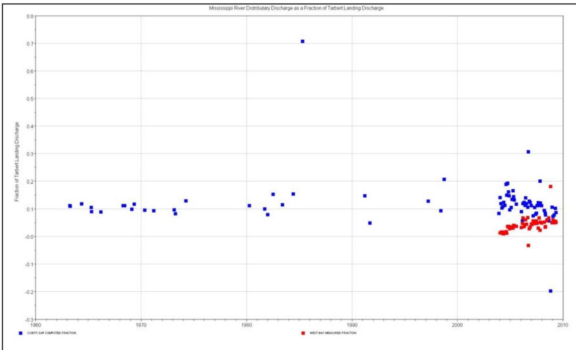
Figure 3.67. Discharge at Cubits Gap and West Bay diversion as a fraction of Tarbert Landing discharge.
