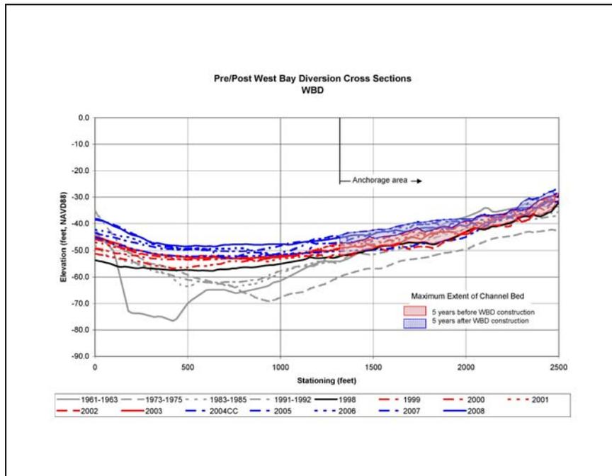
Figure 3.36. Maximum extent of channel bed elevation before and after West Bay diversion construction at West Bay diversion.
