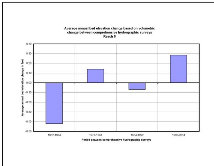
Figure 3.44. Annual average channel bed displacement between comprehensive survey periods for Reach 5.
