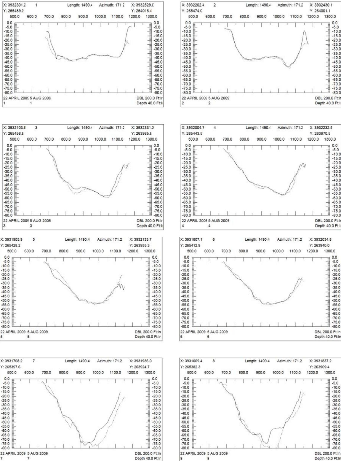
Figure 2.39. Cross Section Plots of the multi-beam surveys Lines 1-8.
