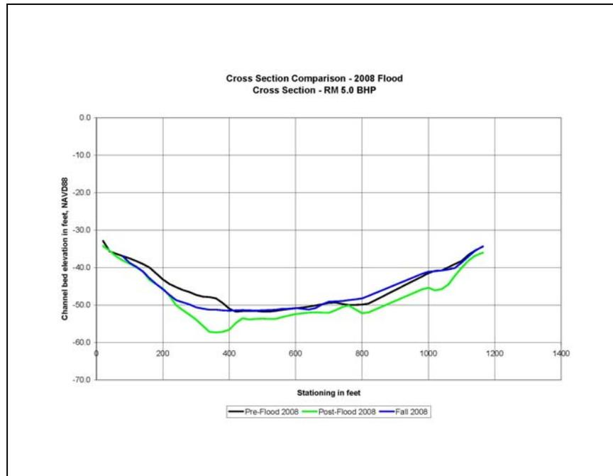
Figure 3.29. Cross section comparison for 2008 flood for cross section located at RM 5.0 BHP.
