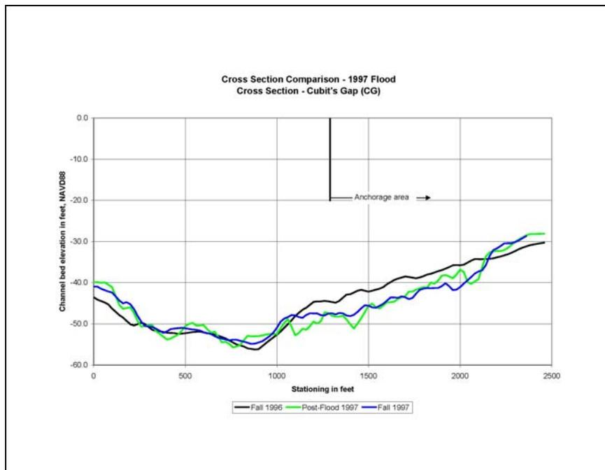
Figure 3.25. Cross section comparisons for 1997 flood for cross section located at downstream limit of Pilottown anchorage area.
