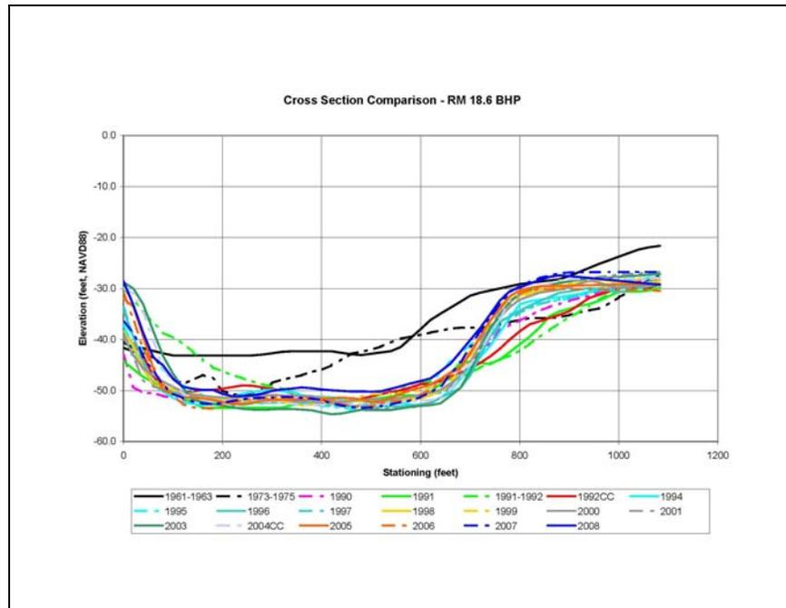
Figure 3.16. Cross section comparison for RM 18.6 BHP.
