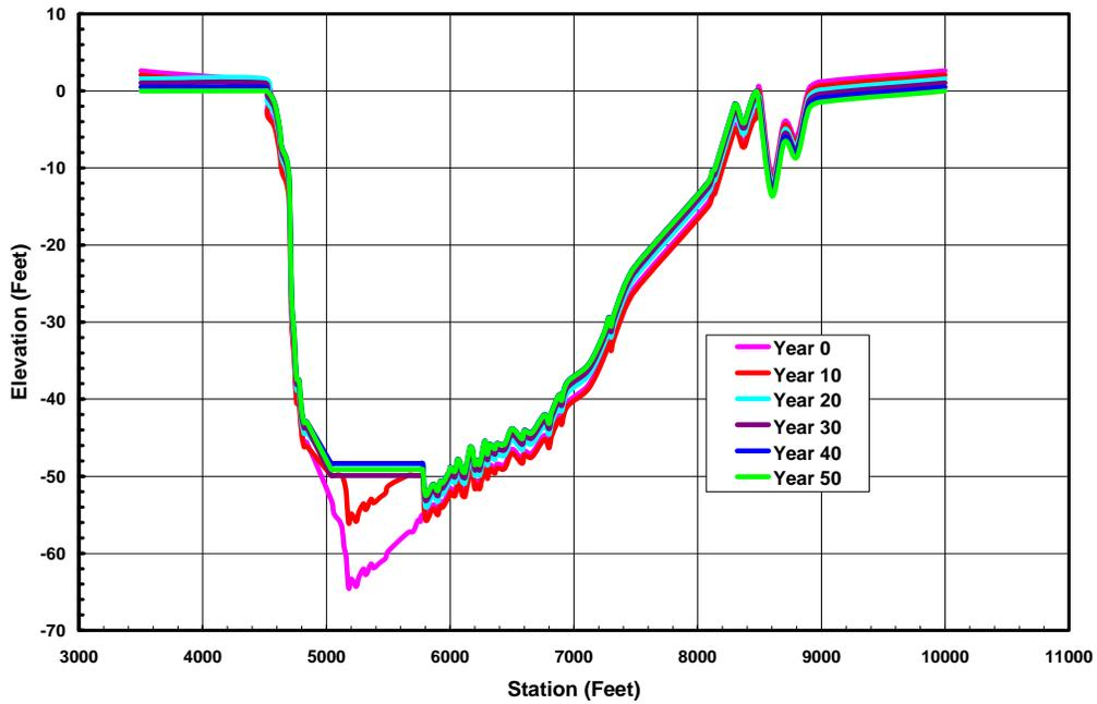
Figure 4.15. Channel Cross Section At River Mile 3.83 In 10 Year Intervals. West Bay Diversion Closed, No Dredging Allowed in PAA
