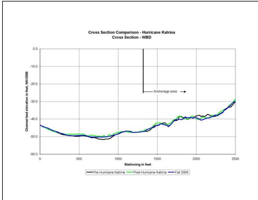
Figure 3.30. Cross section comparison for Hurricane Katrina for cross section located at West Bay diversion.
