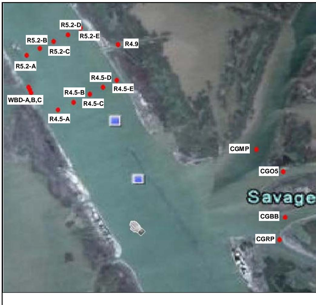
Figure 2.20. Locations of suspended sediment samples, OBS measurements, and salinity measurements.
