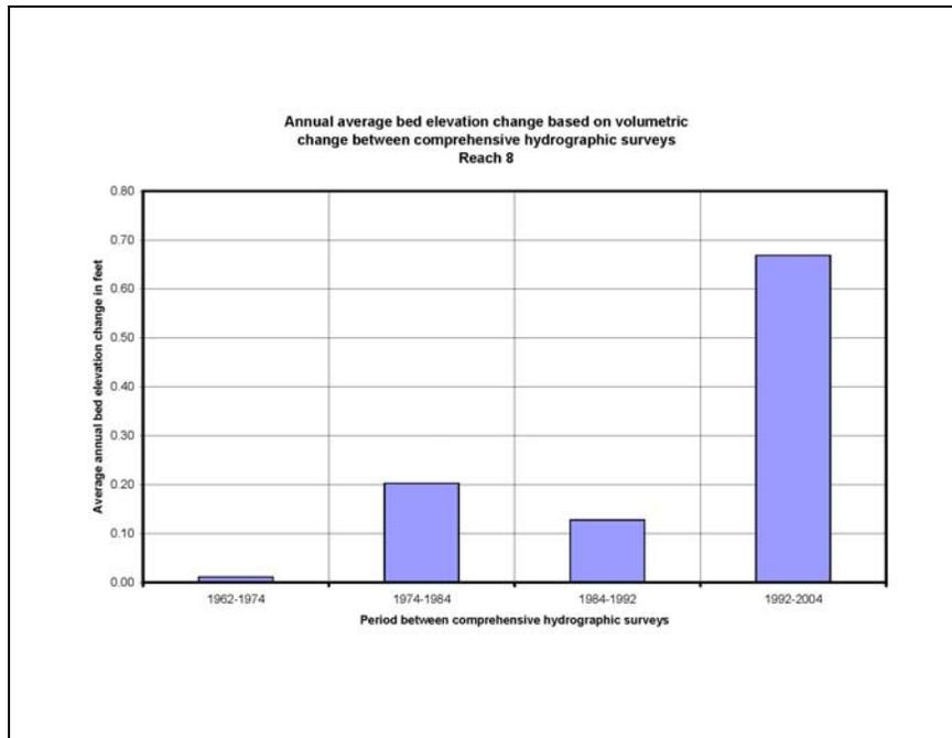
Figure 3.46. Annual average channel bed displacement between comprehensive survey periods for Reach 8.
