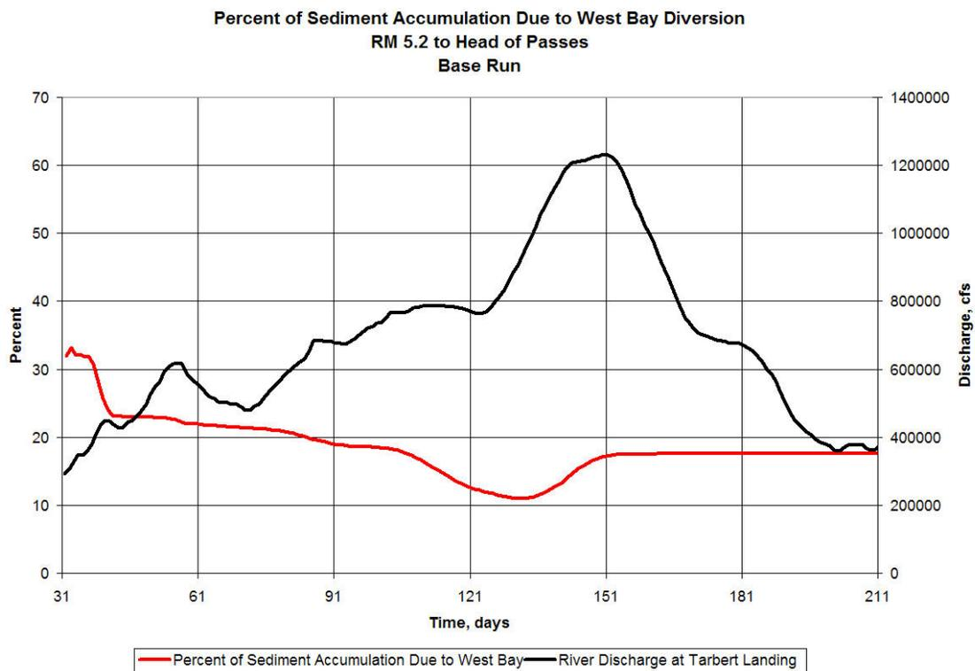
Figure 5.38. Percent increase in net deposition due to west bay diversion between RM 5.2 and Head of Passes, base run.
