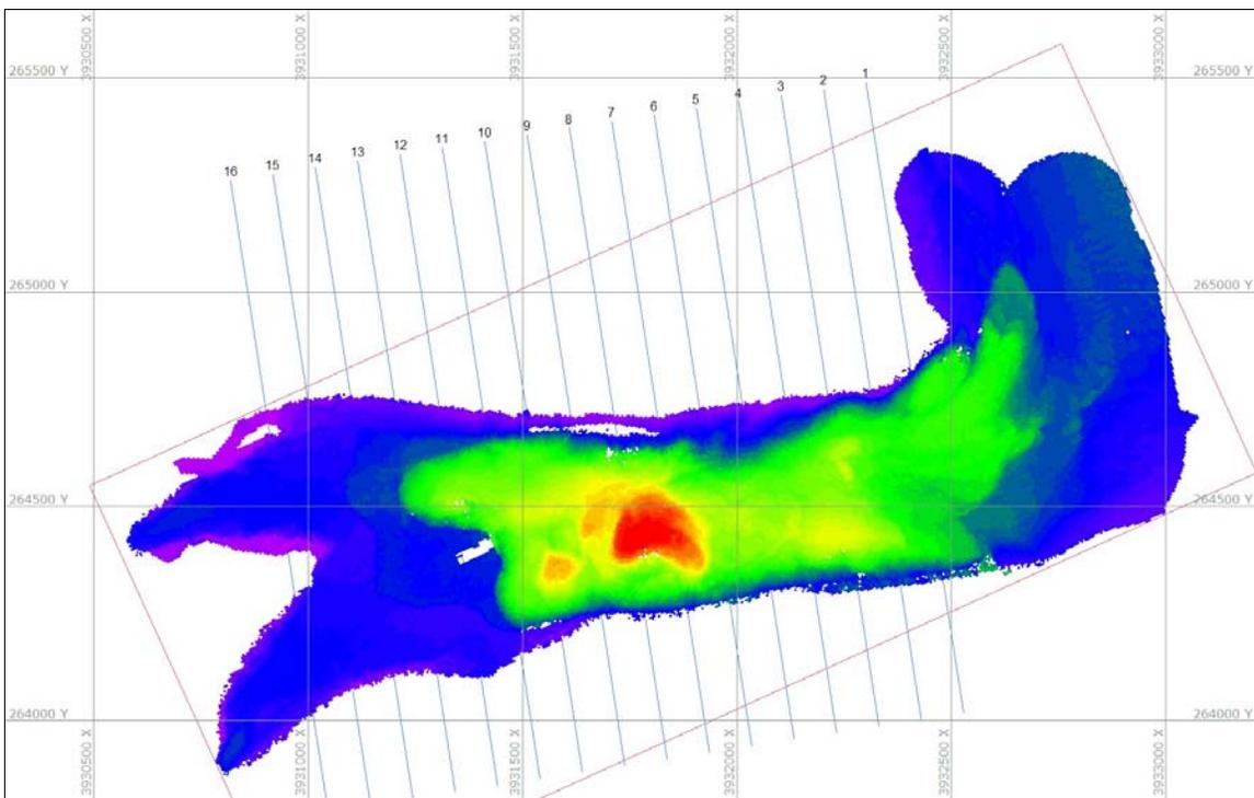
Figure 2.38. August Multi-beam Survey of the Diversion Cut.
