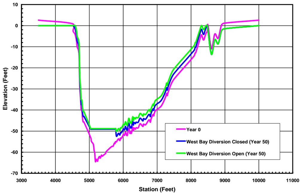
Figure 4.14. Channel Cross Section At River Mile 3.83 At Beginning and End of 50 Year Simulations. No Dredging In Pilottown Anchorage Area
