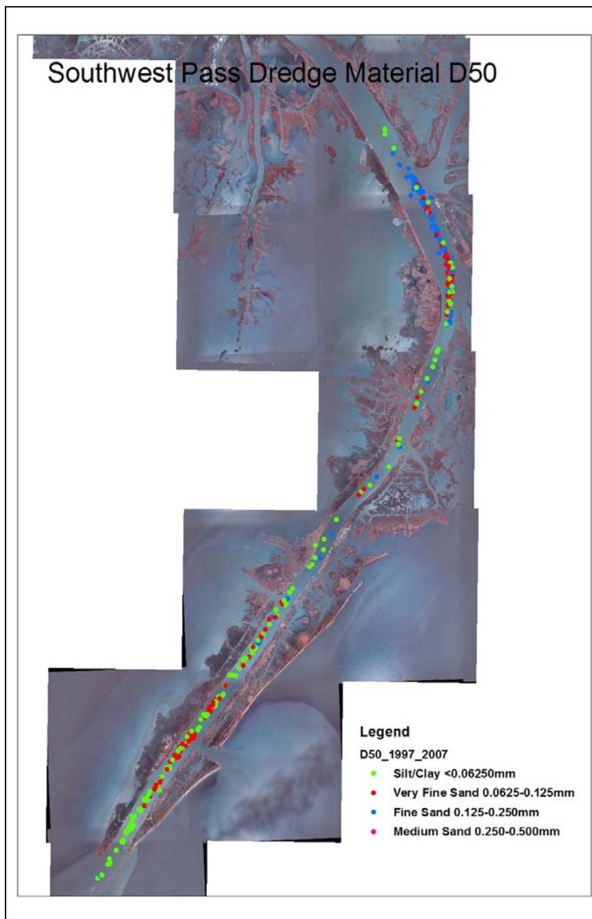
Figure 3.74. Dredge material grab sample location and D<sub>50</sub> grain size.
