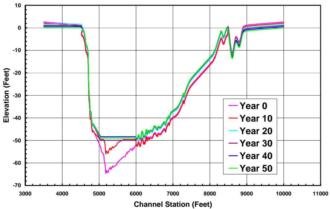
Figure 4.16. Channel Cross Section At River Mile 3.83 In 10 Year Intervals. West Bay Diversion Closed, Dredging Allowed in PAA
