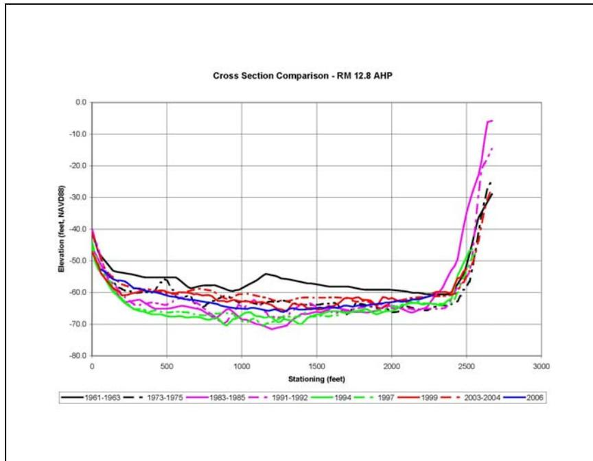
Figure 3.8. Cross section comparison for RM 12.8 AHP, just upstream of Baptiste Collette.
