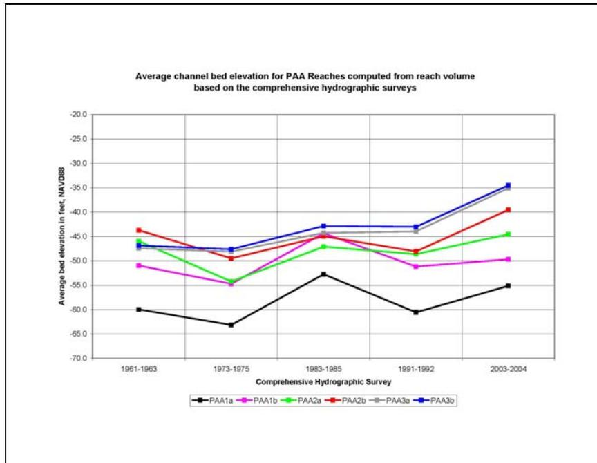
Figure 3.55. Average channel bed elevation computed from volume based on comprehensive surveys for Pilottown anchorage area reaches.
