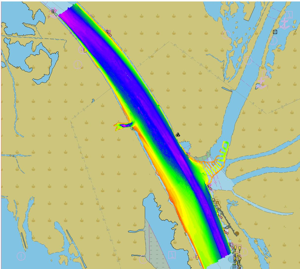
Figure 2.2. Multi-beam survey coverage.
