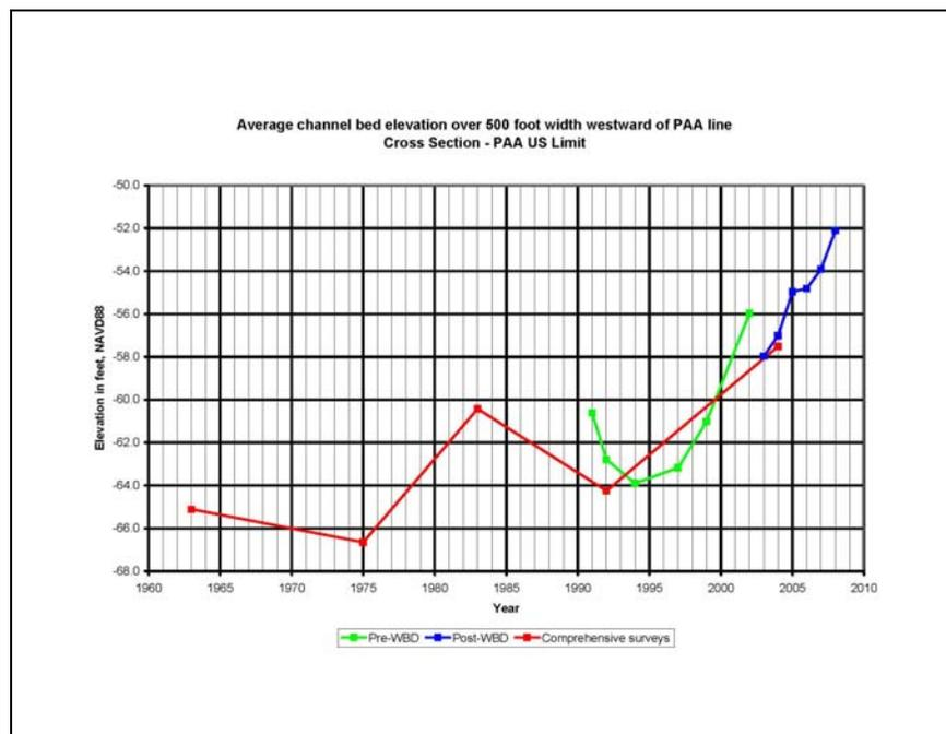
Figure 3.17. Comparison of average channel bed elevation for cross section located at the upstream limit of the Pilotown anchorage area.
