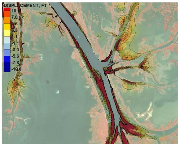
Figure 5.27. Cumulative bed change without West Bay Diversion, slug test run.
