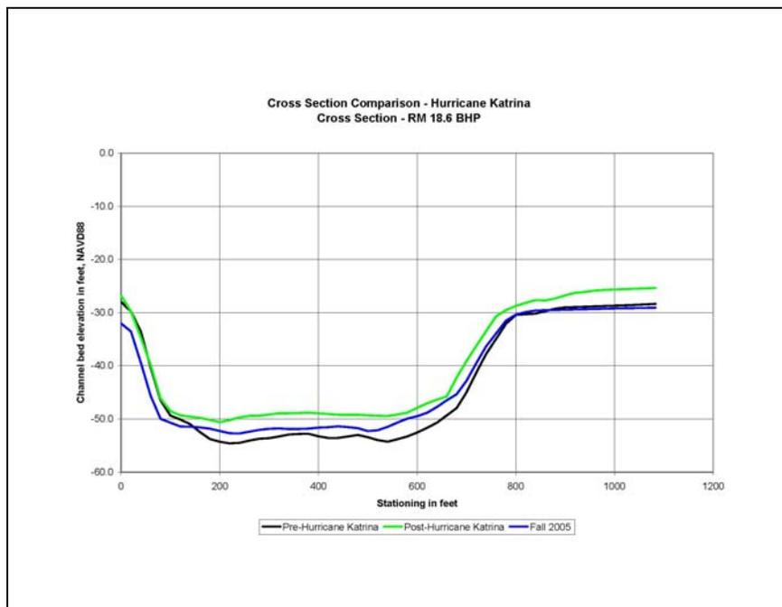
Figure 3.33. Cross section comparison for Hurricane Katrina for cross section located at RM 18.6 BHP.
