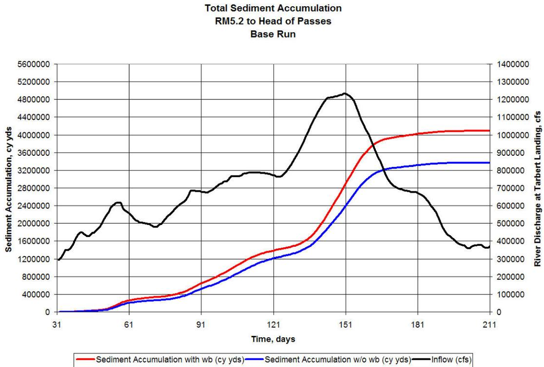
Figure 5.37. Net deposition within between RM 5.2 and Head of Passes, base run.
