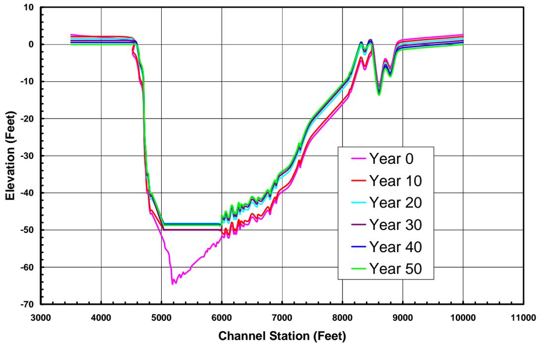
Figure 4.18. Channel Cross Section At River Mile 3.83 In 10 Year Intervals. West Bay Diversion Open, Dredging Allowed in PAA
