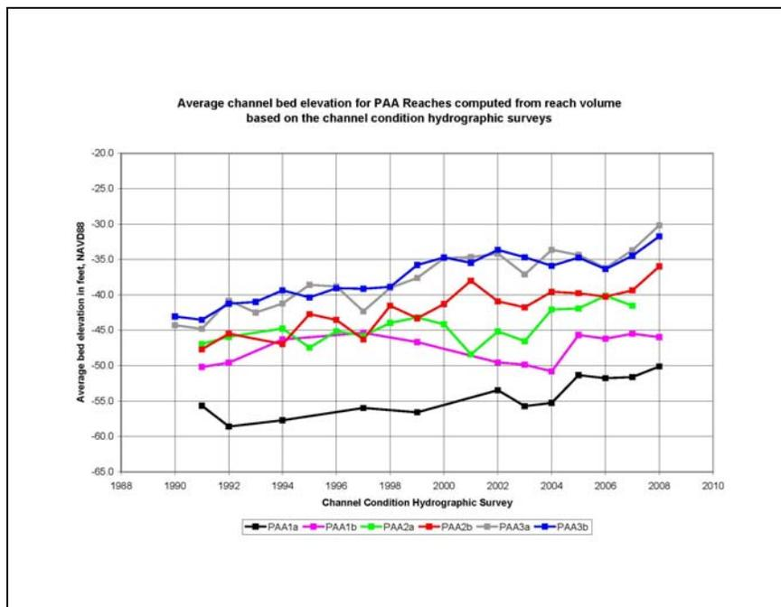
Figure 3.56. Average channel bed elevation computed from volume based on channel condition surveys for Pilottown anchorage area reaches.
