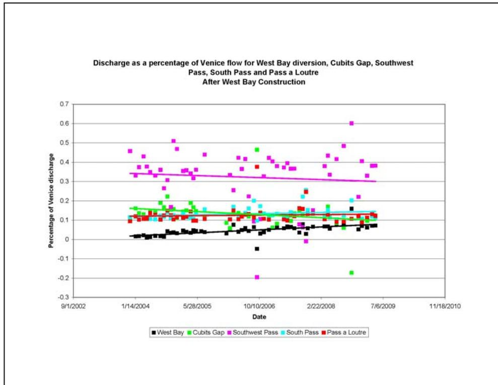
Figure 3.70. Capacity as a percentage of Venice discharge for the outlets downstream of West Bay diversion for the post-construction time period.
