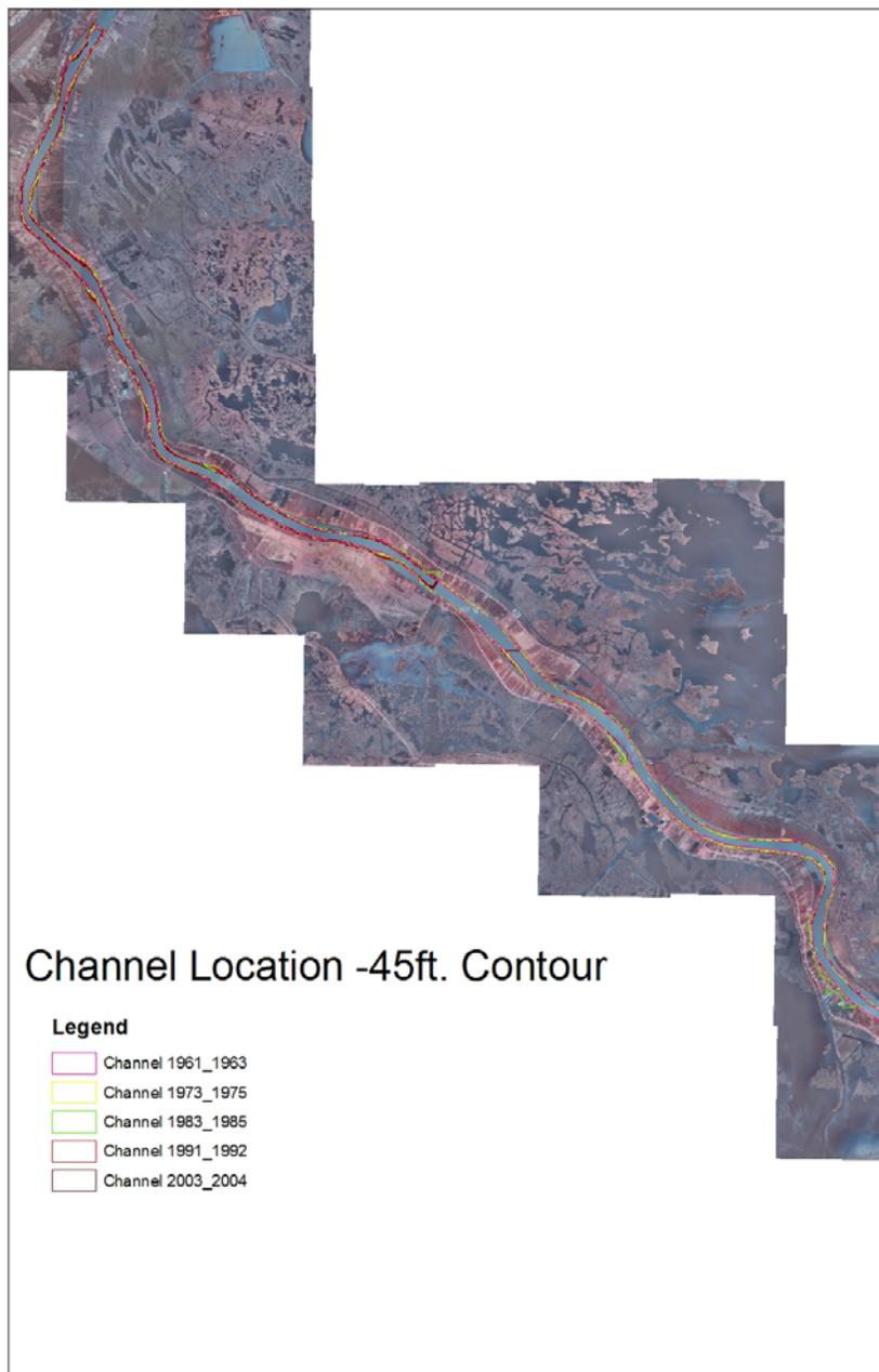
Figure 3.57. Channel location tracings of the -45 ft contour based on the comprehensive surveys from Belle Chase to near Venice.
