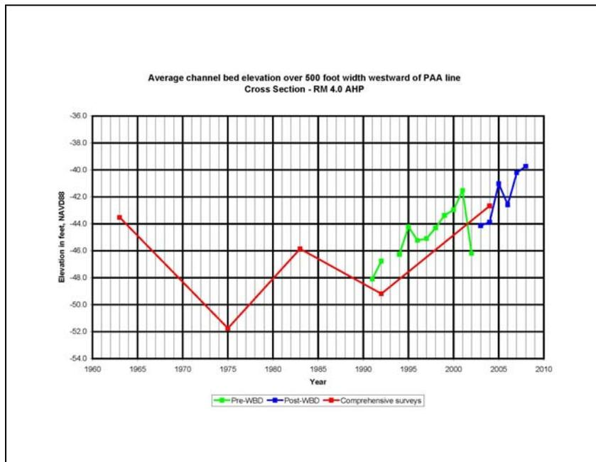
Figure 3.20. Comparison of average channel bed elevation for cross section located at RM 4.0 AHP.
