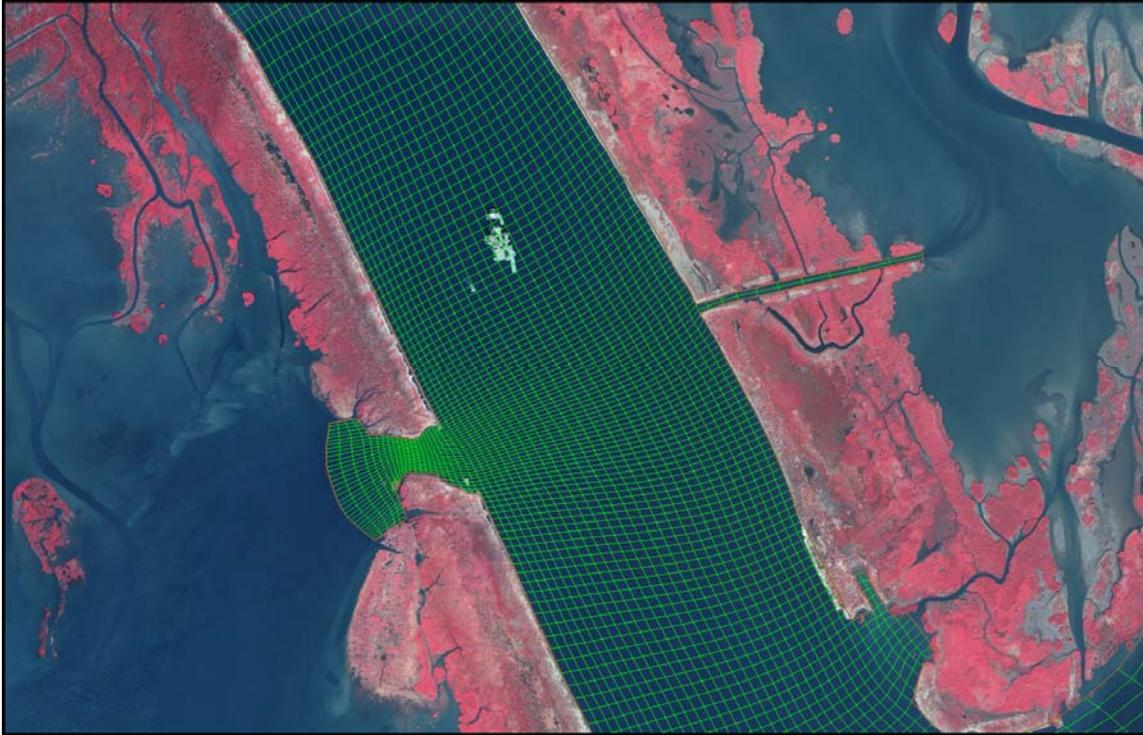
Figure 5.43. Grid Resolution at West Bay Diversion.
