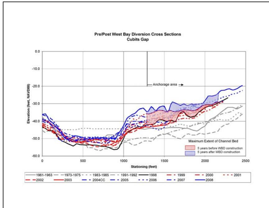
Figure 3.38. Maximum extent of channel bed elevation before and after West Bay diversion construction at Cubit's Gap.
