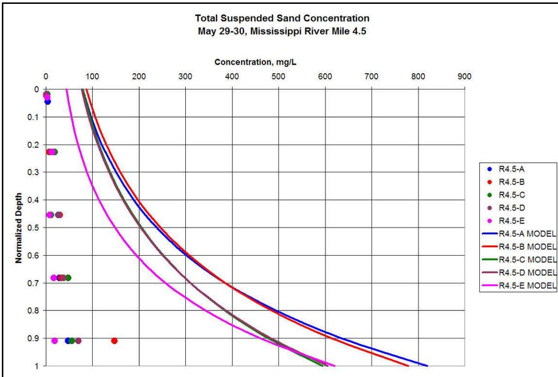
Figure 5.18. Suspended sediment verification at RM 4.5 for May 29-30.
