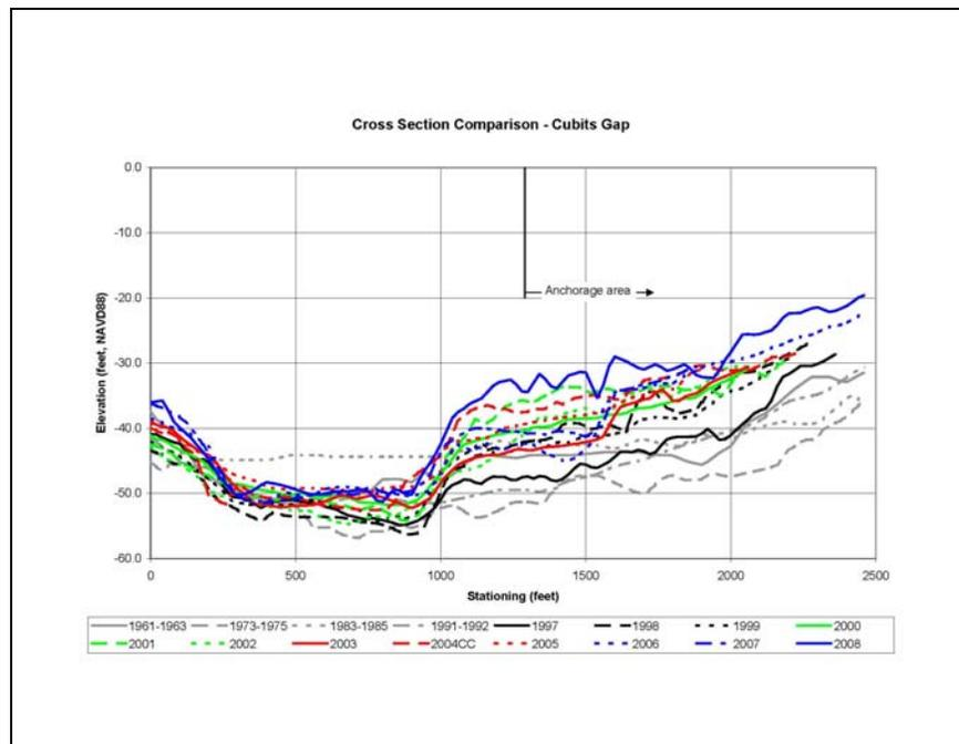
Figure 3.12. Cross section comparison for section located at Cubits Gap.
