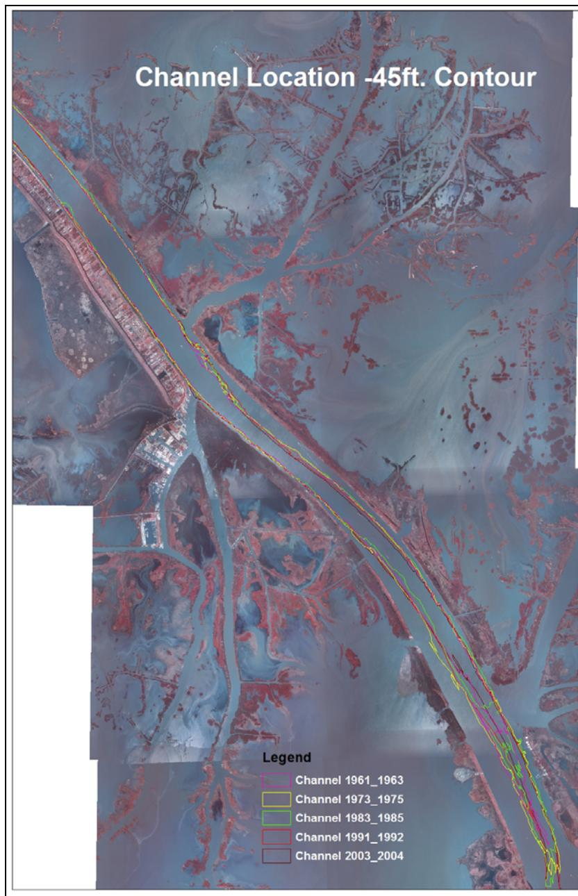
Figure 3.58. Channel location tracings of the -45 foot contour based on the comprehensive surveys from Venice to near Head of Passes.
