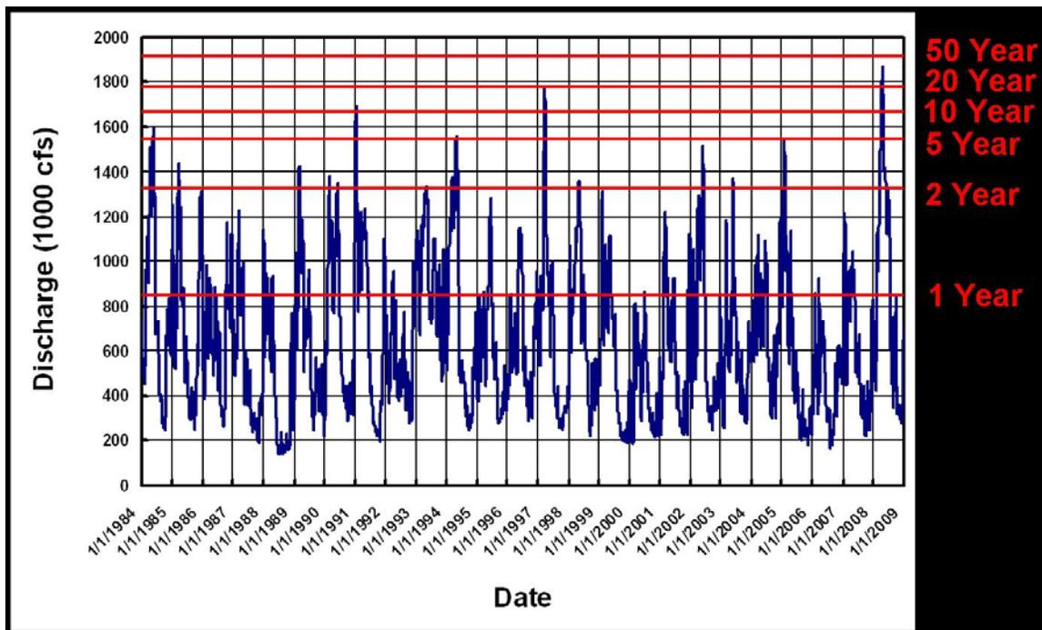
Figure 4.11. Typical Discharge Hydrograph At Vicksburg, MS
