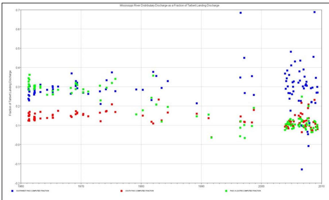
Figure 3.69. Discharge at Southwest Pass, South Pass and Pass a Loutre as a fraction of Tarbert Landing discharge.
