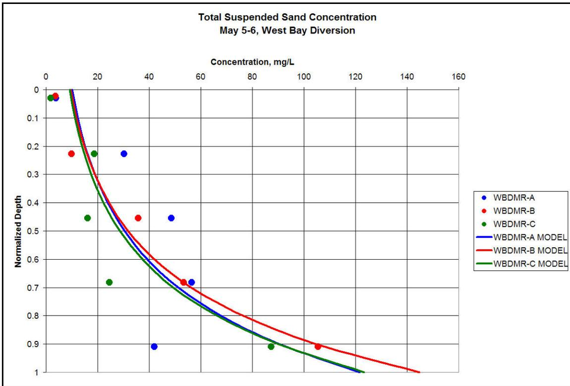
Figure 5.14. Suspended sediment verification at WBD for May 5-6.
