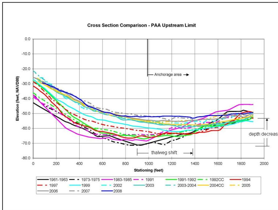
Figure 3.10. Cross section comparison for cross section located at the upstream limit of the Pilottown anchorage area.
