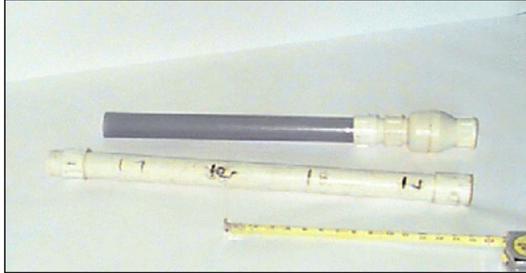
Figure 2.1. Push-core sampler.
