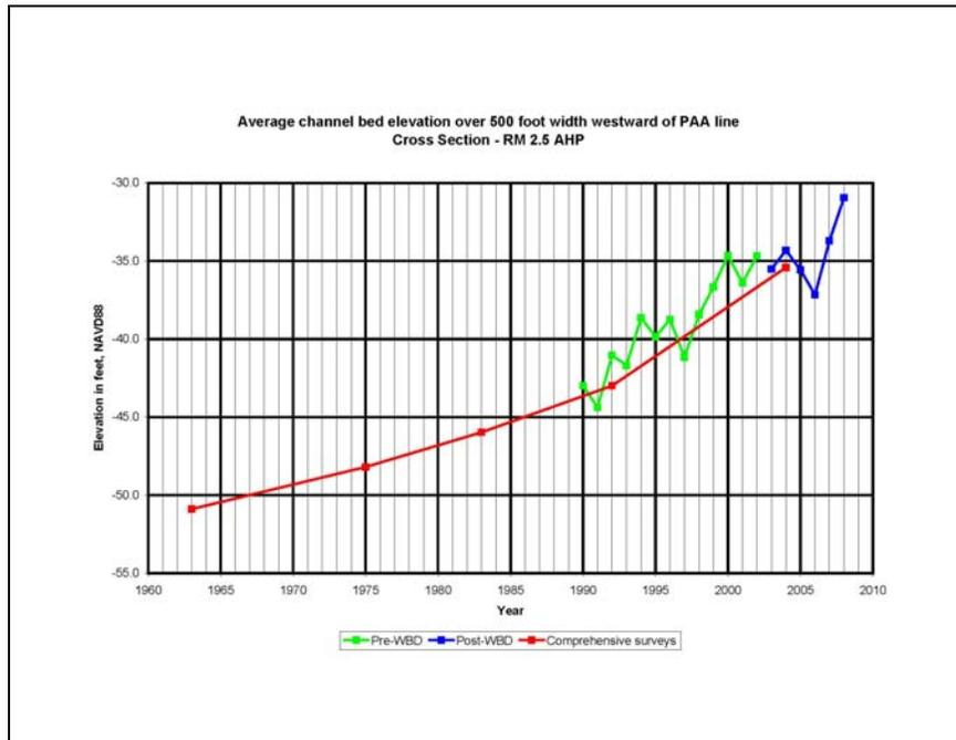
Figure 3.22. Comparison of average channel bed elevation for cross section located at RM 2.5 AHP.
