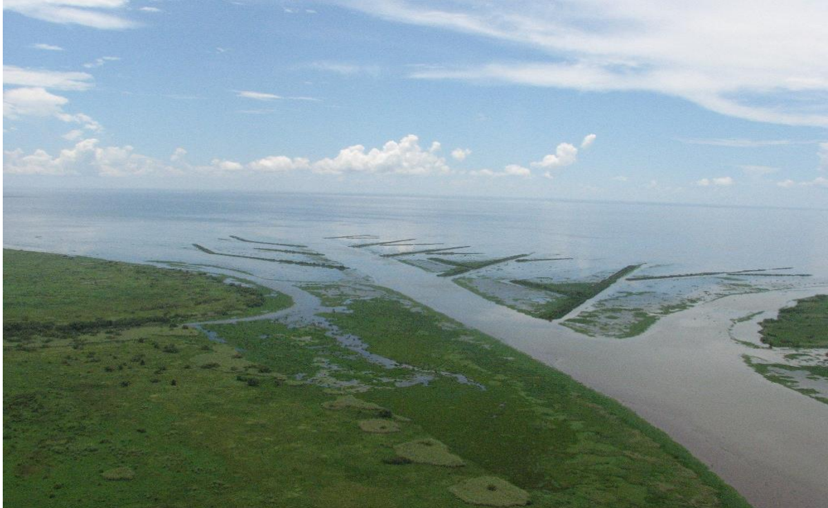
Figure 11. Sediment Trapping at the Jaws (TV-15) 2012 aerial photo looking southwest showing large swaths of SAV, FAV, and some emergent marsh on inter-terrace mudflats.
