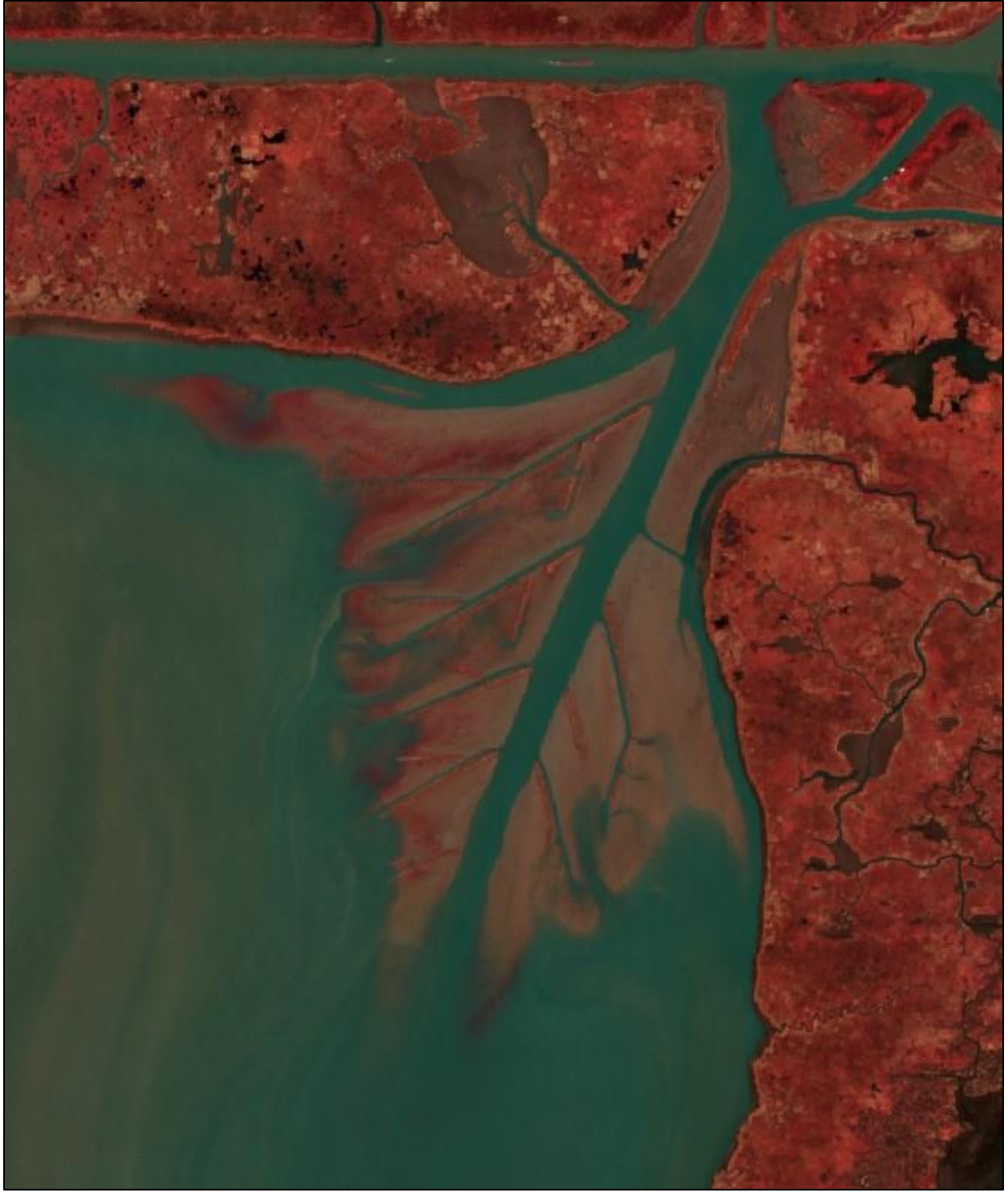
Figure 26. Sediment Trapping at the Jaws (TV-15), a Sentinel-2 L2A satellite color inferred image on 2-19-2021 showing extensive mudflats in the project area (-0.685 water elevation NAVD GEOID 12A). There is a general trend of higher elevation mudflats in the northeast project area and along channels, which gradually tapering downward toward the bay.
