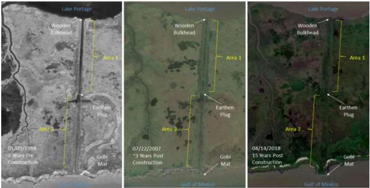
Figure 3. A time series of aerial imagery of TV-0017 Areas 1 and 2 from 6 years preconstruction to 14 years post construction was obtained from GoogleEarth. The images show pre-existing features of the pipeline in white and the TV-0017 in-fill (Area 1) and nourishment (Area 2) areas.
