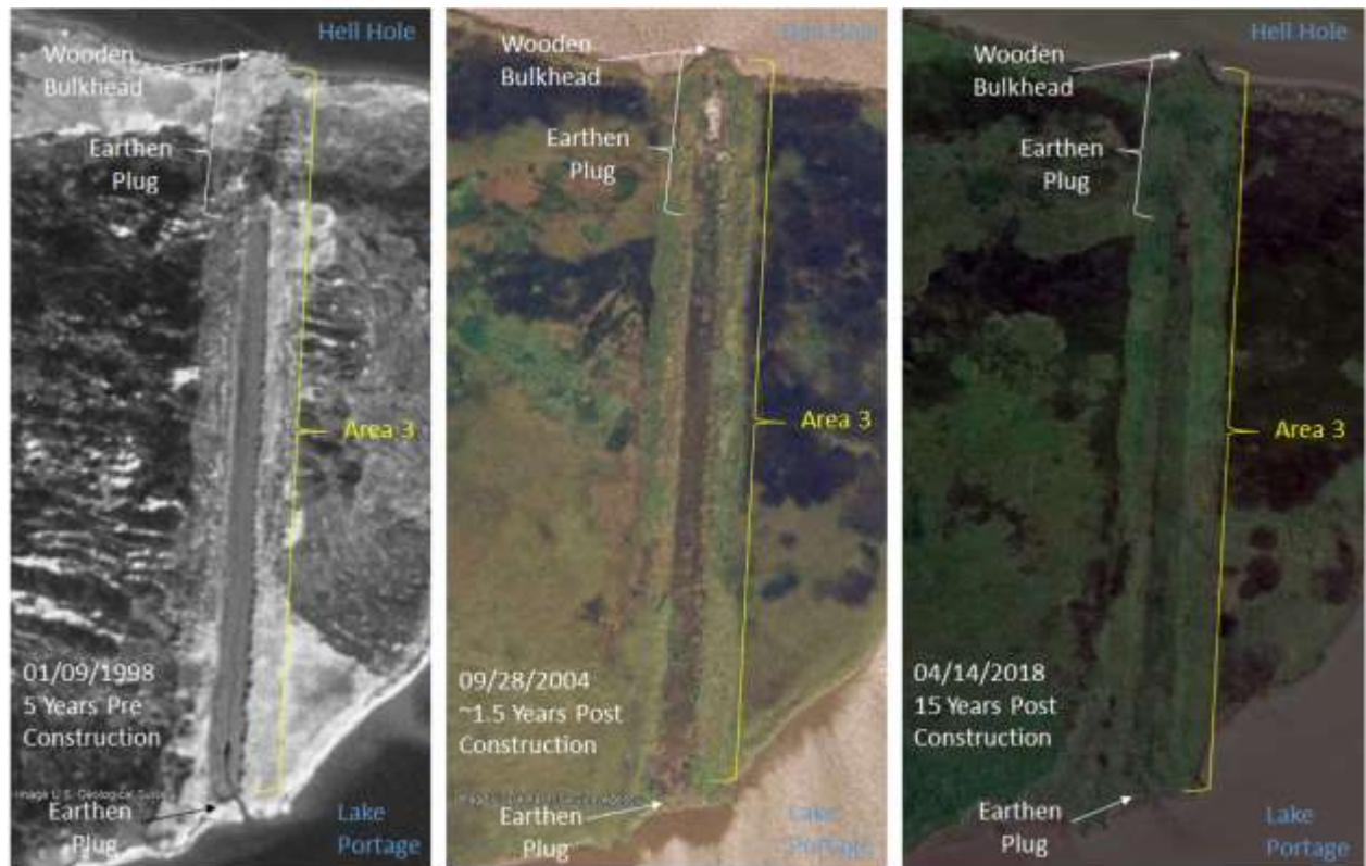
Figure 5. A time series of aerial imagery of TV-0017 Area 3 from 5 years preconstruction to 15 years post construction was obtained from GoogleEarth. The images show pre-existing features of the pipeline and in white and TV-0017 in-fill area.
