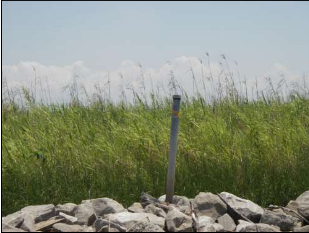
Figure 6. Settlement plate 1007 in the Vermilion River Cutoff (TV03) project at the southern end of the rock breakwater.
