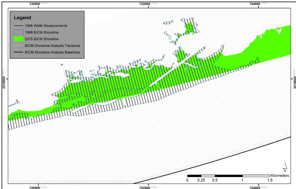
Figure B2. Example of the BICM shoreline measurement baseline and transects along a portion of Trinity/East Island overlain on the 1998 and 2015 datasets. Standardized measurement transects were used for all analysis including shoreline positions, island lengths, and average island widths. Note the measurement transects clipped to the island outline and used to calculate the island width along each transect in 1998.
