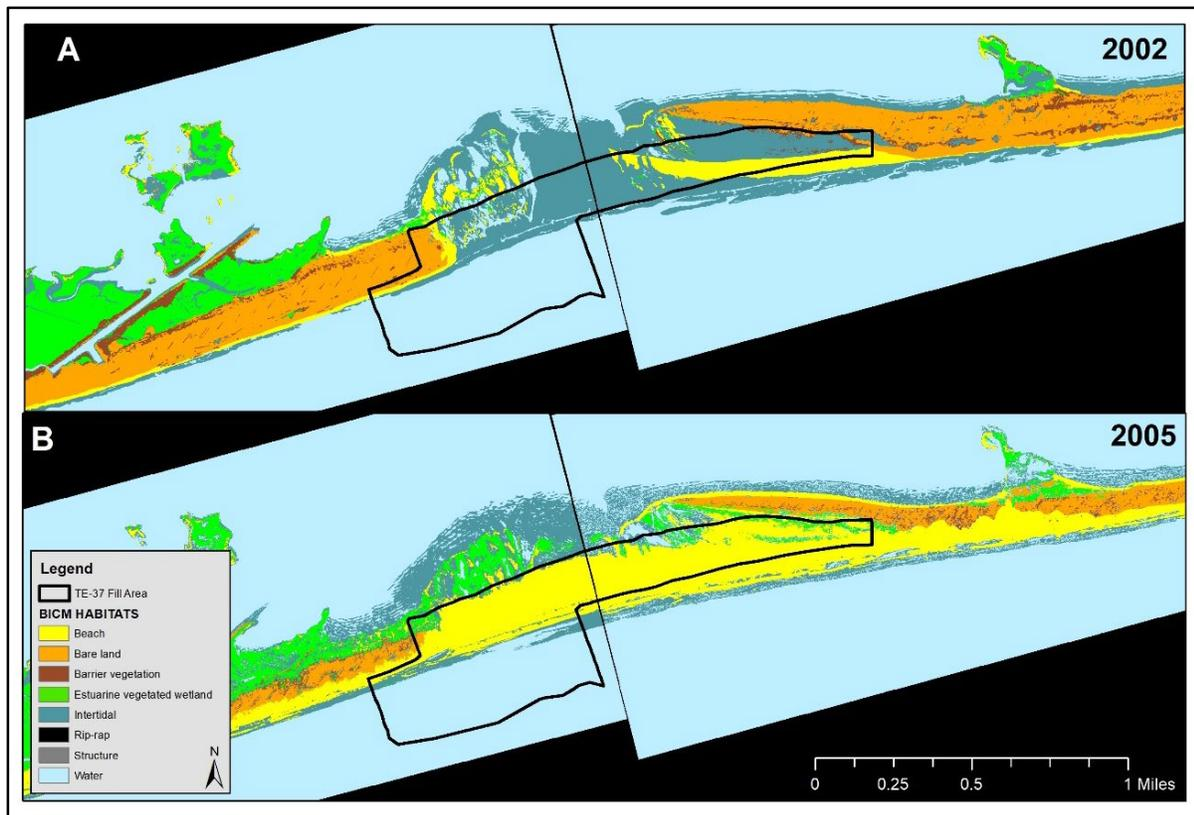
Figure 5. BICM habitat data in 2002 (A) and 2005 (B) indicating the conversion of water to land prior to the TE-37 project in 2007. The TE-37 fill area (outlined in black) is overlain to show the area the project will impact.
