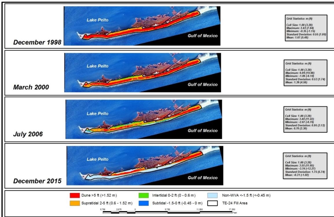
Figure C 2. Elevation classification of the analysis area for the Isles Dernieres Restoration Trinity Island (TE-24) project for four time periods from as-built (1998) to seventeen years post-construction (2015).
