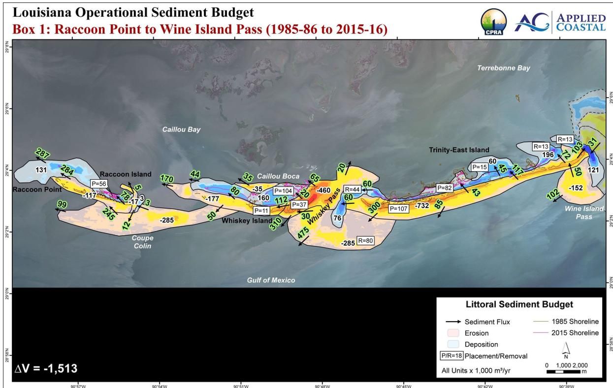
Figure 7. Detailed sediment transport pathways and quantities for Box 1 of the macro-scale sediment budget, 1985-86 to 2015-16. Arrows represent the direction of sediment movement, and black numbers with green border reflect the magnitudes of net sediment transport in thousands of m<sup>3</sup>/yr. Black numbers with white border represent net volume change for a particular zone. (from ACRE 2020).
