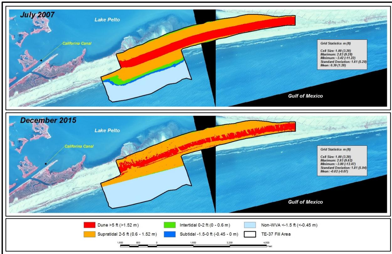
Figure C4. Elevation classification of the analysis area for the New Cut Dune and Marsh Restoration (TE-37) project for two time periods from as-built (2007) to eight years post-construction (2015).
