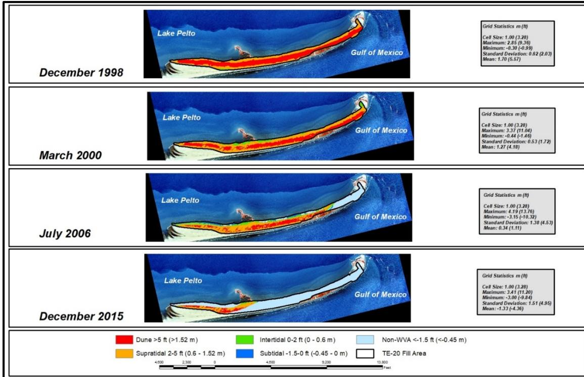
Figure C 1. Elevation classification of the analysis area for the Isles Dernieres Restoration East Island (TE-20) project for four time periods from as-built (1998) to seventeen years post-construction (2015).
