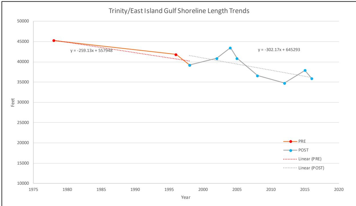
Figure B4. Island lengths at Trinity and East Islands from 1978 to 2016. Note the increase in length from 1998 through 2005 as New Cut filled with sediment and created a contiguous island. However, the overall trend indicates island shortening over time regardless of the initial increase in length, with a post-restoration shortening rate 17% greater than pre-restoration.
