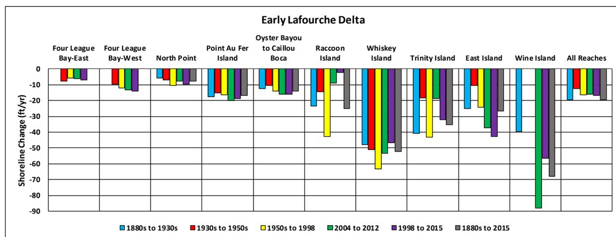
Figure B6. BICM shoreline change for the Early Lafourche Delta (from Byrnes et al. 2018). Note the Trinity Island reduction in erosion post restoration (1998-2015), while East Island exhibits a large increase during this period.
