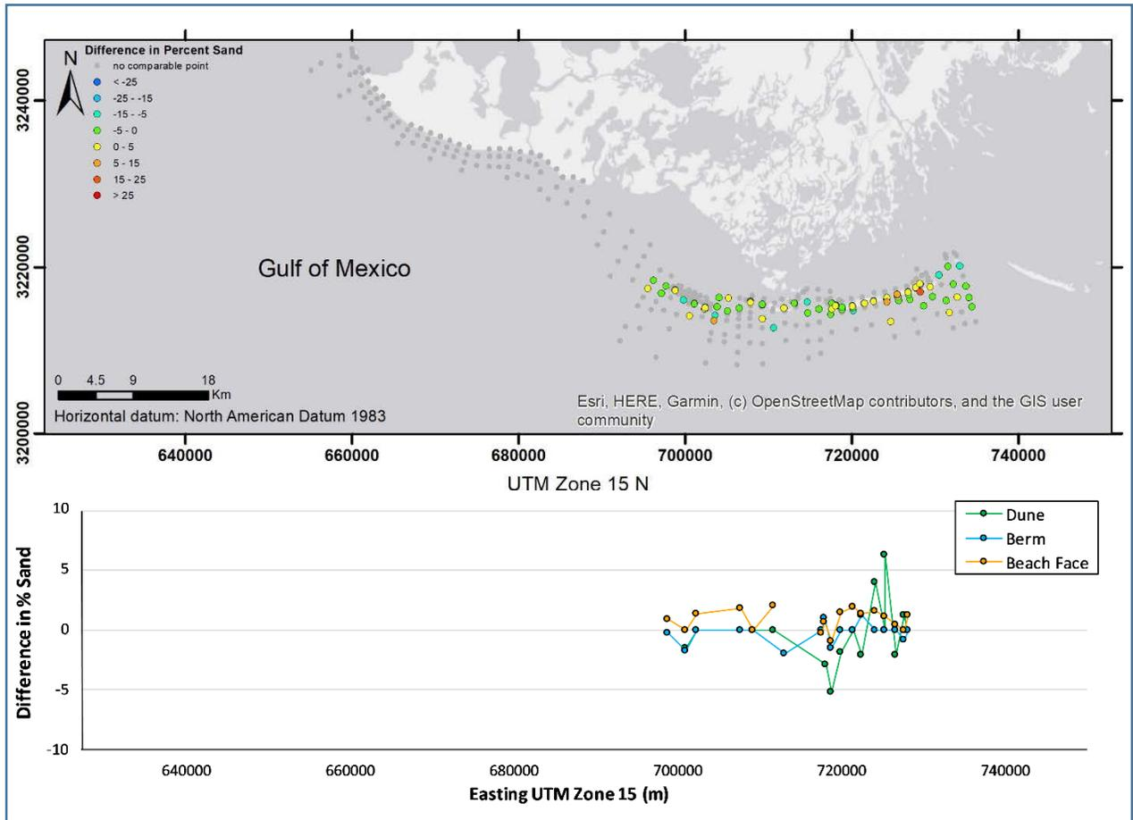
Figure 12. Differences in sand content along the Early Lafourche Delta from 2008 to 2015 in plan view (top) and graphically (bottom) for onshore environment (dune, berm and beach face). Note numbers above zero indicate increases in sand content with decreases less than zero (from Georgiou et al. 2019).
