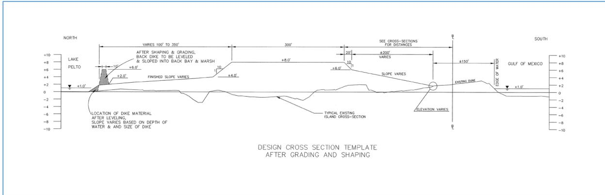
Figure 6. Typical construction template cross section at TE-24 showing the fill placement behind the existing shoreline.
