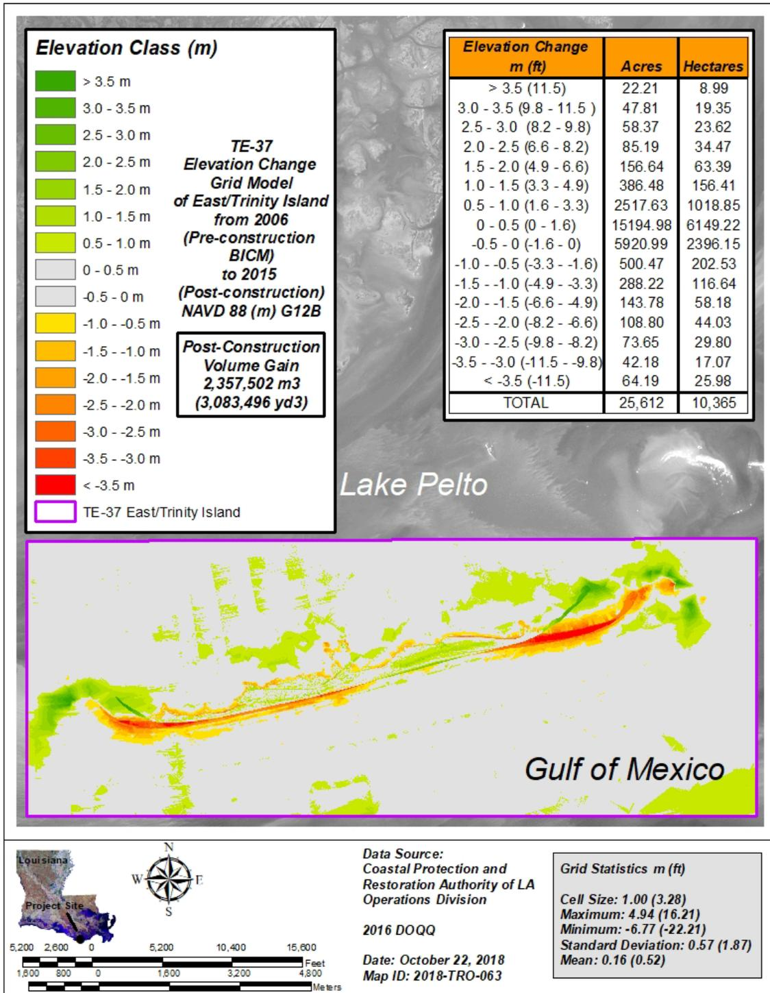
Figure C5. Elevation change surface, 2006 to 2015/16 at Trinity/East Island. Yellows and reds illustrate erosion areas; greens illustrate deposition areas. Grey areas represent areas within model uncertainties and are excluded from the volume calculations.
