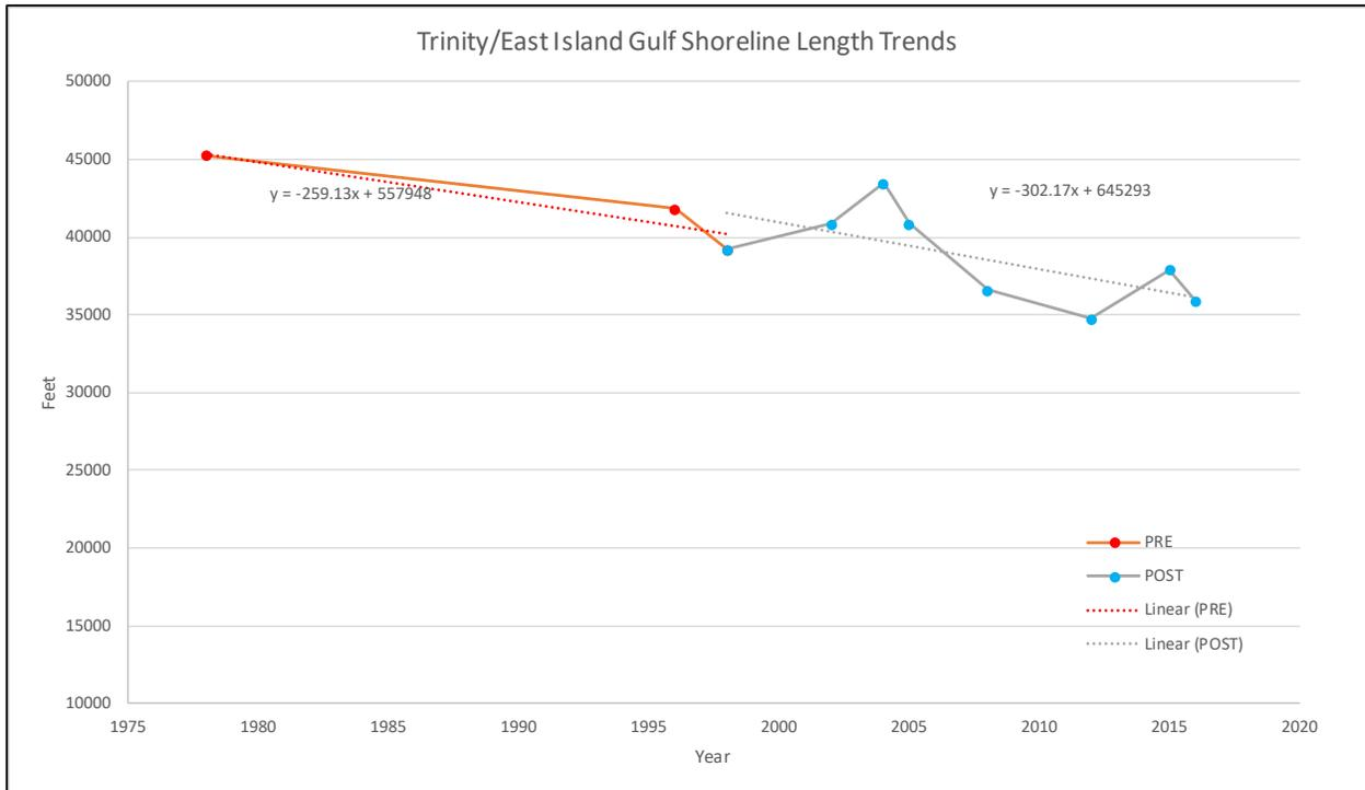
Figure 8. Island lengths at Trinity and East Islands from 1978 to 2016. Note the increase in length from 1998 to 2005 as New Cut filled with sediment and created a contiguous island. The overall trend indicates island shortening over time regardless of the initial increase in length. The post restoration shortening rate is 17% greater than the pre-restoration rate.
