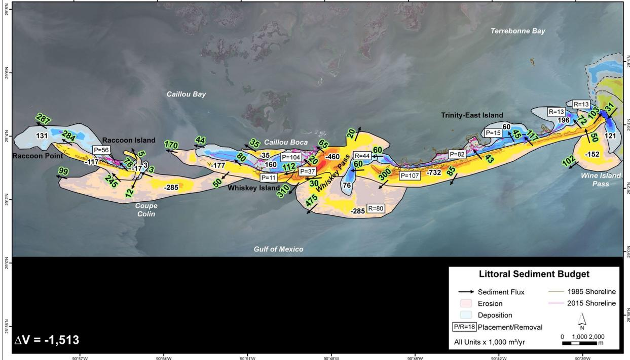
Figure C6. Detailed sediment transport pathways and quantities for the Isle Dernieres for the macro-scale sediment budget, 1985-86 to 2015-16. Arrows represent the direction of sediment movement, and black numbers with green border reflect the magnitudes of net sediment transport in thousands of m<sup>3</sup>/yr. Black numbers with white border represent net volume change for a particular zone. (from ACRE 2020).
