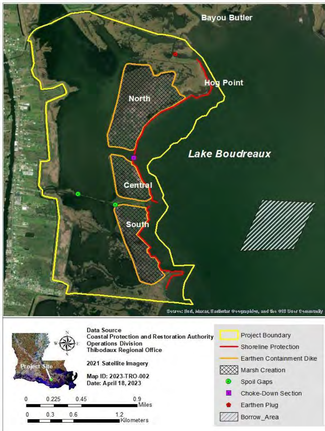
Figure 2. Map indicating the locations and types of constructed features inside the boundary of the West Lake Boudreaux Shoreline Protection and Marsh Creation (TE-0046) project.
