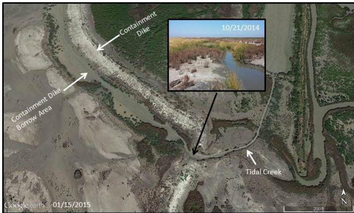
Figure 27. Jan 2015 Google Earth image and Oct 2014 oblique image depicting tidal connectivity and vegetation colonization through the gapped containment dike at the West Belle Pass Barrier Headland Restoration (TE-52) project. Note the vegetation colonization along the edges of the low elevated containment dike borrow area.
