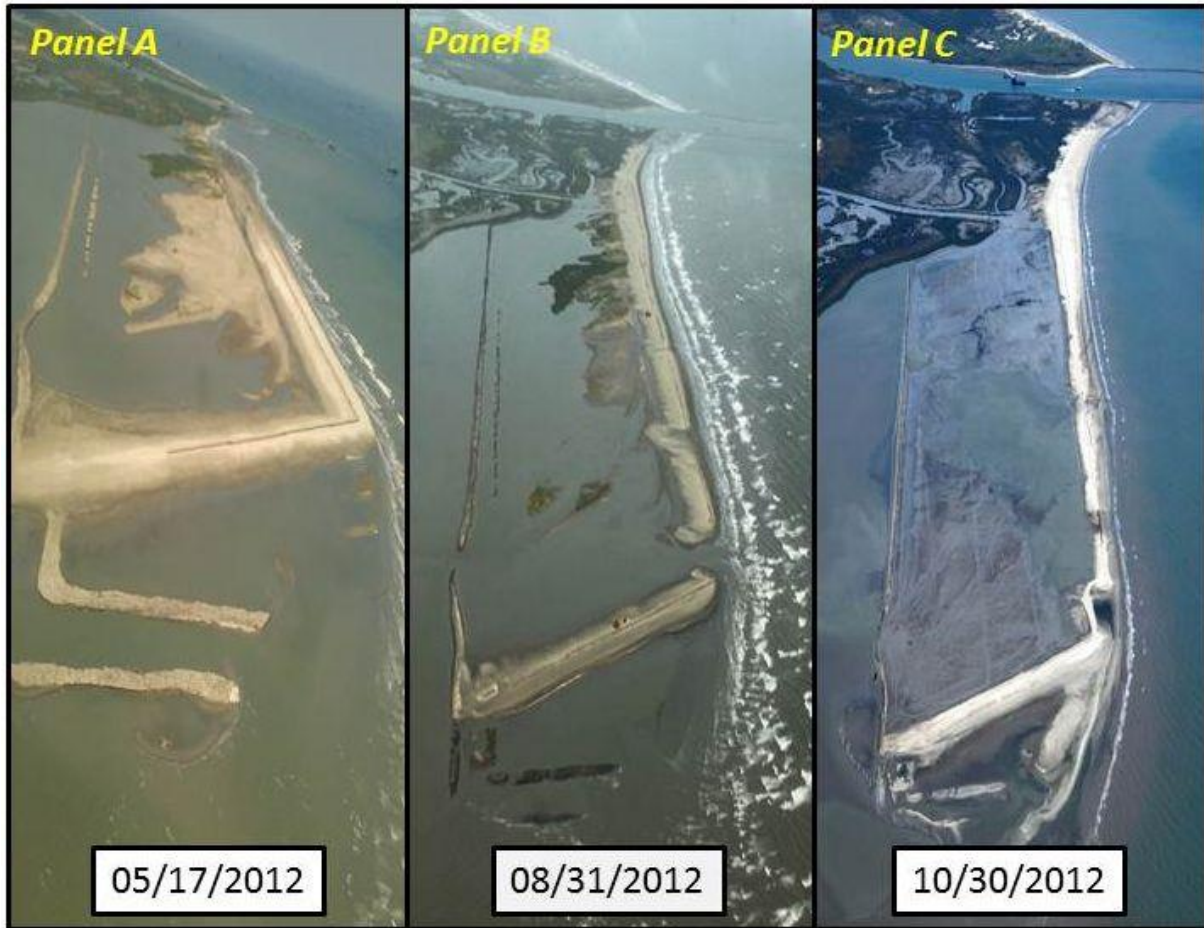
Figure 10. Oblique aerial images depicting the West Belle Pass Barrier Headland Restoration (TE-52) project before (Panel A) and after (Panel B) Hurricane Isaac and after dredging operations were complete (Panel C). Panels A and B were taken before marsh creation activates began. The earthen structure in the foreground of Panel A is the floatation channel spoil and can be seen in subsequent photographs. Note the breaching of the primary containment dike and the dune by the hurricane (Panel B) and the embryonic stages of the spit development in Panels B and C. Also note the offset position of the dune in the breached area and erosion along the Gulf of Mexico shoreline in panel C and the large volume of sand that was overwashed into the marsh creation area during beach and dune construction in panel A.
