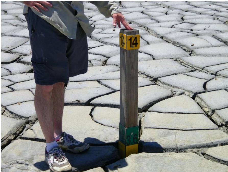
Photo 22: TE-48 marsh creation area settlement gage #14 (Raccoon_164). Note persons could access by walking and settlement indicated approx. 3.5 ft elevation.
