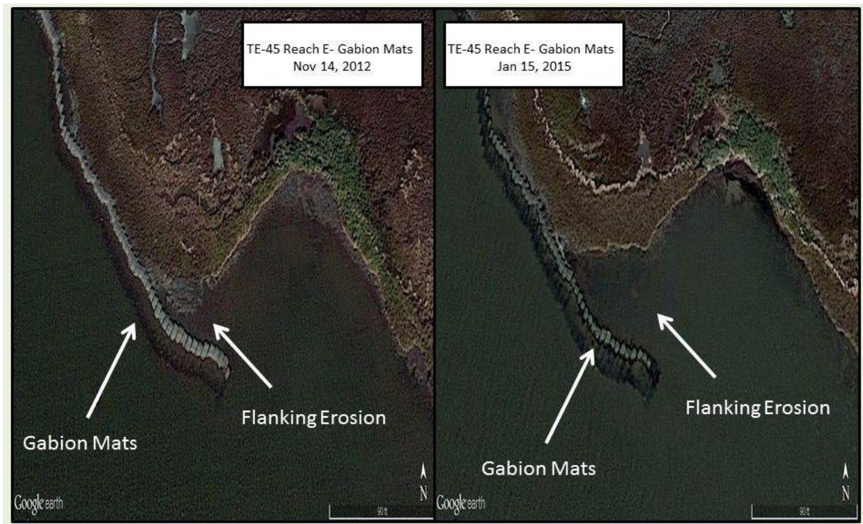
Figure 19. November 14, 2012 and January 15, 2015 images depicting flanking erosion behind the Reach E Gabion Mat treatment at the Terrebonne Bay Shore Protection Demonstration (TE-45) project. Note the increased erosion in 2015. Images reproduced from Google Earth.
