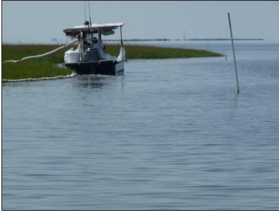
Figure 28. Boat laying oil boom in summer 2010 at Reach E because of the DWH oil spill in the Gulf of Mexico. Boom is being laid on a high tide as boat travels between marsh shoreline and bio-engineered structures.
