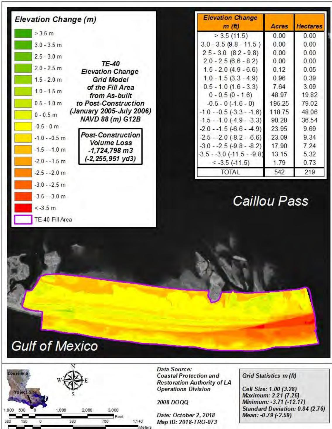
Figure 4-2. Elevation and volume change grid model for the TE-40 fill area from as-built (Jan 2005) to post-construction 1 (Jul 2006) at the Timbalier Island Dune and Marsh Restoration (TE-40) project.
