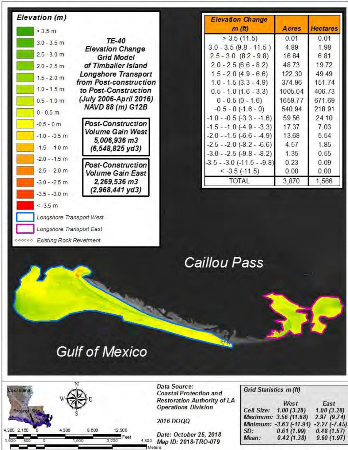
Figure 4-5. Elevation and volume change grid model depicting longshore transport along Trinity Island from Jul 2006 to Apr 2016. This timeline represents the post-construction 1 to the post-construction 2 interval for the Timbalier Island Dune and Marsh Restoration (TE-40) project..
