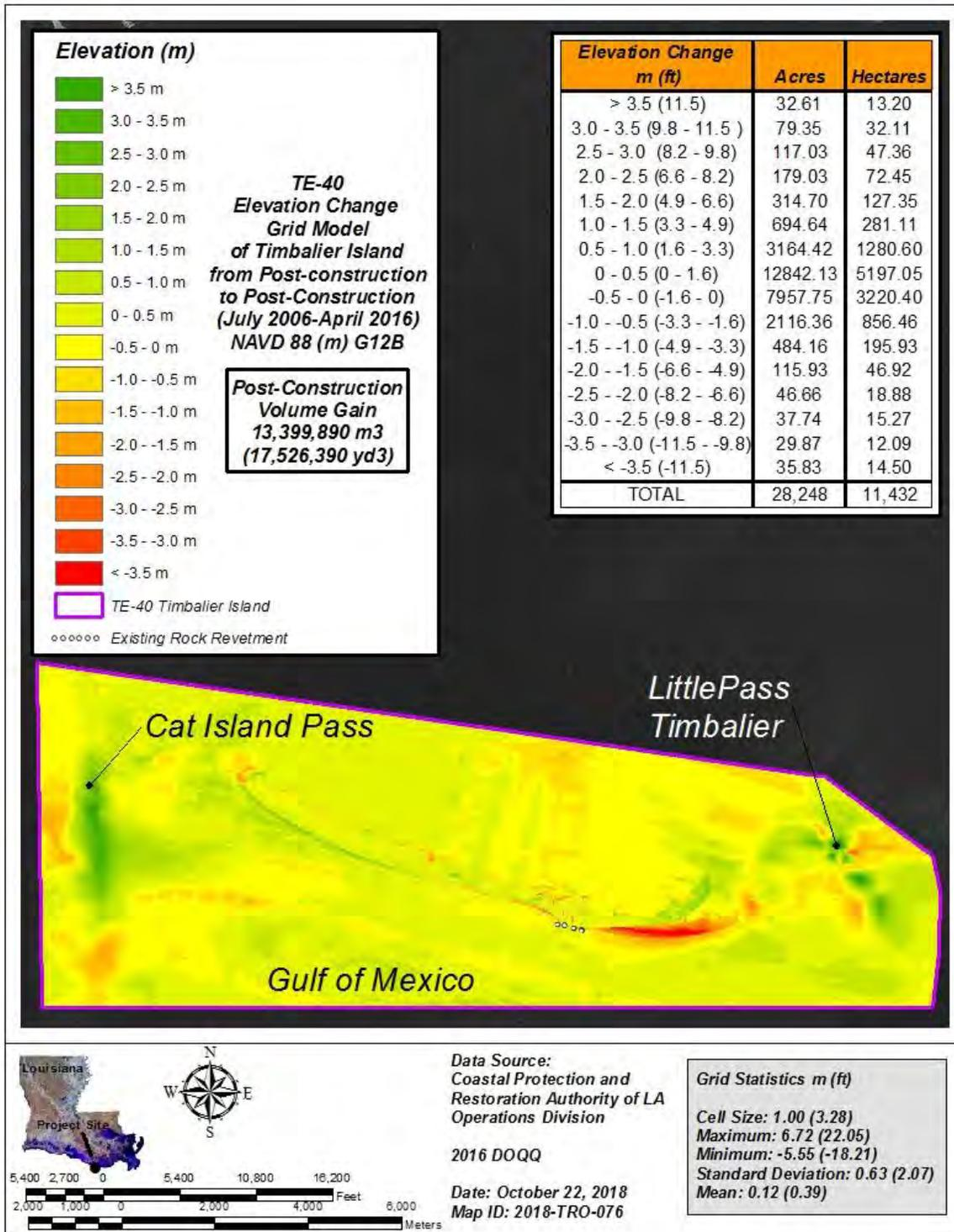
Figure 4-4. Elevation and volume change grid model for the Timbalier Island system from Jul 2006 to Apr 2016. This timeline represents the post-construction 1 to the post-construction 2 interval for the Timbalier Island Dune and Marsh Restoration (TE-40) project.
