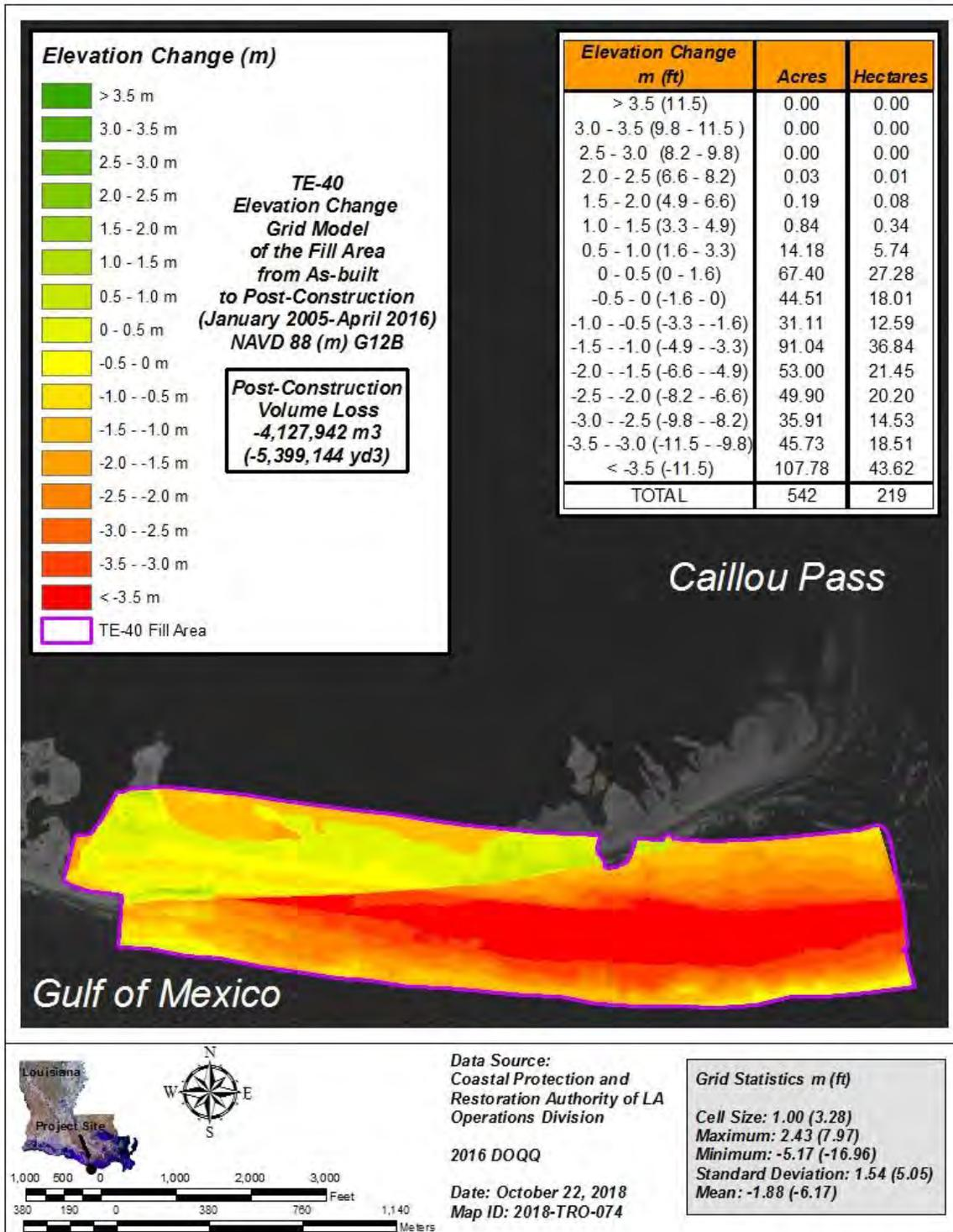
Figure 4-3. Elevation and volume change grid model for the TE-40 fill area from as-built (Jan 2005) to post-construction 2 (Apr 2016) at the Timbalier Island Dune and Marsh Restoration (TE-40) project.
