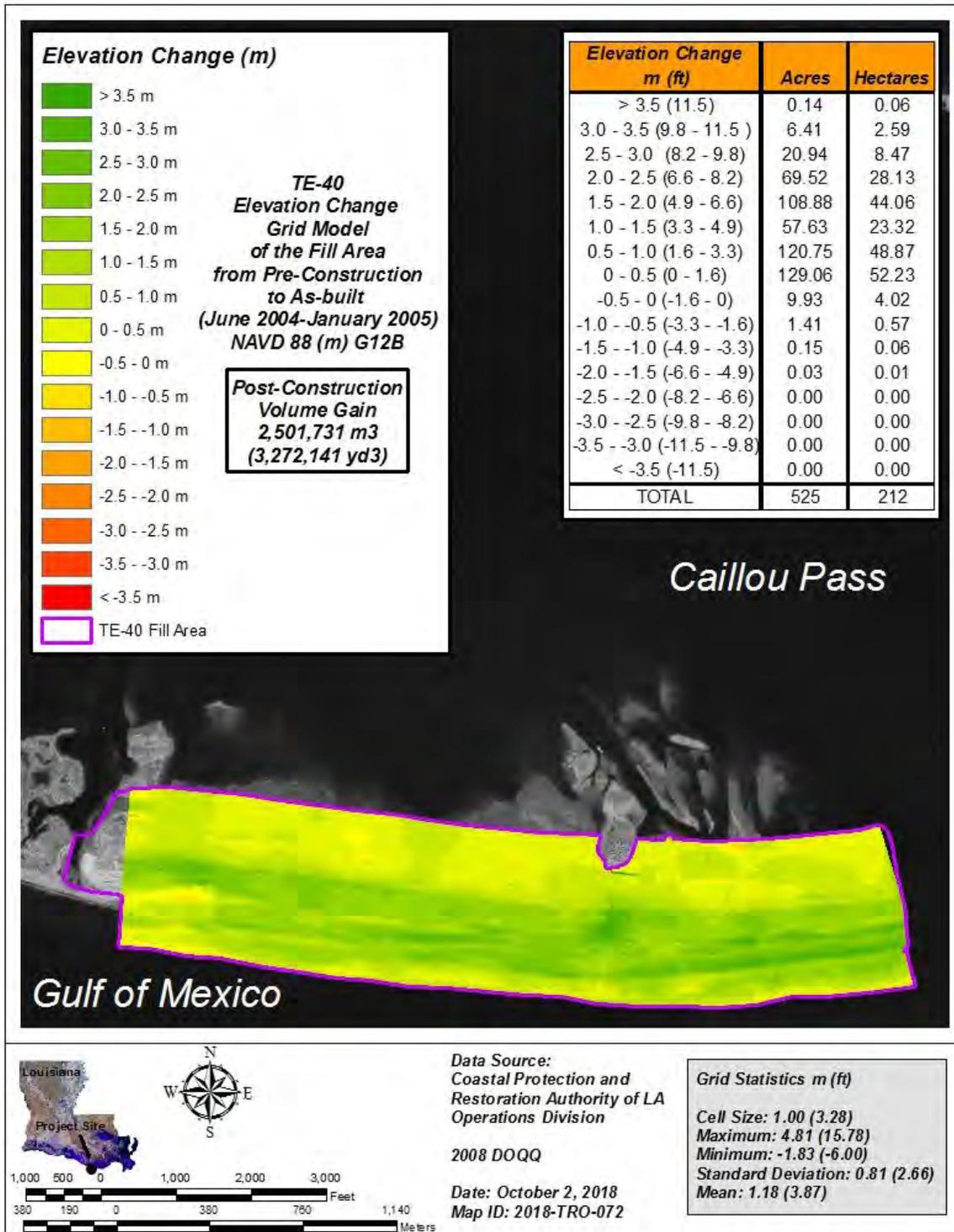
Figure 4-1. Elevation and volume change grid model for the TE-40 fill area from pre-construction (Jun 2004) to as-built (Jan 2005) at the Timbalier Island Dune and Marsh Restoration (TE-40) project.
