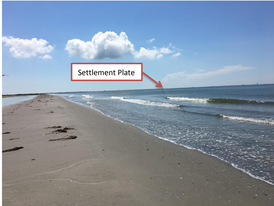
Photo 11: View of settlement plate, which used to be in the center of the dune.
