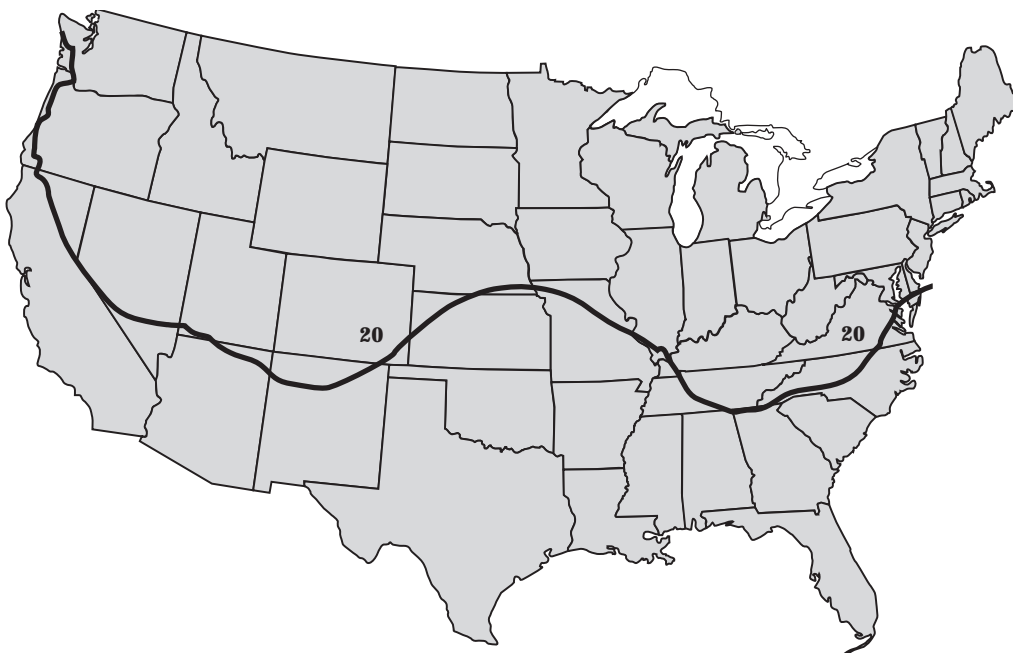
Figure 523–1 Number 20 freeze-thaw severity index isoline (map approximates the map in ASTM D 5312)
