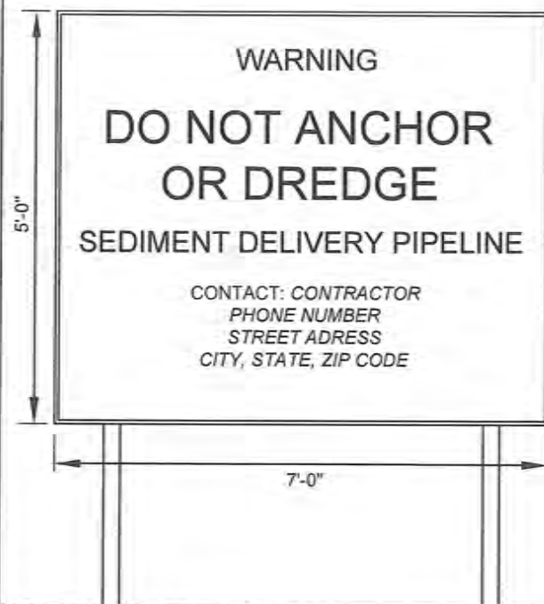
SEDIMENT PIPELINE CHANNEL CROSSING MARKER DETAIL (NOT TO SCALE)
