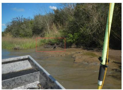
**Figure 2:** Photograph taken during the magnetometer survey depicting a large pile of metal debris outlined in red on bank. This pile of debris would introduce a significant anomaly in the magnetometer data. It is thought to be the source of Anomaly No. 139.
