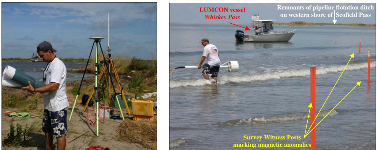
Figure 1. “Pelican Base” survey point and RTK GPS base station located on Scofield Island (left). Terrestrial based magnetometer survey and magnetic anomalies (right).
