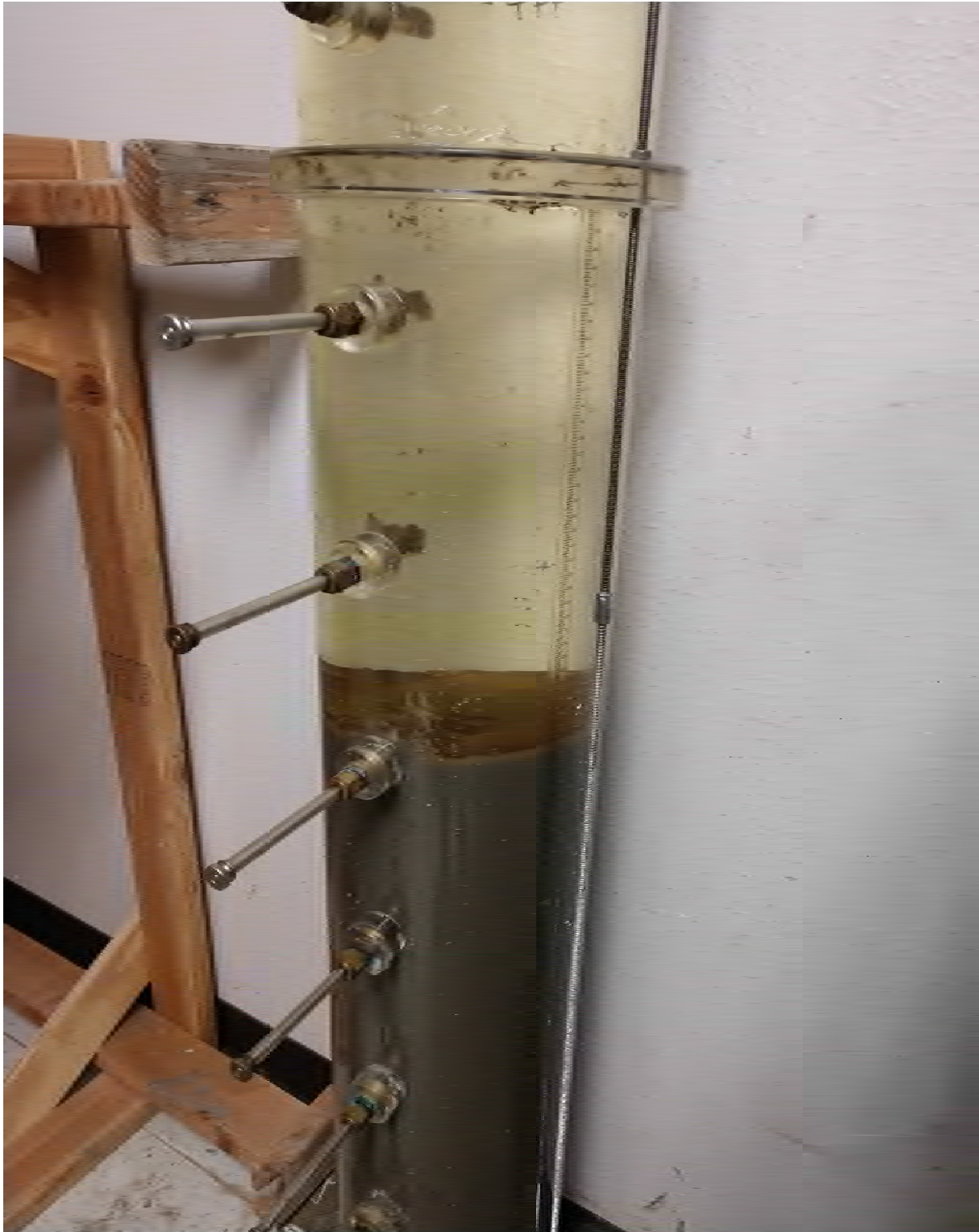
Settling Colum Test
