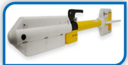
A Geometrics 882 Cesium Vapor Marine Magnetometer was used to conduct the magnetometer portion of the borrow area survey. The tow fish was pulled from the stern of the vessel at a distance (layback) of 81' along the provided transect lines to prevent any interference from the vessel. RTK GPS data from the Leica GS14 was input into Hypack data collection software to correlate the vessel position with the towfish.
