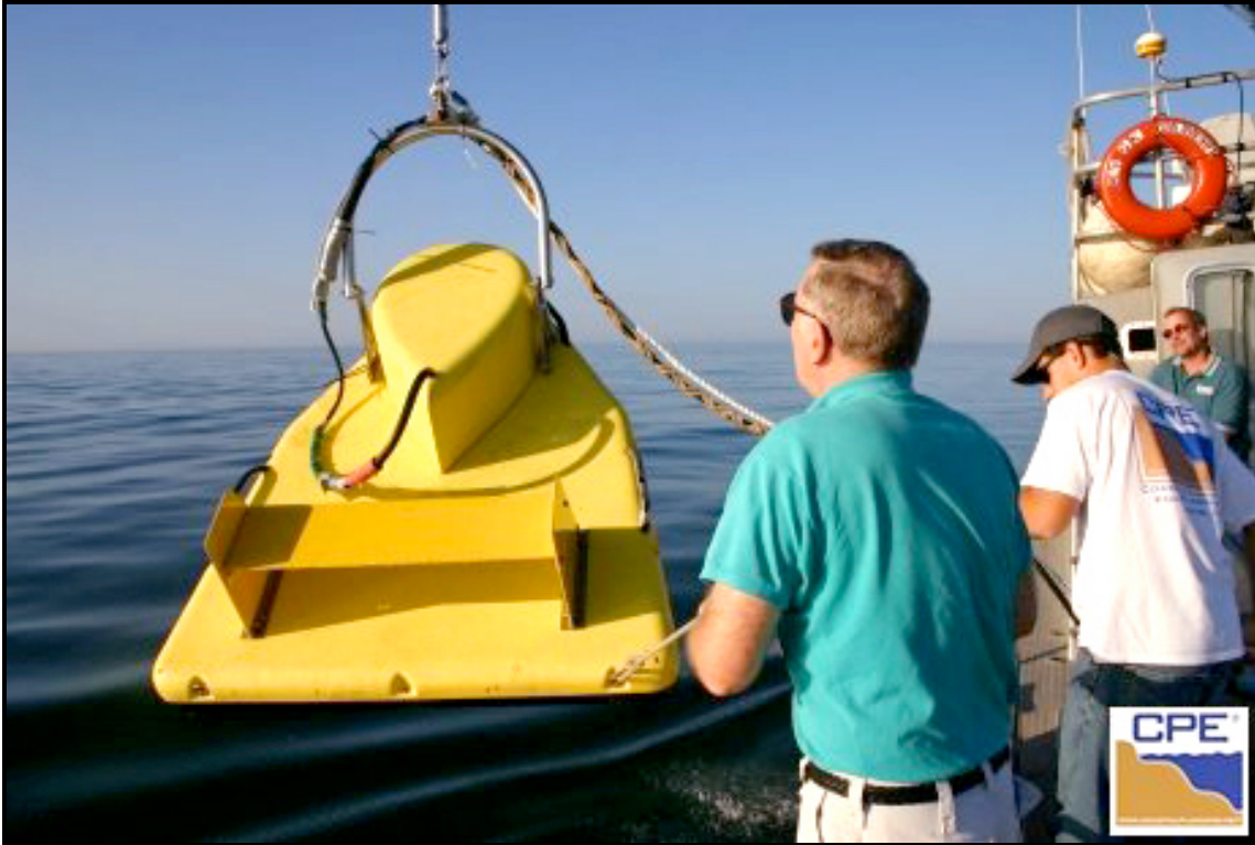
Figure 10. EdgeTech 512i Sub-bottom Profiler Towfish.
