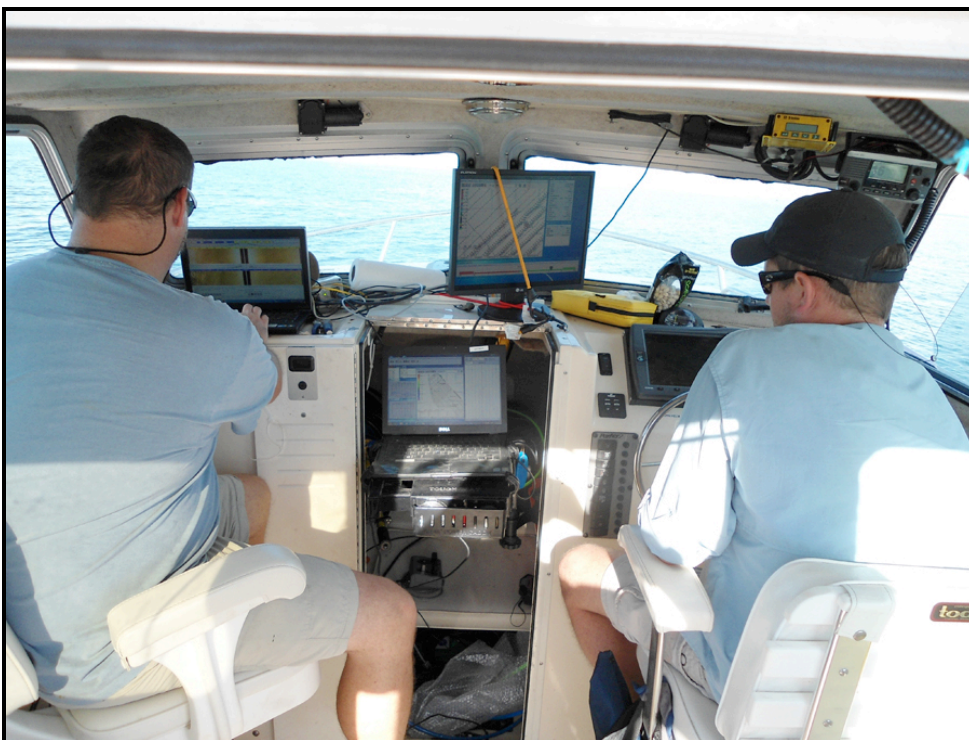
Figure 6. Navigation and Sonar Computers on Survey Vessel Bridge.
