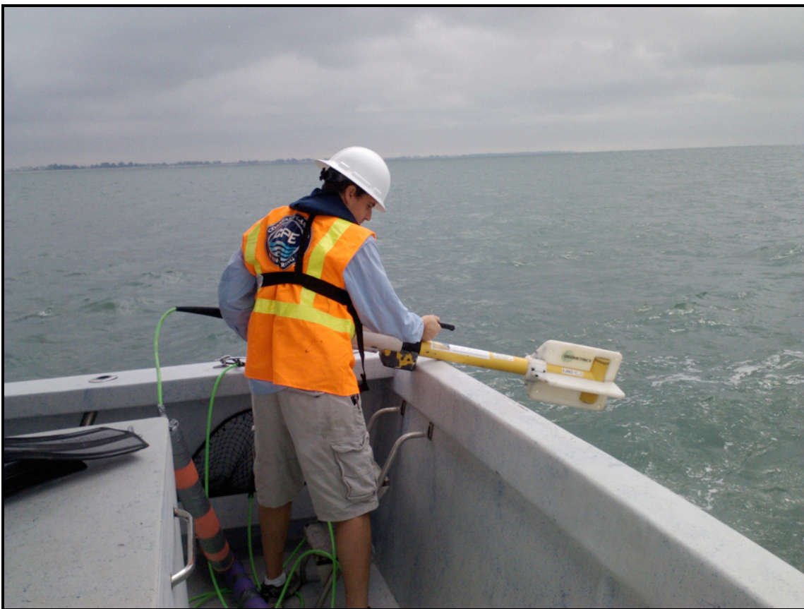
Figure 8. Geometrics 882 Cesium Vapor Magnetometer.
