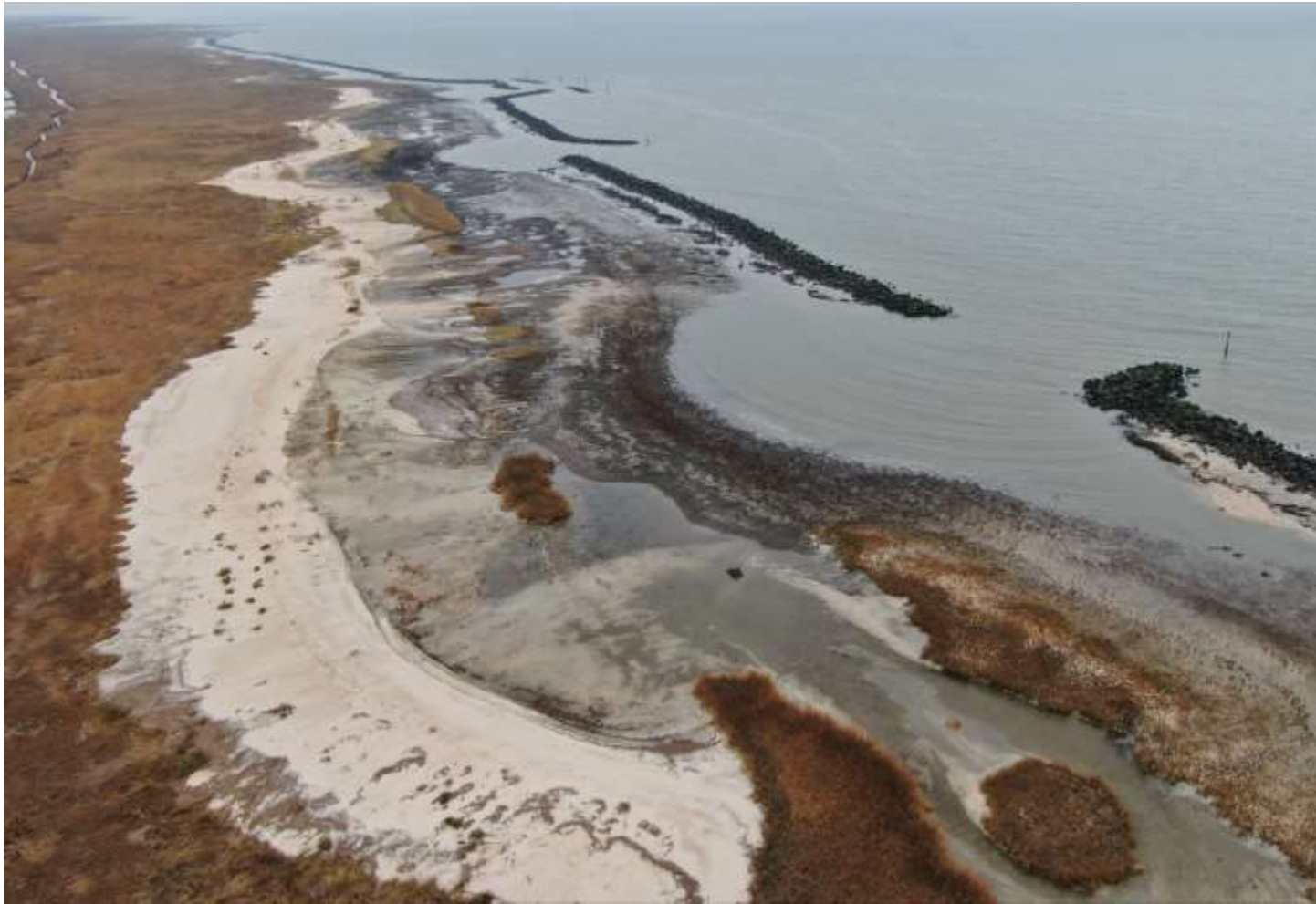
Photo A2: Taken January 29, 2025 facing southeast towards wider fish gaps west of LA-0008. The enhanced erosion is apparent by the concave shoreline and fragmented, degrading vegetation.
