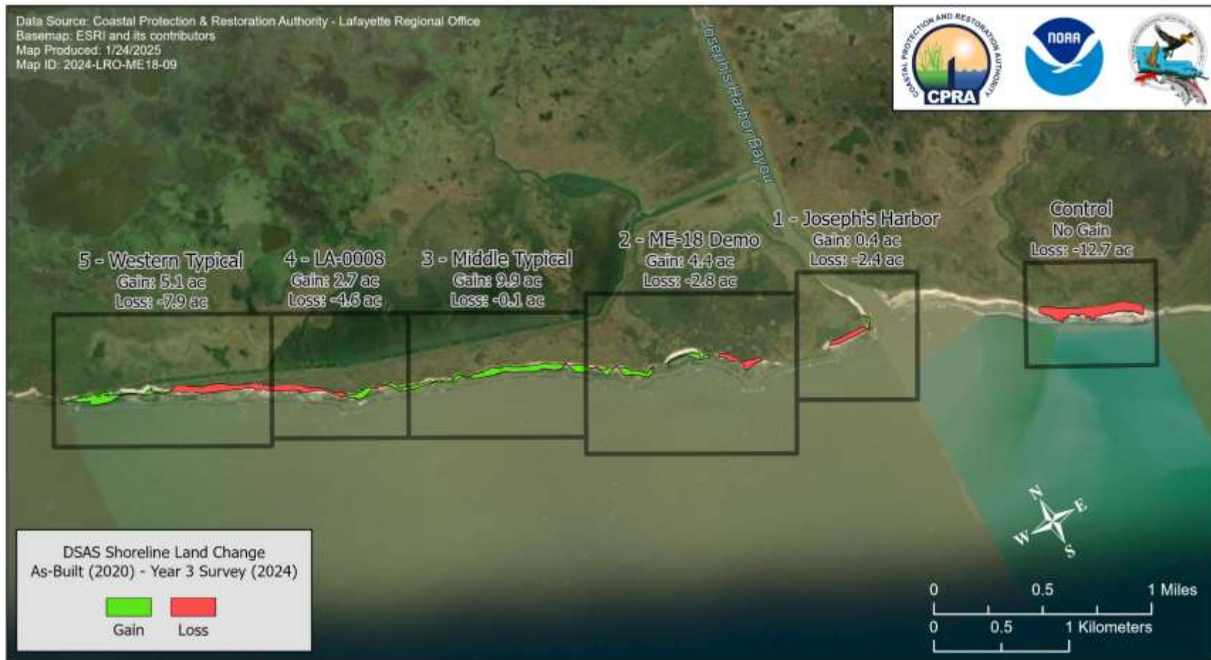
Figure 6. Shoreline land change acreages calculated from DSAS analysis of As-Built (May 2020) and Year 3 (April 2024) survey data.
