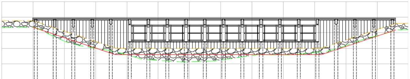
**Figure 17: Variable Crest Weir - Typical Cross Section**
