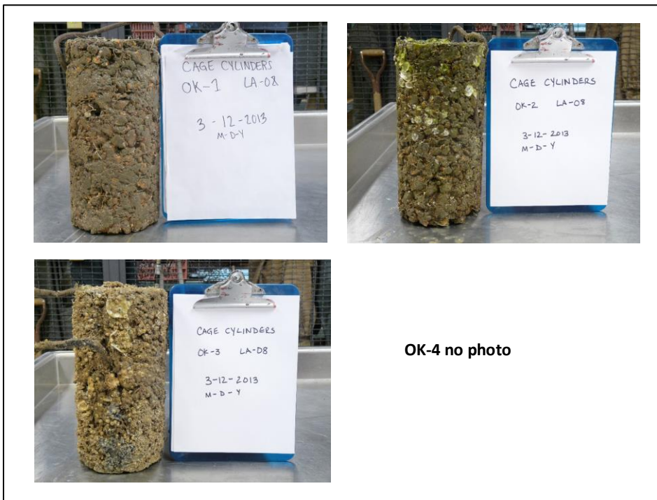
Figure A-9. Experimental OysterKrete Cylinders in Cages Deployed on April 19, 2012 and Retrieved on March 12, 2013.
