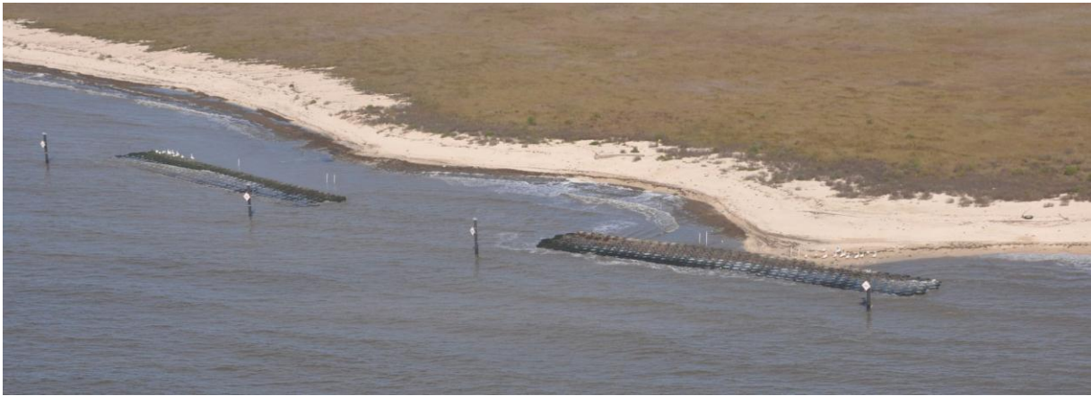
Picture 1. Oblique photograph taken during low water (~0 ft NAVD88) by Louisiana Department of Wildlife and Fisheries about a year after construction of the Oysterbreaks at the Bio-engineered Oyster Reef Demonstration project (LA-08). Note the elevation difference between Oysterbreak - West composed of OysterKete ® (lower) and Oysterbreak - East composed of standard weight concrete (taller) based on water inundation. Also, note the tombolo behind Oysterbreak - East that formed during construction.
