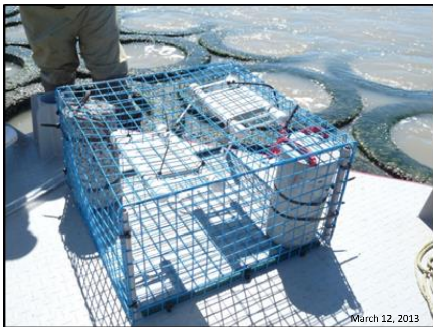
Figure A-4. Photo of Experimental Cage with two Quarry Tiles and two Experimental Cylinders, one OysterKrete (OK) and the other Standard-Weight Concrete (SW).
