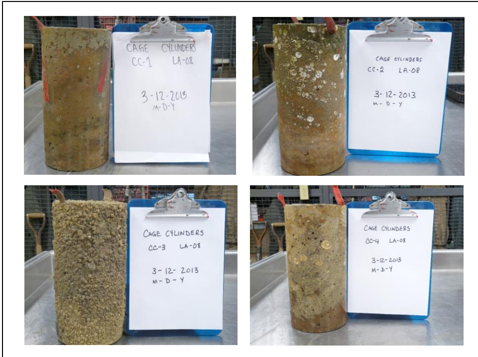
Figure A-8. Experimental Standard-Weight Concrete Cylinders in Cages Deployed on April 19, 2012 and Retrieved on March 12, 2013.
