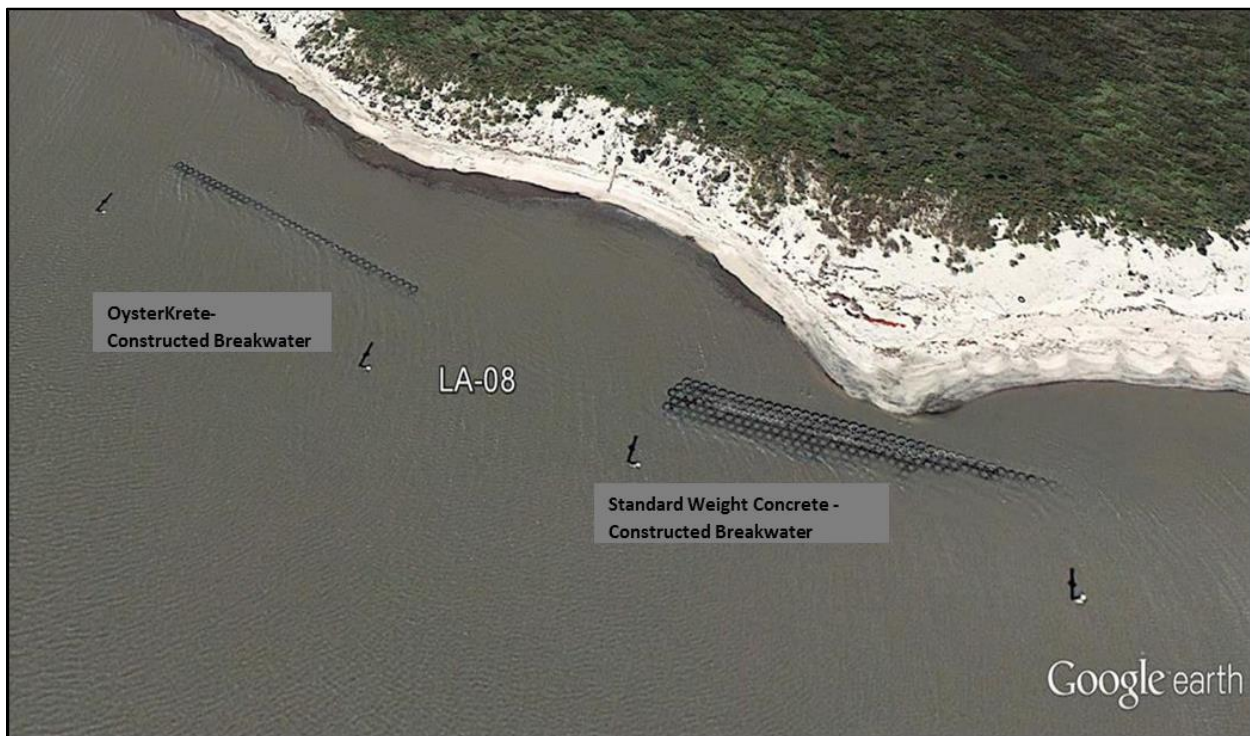
Figure 2. Aerial View of Completed Project LA-08 Oysterbreaks at near-High Tide along the Gulf of Mexico Shoreline; OysterKrete (OK) is to the West and Standard-Weight Concrete (SW) is to the East.
