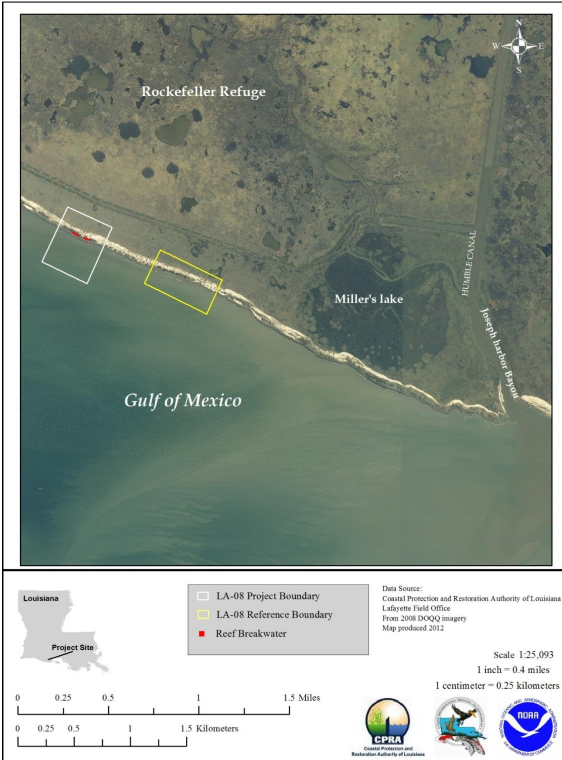
Figure 1. The Bioengineered Oyster Reef Demonstration Project (LA-08) consists of two reef segments on the Gulf of Mexico coast of Rockefeller Wildlife Refuge. The Reef Breakwaters (Oysterbreak™ segments) are each 215 ft long; the OysterKrete segment is to the west, and the standard weight concrete segment is to the east.
