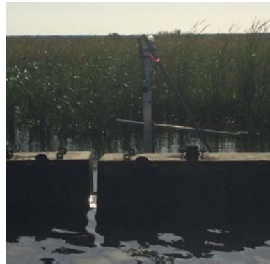
Site 4. Buoyancy compensated erosion control modular system.
