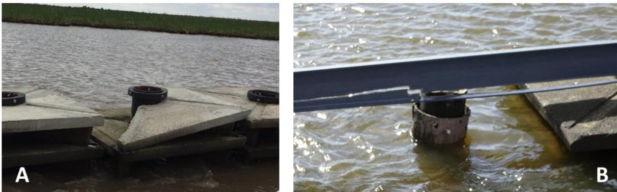
Figure 17. (A) Breakage of upper plates was caused by flexibility of the fiberglass pile. (B) The C-channel used for bracing the piles cracked and split by the end of the one and one-half year monitoring period.
