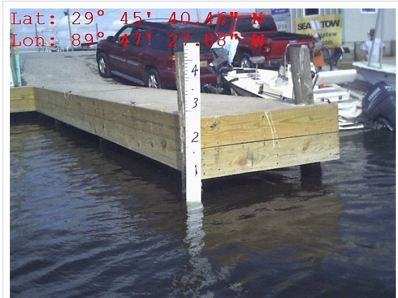
Staff Gauge Installed at Boat Launch in Bayou Terre Aux Boeufs
