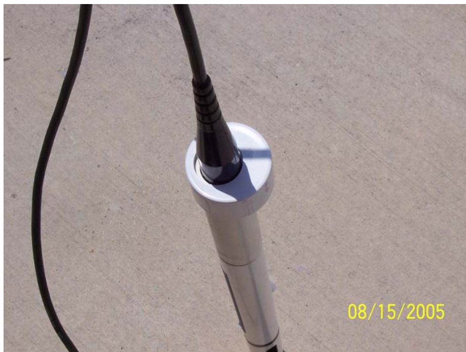
Figure 1: A 2" Schedule 40 PVC cap threaded through the cable and sitting on top of a Hydrolab MS5 continuous recorder.
