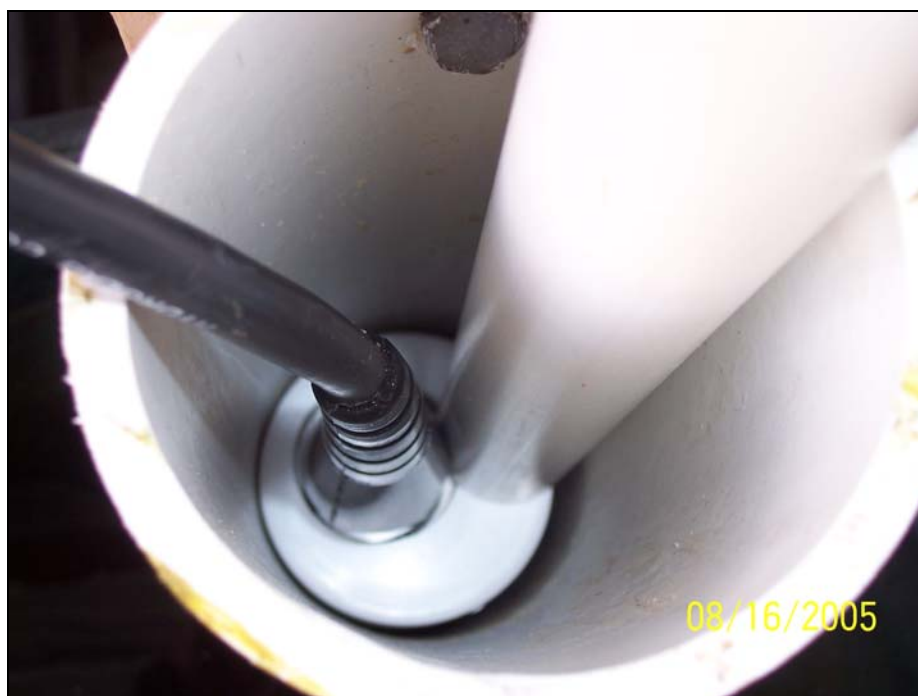
Figure 2: Hydrolab MS5 resting in a 3" Schedule 40 PVC well with the 2" PVC cap and a 1" Schedule 40 PVC pipe.
