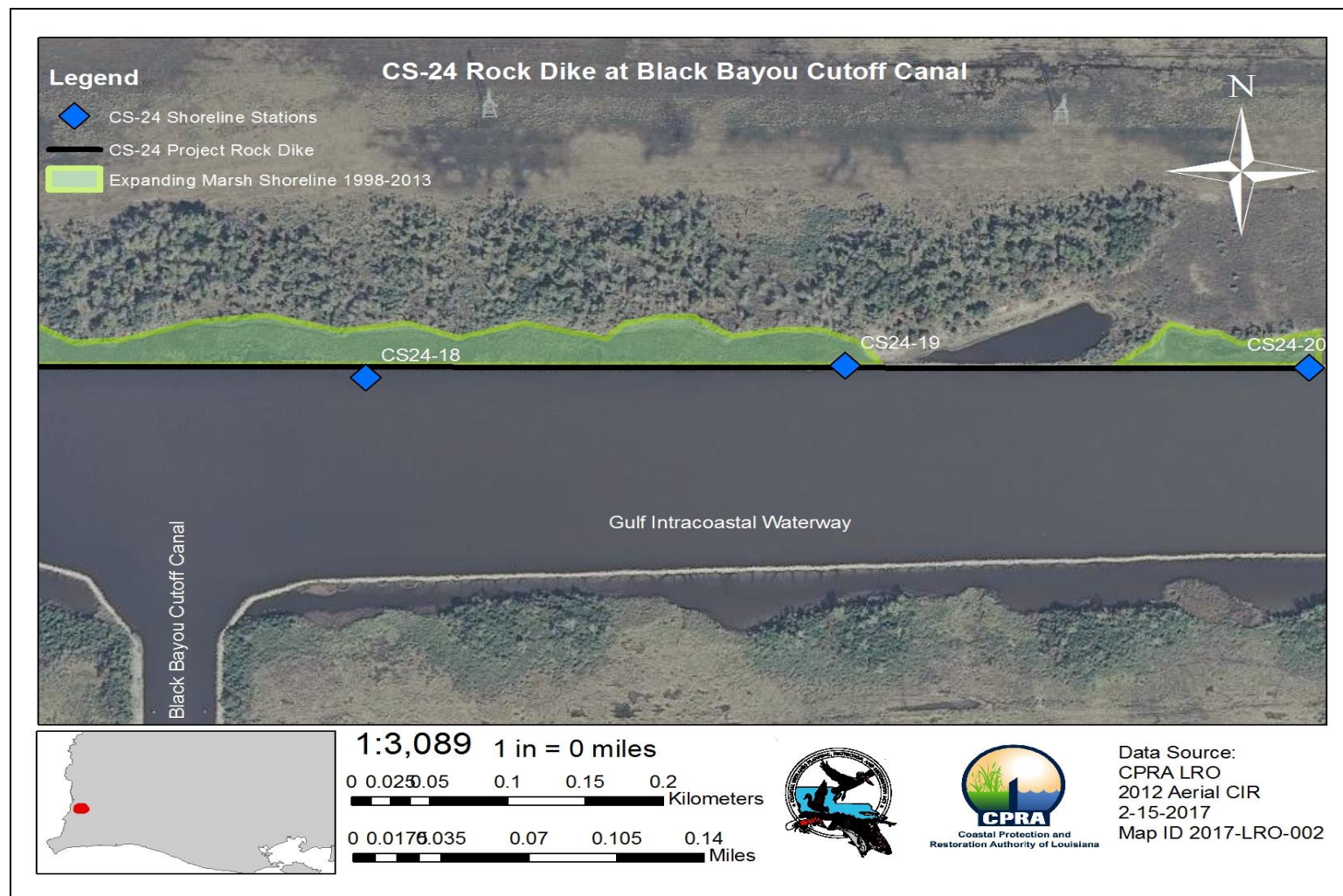
Figure 6. A typical shoreline reach at Perry Ridge (CS-24) illustrating the rock dike, shoreline stations, and expanding marsh shoreline at the confluence of Black Bayou Cutoff Canal and the GIWW in the central region of the project.
