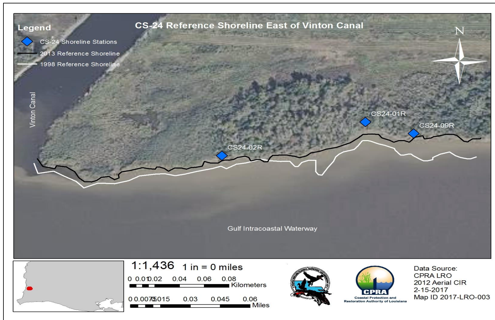
Figure 7. The reference shoreline at Perry Ridge (CS-24) containing shoreline stations and historic shoreline positions at the confluence of the Vinton Canal and the GIWW just east of the project area.
