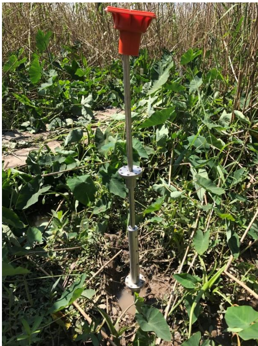
Figure 4.4. Photograph of CRMS rod extension with new collar at Mississippi River Delta site CRMS0156 in 2016
