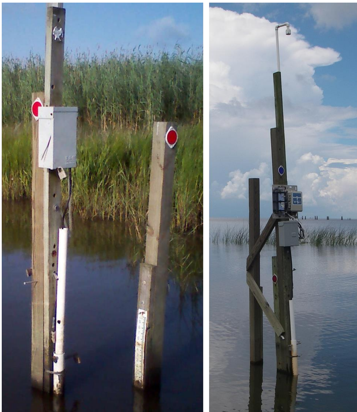
Figure 3.1b. Photographs of typical hydrologic recorder stations. The original version is to the left and the newer version is to the right (see Fig. 3.5b for snorkel description).
