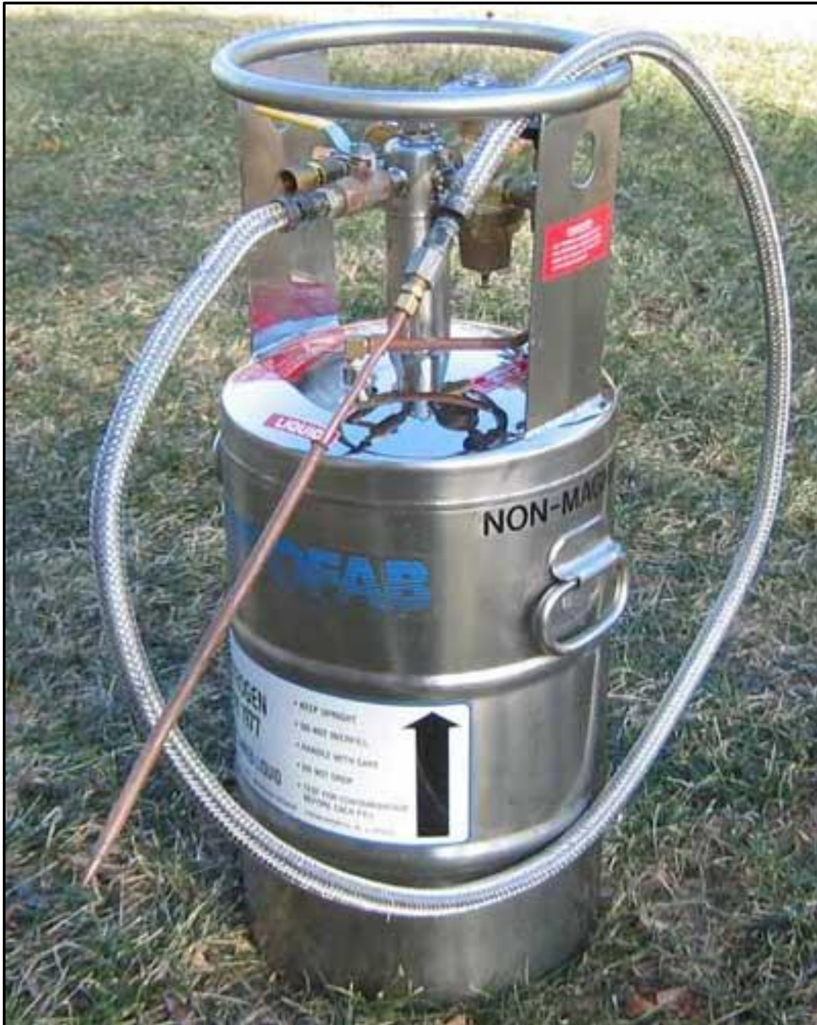
Figure 5.4b. Photograph of cryogenic coring equipment including the liquid nitrogen cylinder (cryo-cyl), flexible hose, and copper bullet (cryo-probe).
