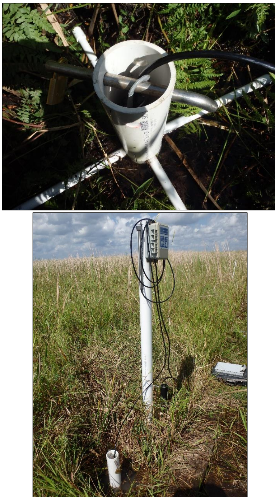
Figure 3.4b. Photographs of a typical floating marsh mat recorder deployed in the field
