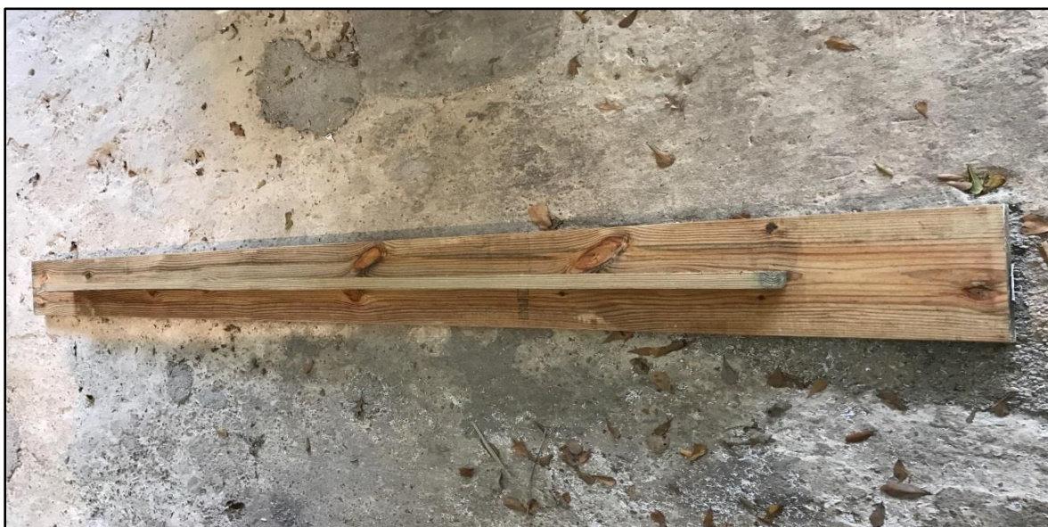
Figure 2.6. Photograph of a 2"x12"x12' boardwalk plank with a 2"x4"x8' strong-back bracing underneath.
