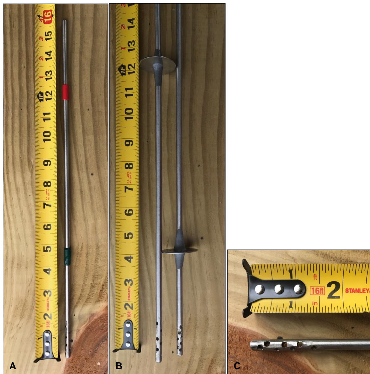
Figure 3.20. Stainless steel sipper tube alternatives for soil porewater collection. (A) Green and red tape mark 10 cm and 30 cm soil depths, respectively, for non-flooded conditions. (B) Metal washers fixed with a marine grade, metal adhesive (epoxy or weld compound) stop the tube at 10 cm and 30 cm soil depths in flooded conditions. (C) Larger diameter holes (1/8 in. diameter) are drilled to reduce clogging at the extraction depth.
