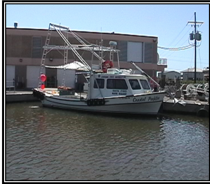
Figure 2. The R/V Coastal Profiler, a custom built vessel for shallow water geophysical survey work and coring.
