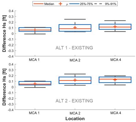
Figure 14. Differences in Hs at the lakeside berm of MCA 1, 2, and 4 for a 1-yr event.
