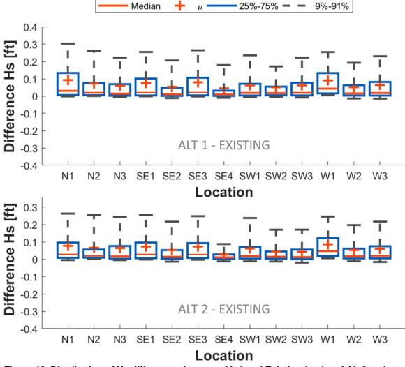
Figure 10. Distribution of Hs differences between Alt 1 and Existing (top) and Alt 2 and Existing (bottom) conditions. The average difference ( $\mu$ ) in Hs between 04/11/2015 – 04/11/2016 is approximately 0.07 ft (0.8 inches) for an average Existing Hs of 0.4-0.5 ft.
