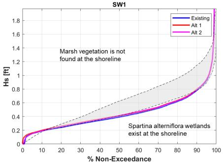
Figure 18. Representative year wave conditions at the project shoreline (SW-1) plotted against the R&D curve (dashed line).
