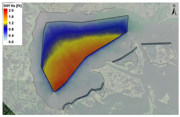
Figure 13. Increase in wave height for Alternative 2 during a 20-yr event at 345°.
