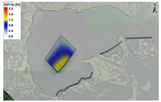
Figure 12. Increase in wave height for Alternative 1 during a 20-yr event.
