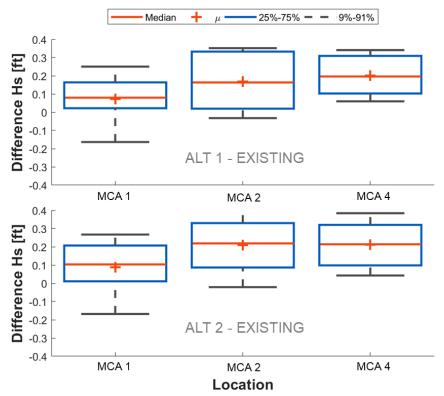
Figure 15. Differences in Hs at the lakeside berm of MCA 1, 2, and 4 for a 20-yr event.
