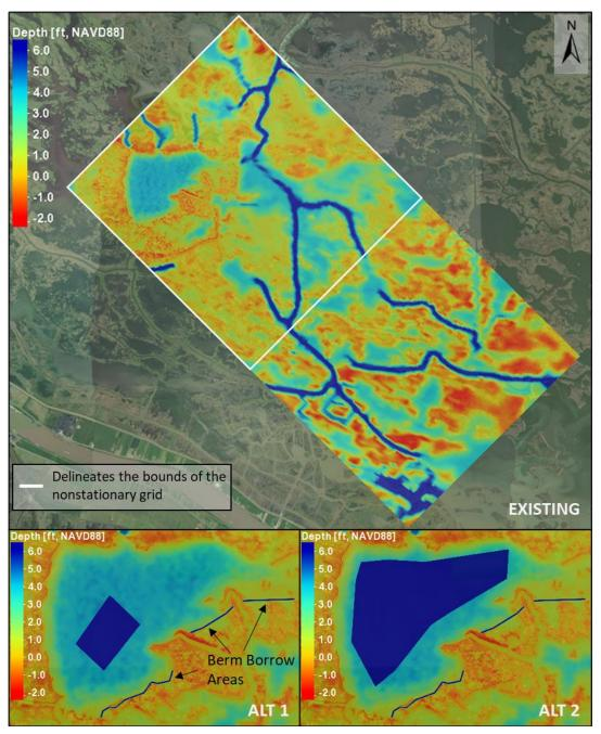
Figure 8. Bathymetric grids (top). Details are shown for proposed alternatives Alt 1 and 2.
