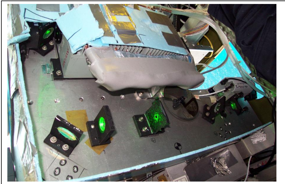
Figure 3. Photograph of EAARL's laser operating in aircraft (NASA, 2003).
