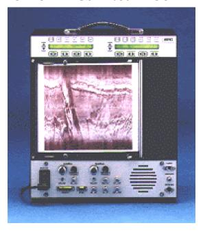
The EPC Model GSP-1086 is an all-purpose, continuous image printer. Photographic quality images are printed using a 2048 pixel thermal print head with dot density of eight dots/millimeter. Pixel depth is selectable up to eight bits.
