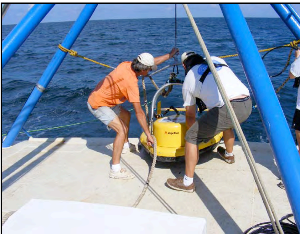
Figure 8. Launching the EdgeTech 512i sub-bottom profiler.
