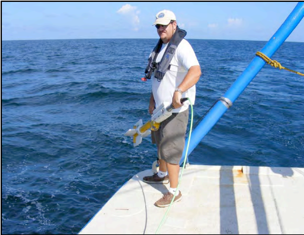
Figure 6. Deploying the EG&G Geometrics G-882 magnetometer.
