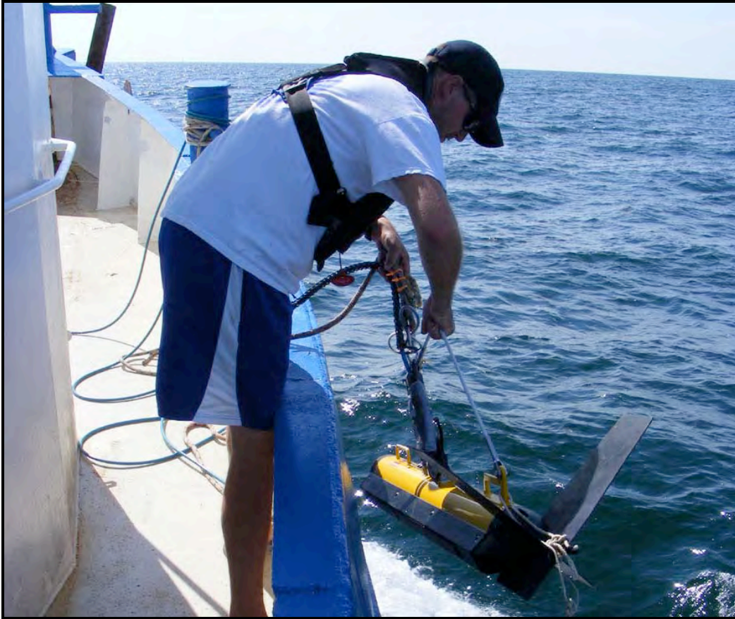
Figure 7. Launching the EdgeTech 4200-HFL sidescan sonar.
