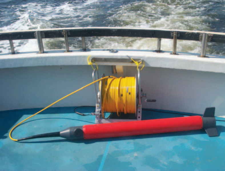
SeaSPY towfish with altimeter and 200m of cable on a metal reel
