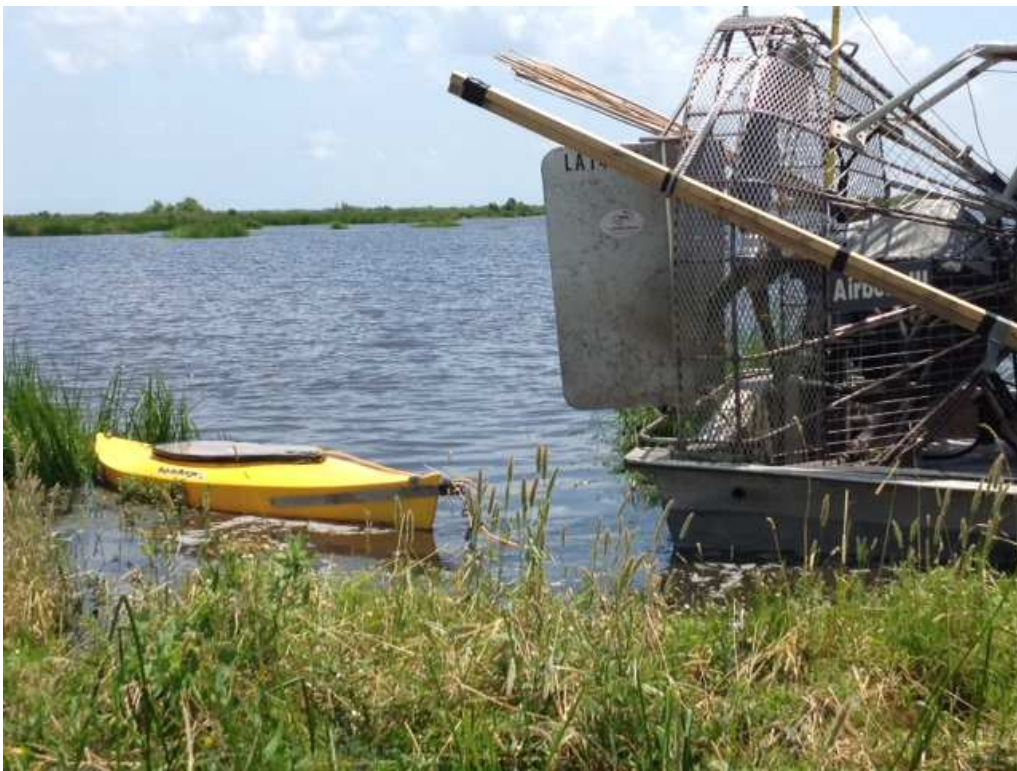
Figure 1. Proton magnetometer sensor mounted inside a kayak being towed behind Airboat.
