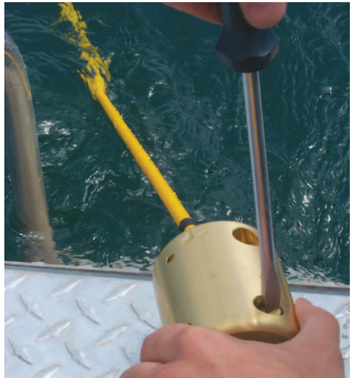
Brass tow cable weight attached to MMC's cable
