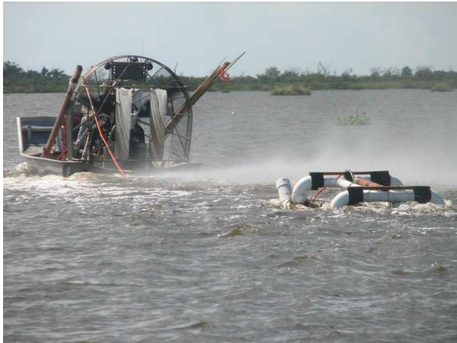
Figure 1. Proton magnetometer sensor and PVC sled being towed behind Airboat.
