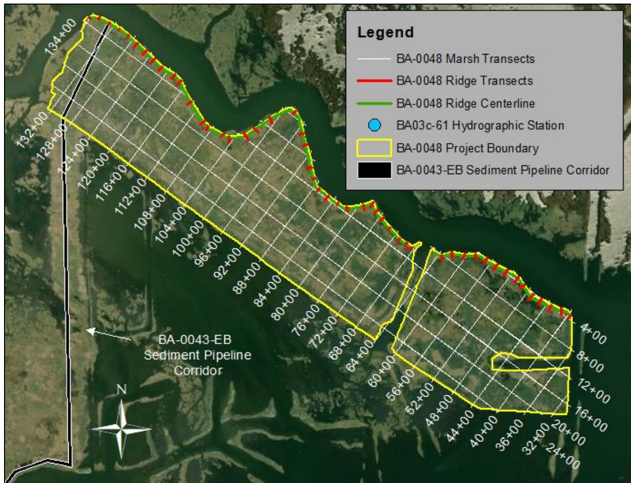
Figure 2. BA-0048 marsh and ridge established elevation survey transects.
