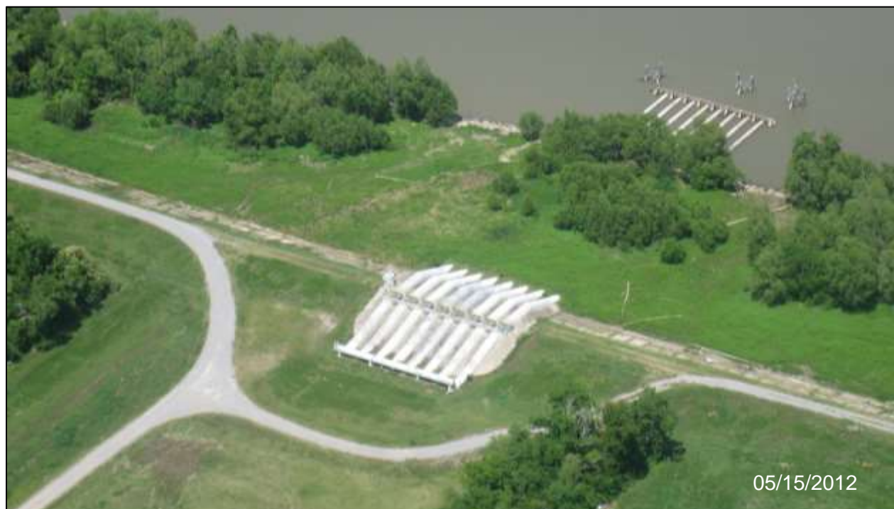
Figure 1. Naomi Siphon Diversion (BA-0003). Visible in the photograph is the location of the eight siphon intakes in the Mississippi River and the section of the siphons that was constructed over the top of the levee. The siphons discharge into an outfall pond just outside of the frame of the photograph.
