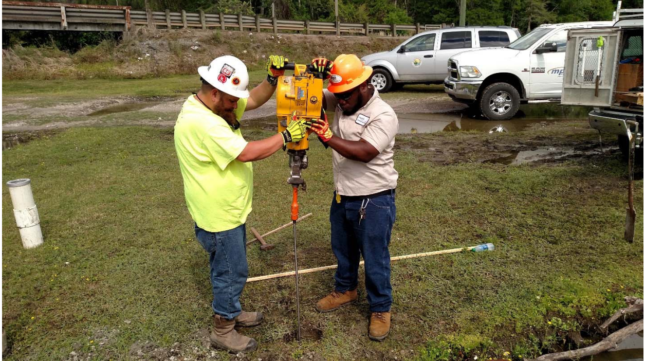
Photograph 21 – MPH crew using a jackhammer to drive rods to refusal.
