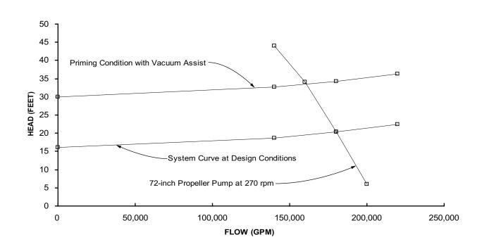
FIGURE G-12 HIGH HEAD, 400-CFS PUMP SELECTION
