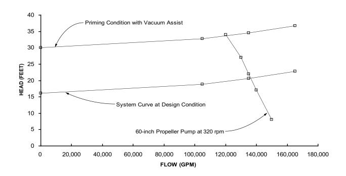
FIGURE G-11 HIGH HEAD, 300-CFS PUMP SELECTIONS
