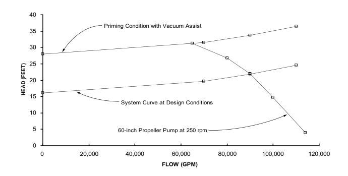
FIGURE G-9 HIGH HEAD, 200-CFS PUMP SELECTION
