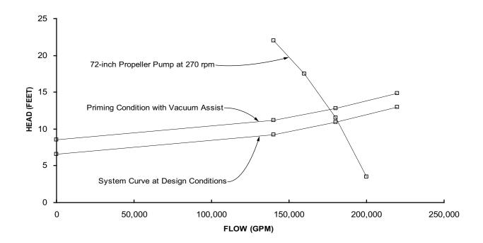
FIGURE G-6 LOW HEAD, 400-CFS PUMP SELECTION
