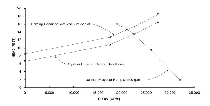
FIGURE G-1 LOW HEAD, 50-CFS PUMP SELECTION
