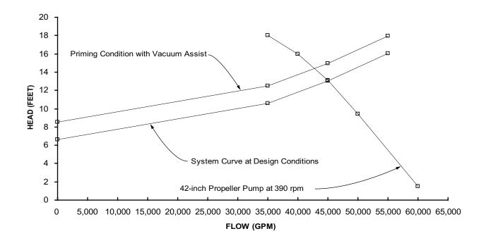
FIGURE G-2 LOW HEAD, 100-CFS PUMP SELECTION
