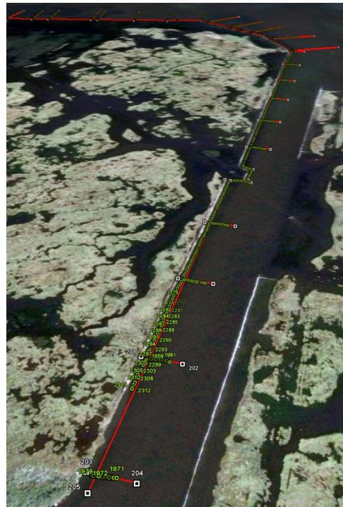
The profile of Structure 14A was taken along the centerline at approximately 25 foot intervals and all points of inflections (PI's) and other low points beginning at Sta. -00+63 and ending at Sta. 16+00. The transects of
