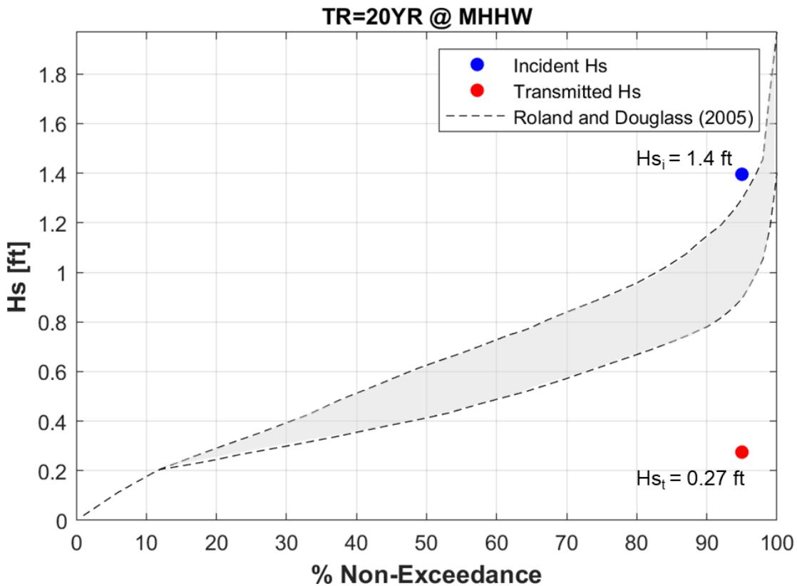
**Figure 20. Wave transmission across 1-row of WAD units for a 20-yr event at MHHW water level. R&D curve included as a reference.**
