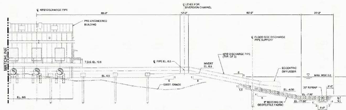
TYPICAL CROSS SECTION OF 48"Ø DISCHARGE PIPE - LOOKING SOUTH
