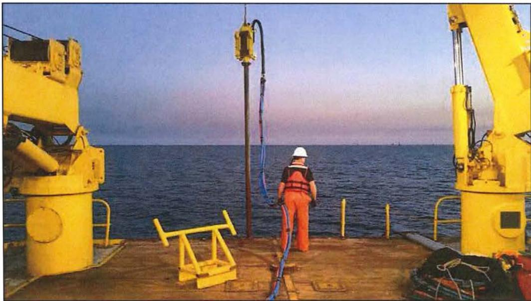
Figure 2. (upper) EBI liftboat utilized during the investigation. (lower) OSI vibratory corer deployed via crane and tended by OSI crew from the deck of the liftboat.
