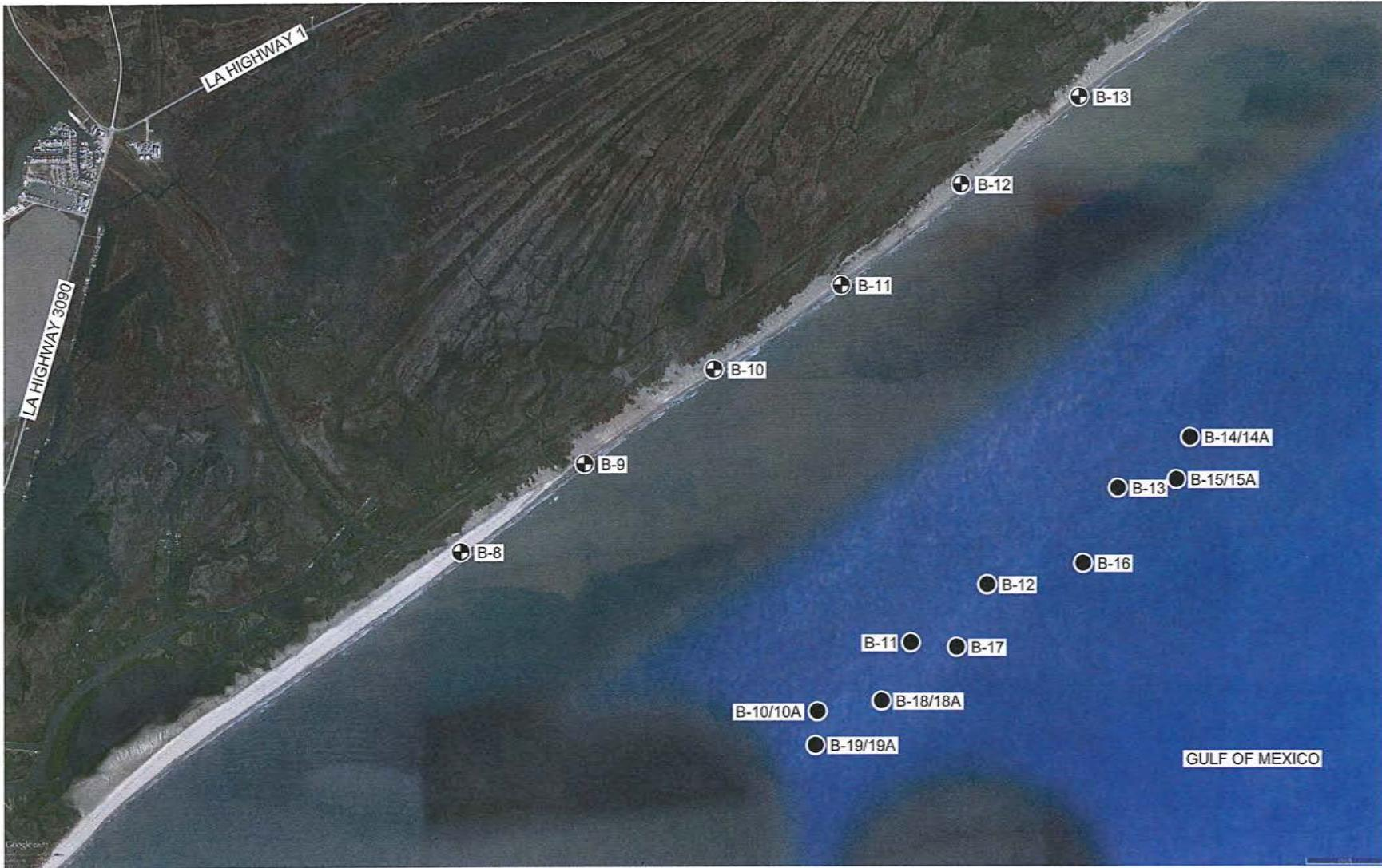
● DENOTES LOCATIONS OF UNDISTURBED SOIL BORINGS PERFORMED BY GEOENGINEERS, INC.
