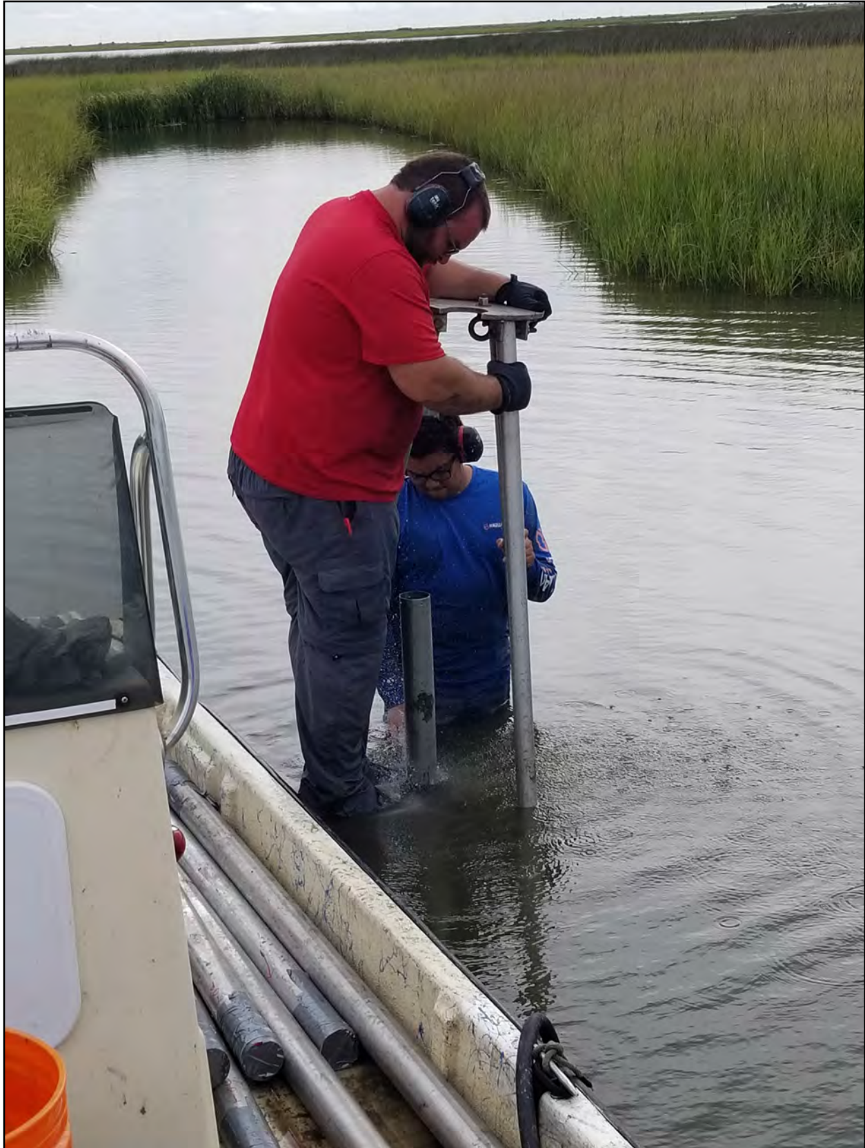
Figure 5.1 Photograph of extraction of vibracore along the dredge pipeline corridors at Long Point Bayou.
