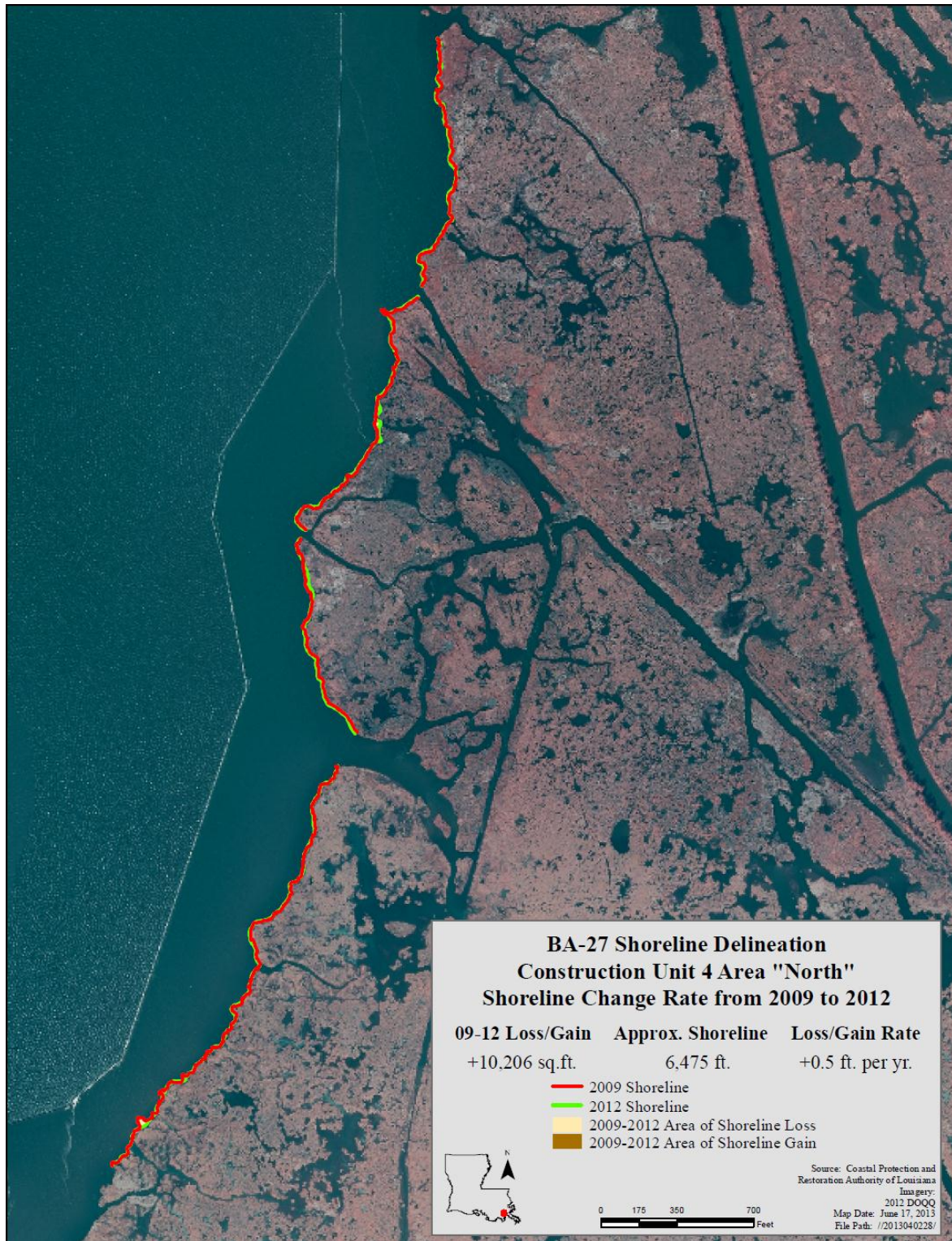
Figure 15. Post-construction shoreline change analysis for the northern section of Construction Unit 4 of the Barataria Basin Landbridge Shoreline Protection Project (BA-27, Phases 1 & 2) from 2009 to 2012.
