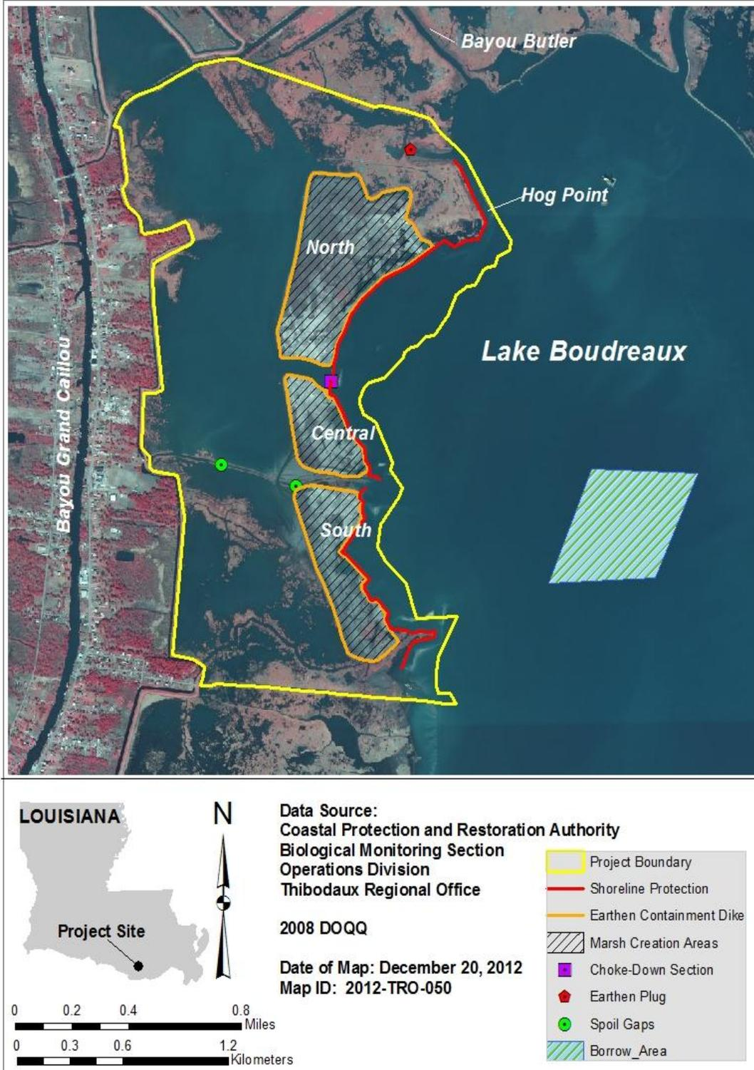
Figure 2. As-built project features located in the West Lake Boudreaux Shoreline Protection and Marsh Creation (TE-46) project area.
