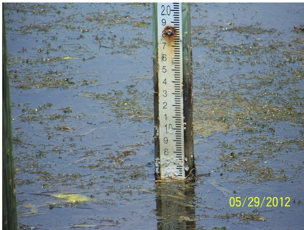
Photo #36: View of water level reading of 0.6' NAVD88 @ 1:20pm from station BA-02-57
