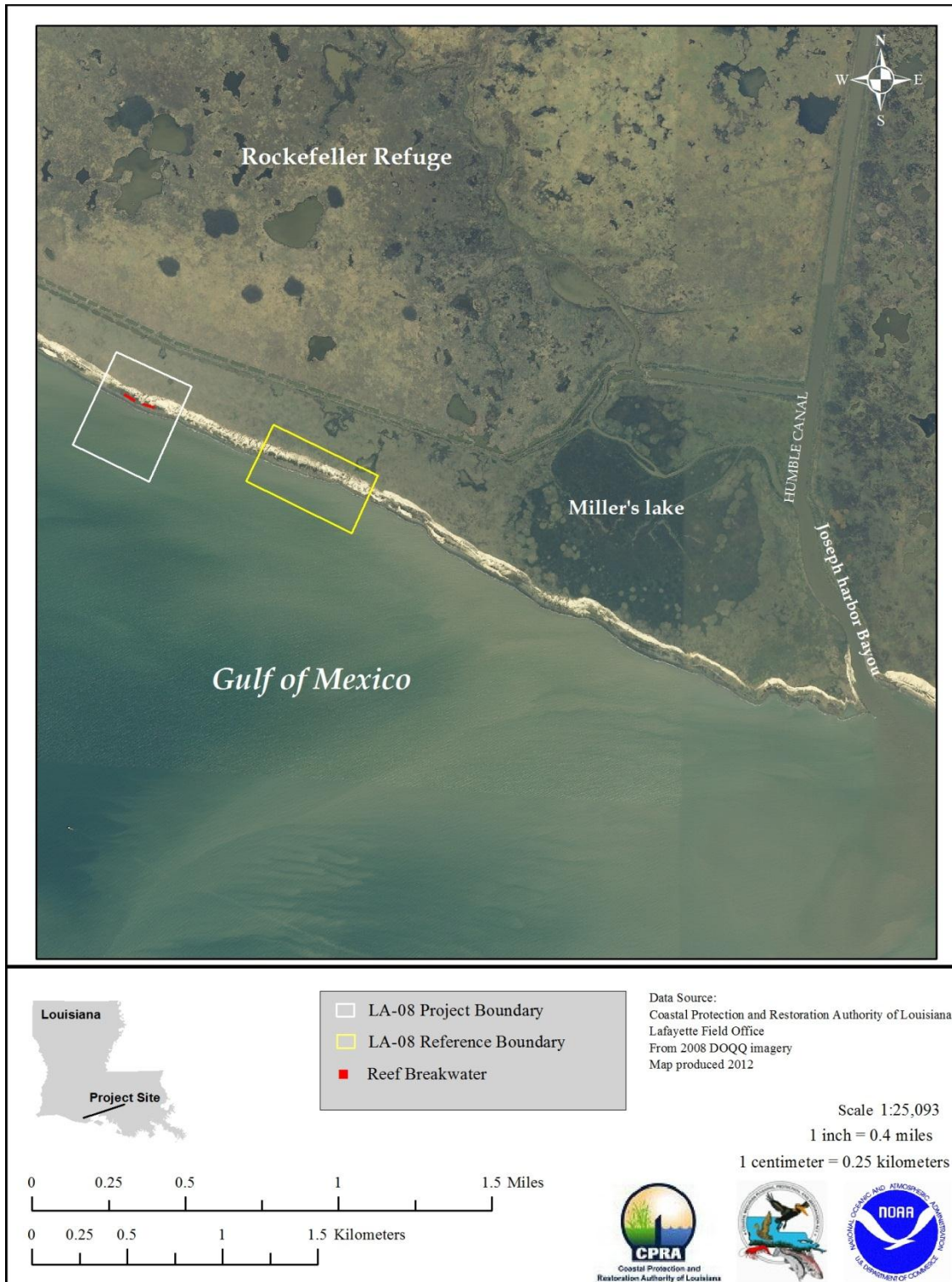
Figure 1. The Bioengineered Oyster Reef Demonstration Project (LA-08) consists of two reef segments on the Gulf of Mexico coast of Rockefeller Wildlife Refuge. The reef segments are each 215 ft long and intended to act as breakwaters to diminish wave energy from eroding the coastline. Note that the reef segments are located on the 2008 shoreline.
