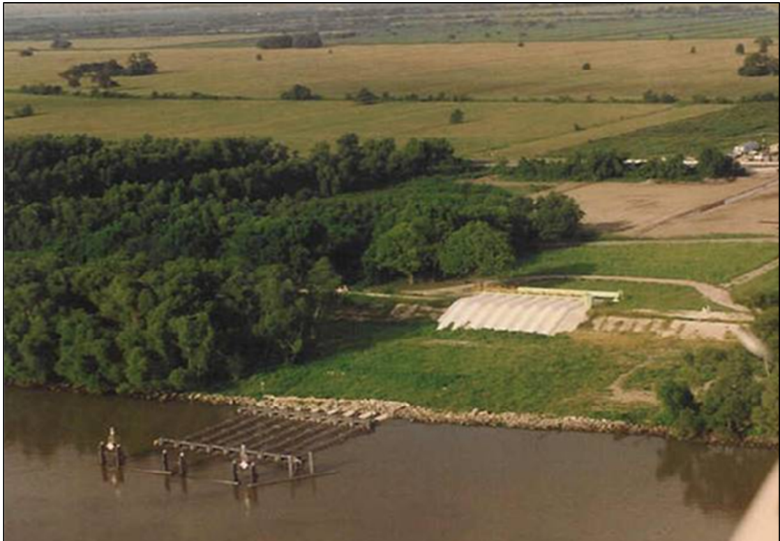
Figure 1. Naomi Siphon Diversion (BA-03). Water is siphoned from the Mississippi River, discharged into a ponding area (not visible in this photograph), and distributed through a single channel into the surrounding marshes.
