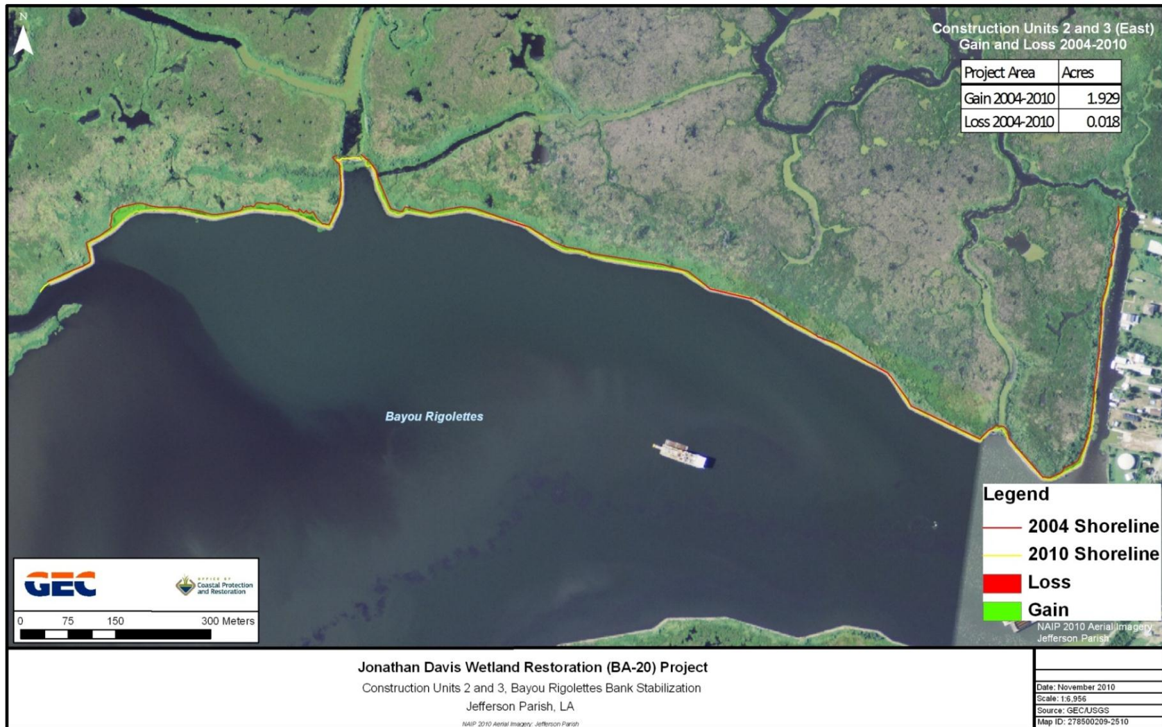
Figure 25. Shoreline change within Construction Unit 2 and the eastern portion of Construction Unit 3 of the Jonathan Davis Wetland Restoration (BA-20) project from 2004 to 2010.
